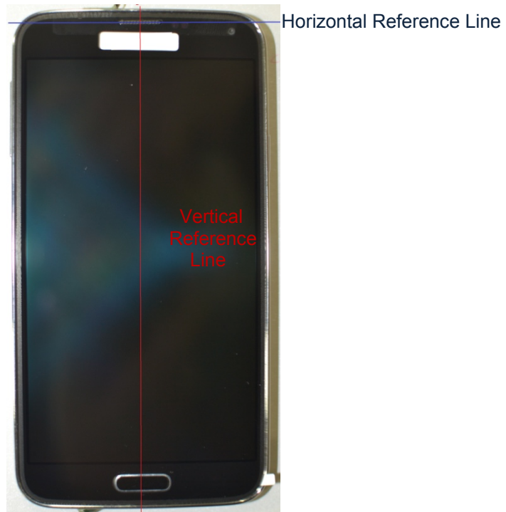
SAR Test Setup Photo 10 – Horizontal and Vertical Reference Lines
