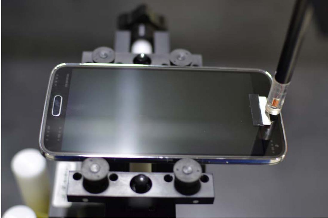
Figure 13-1 Test Setup for Wireless Device
