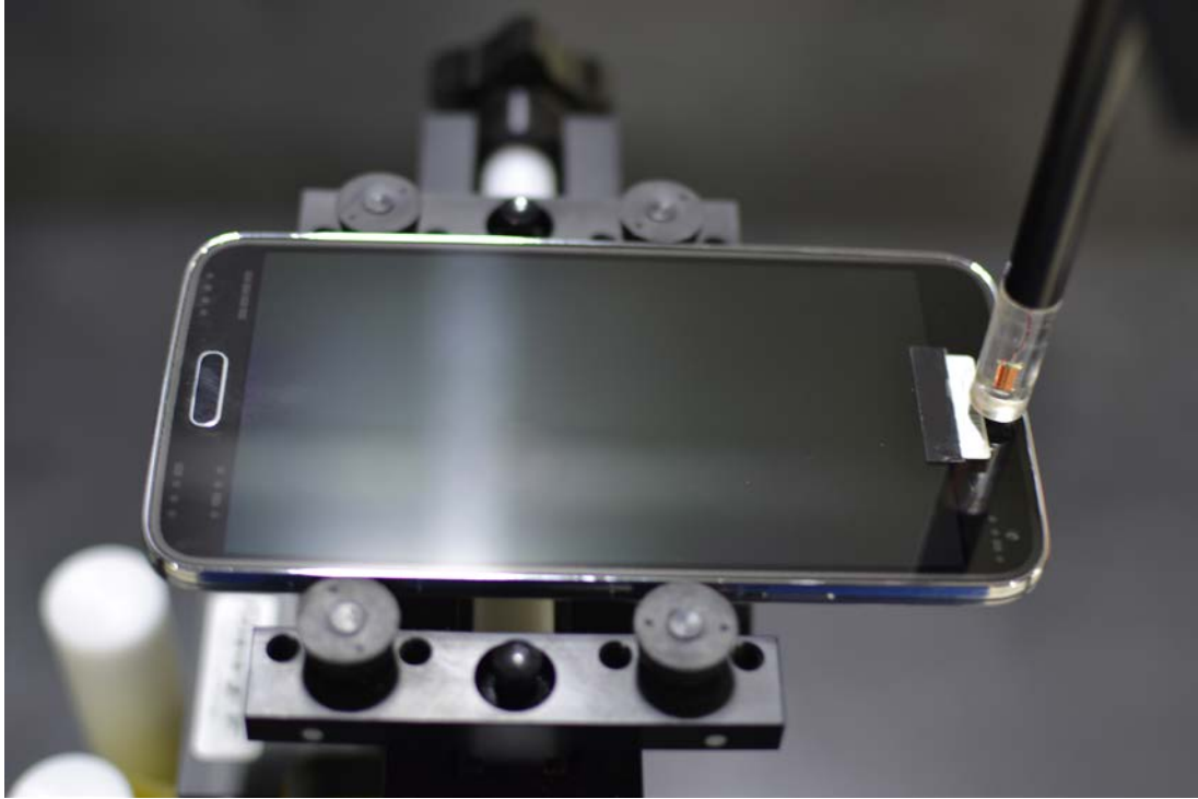
Figure 13-1 Test Setup for Wireless Device
