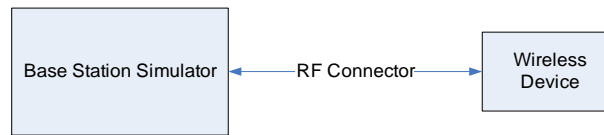
Figure 9-2 Power Measurement Setup
