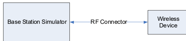
Figure 9-3 Power Measurement Setup
