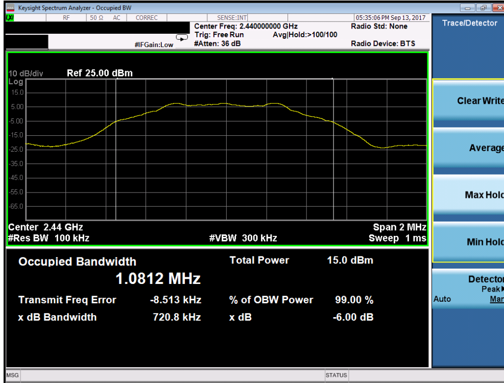
Plot 7-2. 6dB Bandwidth Plot (Bluetooth (LE), 1Mbps – Ch. 19)
