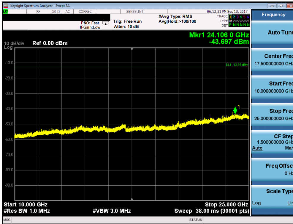
Plot 7-28. Conducted Spurious Plot (Bluetooth (LE), 1Mbps – Ch. 39)
