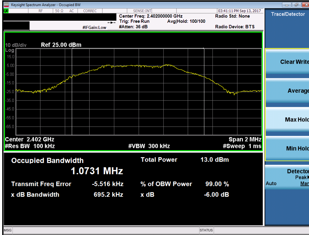
Plot 7-4. 6dB Bandwidth Plot (Bluetooth (LE), 2Mbps – Ch. 0)
