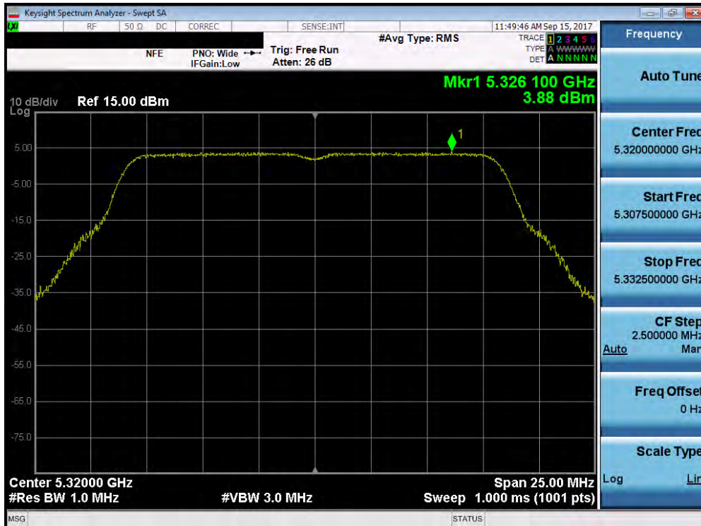
Plot 7-129. Power Spectral Density Plot (802.11a (UNII Band 2A) – Ch. 64)
