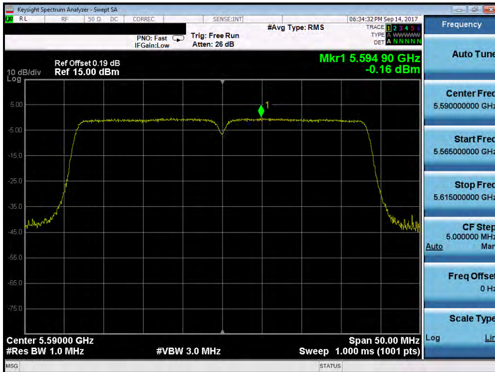
Plot 7-104. Power Spectral Density Plot (40MHz BW 802.11n (UNII Band 2C) – Ch. 118)
