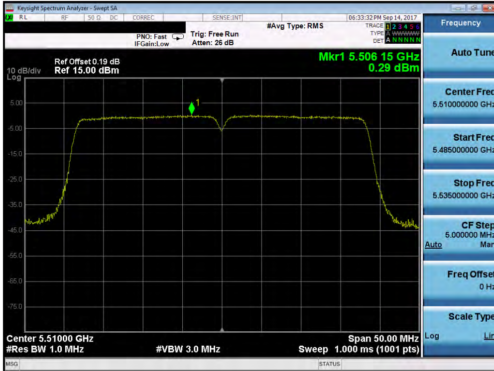
Plot 7-103. Power Spectral Density Plot (40MHz BW 802.11n (UNII Band 2C) – Ch. 102)
