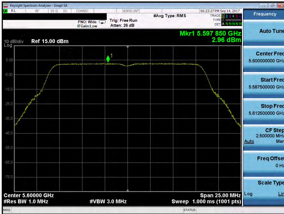
Plot 7-98. Power Spectral Density Plot (802.11a (UNII Band 2C) – Ch. 120)
