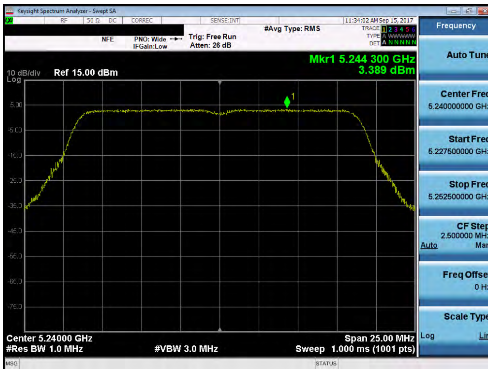
Plot 7-123. Power Spectral Density Plot (20MHz BW 802.11n (UNII Band 1) – Ch. 48)
