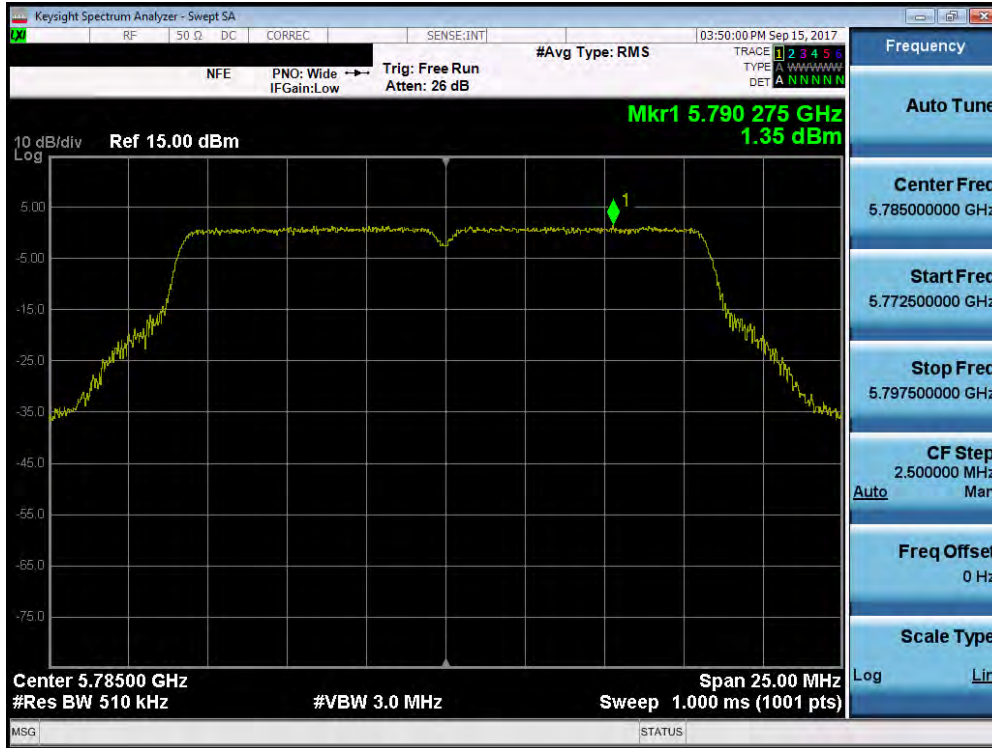
Plot 7-149. Power Spectral Density Plot (802.11a (UNII Band 3) – Ch. 157)
