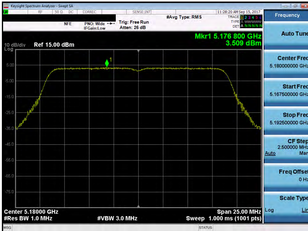
Plot 7-121. Power Spectral Density Plot (20MHz BW 802.11n (UNII Band 1) – Ch. 36)
