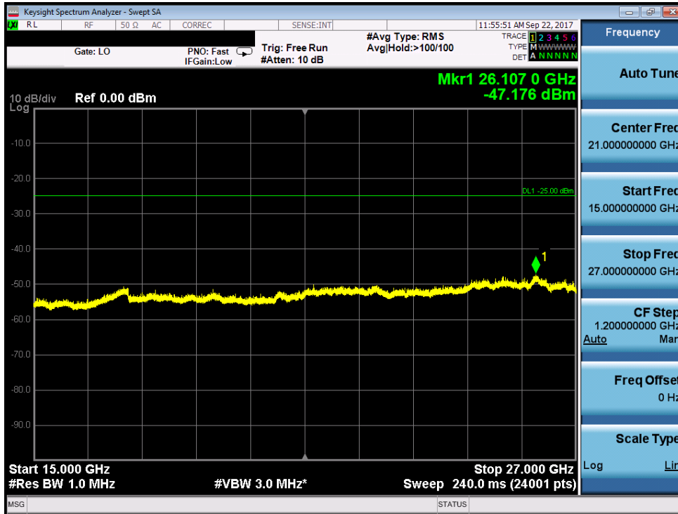
Plot 7-317. Conducted Spurious Plot (Band 41 – 20.0MHz QPSK – PCC 100/0 SCC 100/0 – Mid Channel)
