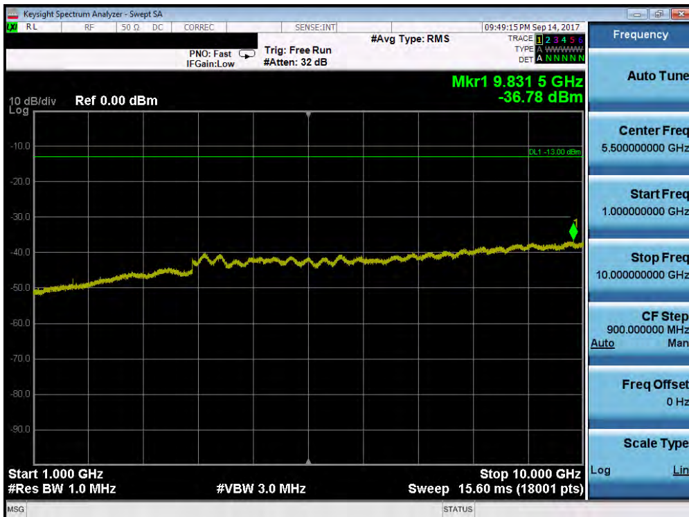
Plot 7-135. Conducted Spurious Plot (Band 5/26 – 10.0MHz QPSK – RB Size 1, RB Offset 0 – Low Channel)
