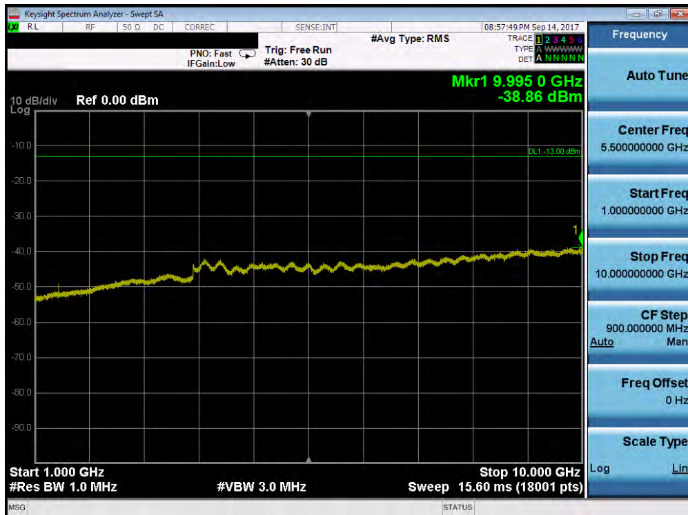
Plot 7-117. Conducted Spurious Plot (Band 12/17 – 10.0MHz QPSK – RB Size 1, RB Offset 0 – Low Channel)
