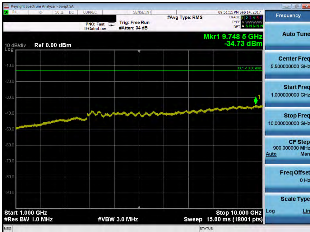
Plot 7-141. Conducted Spurious Plot (Band 5/26 – 10.0MHz QPSK – RB Size 1, RB Offset 0 – High Channel)
