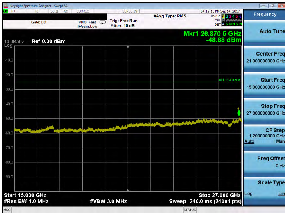
Plot 7-171. Conducted Spurious Plot (Band 38/41 – 20.0MHz QPSK – RB Size 1, RB Offset 0 – Low Channel)
