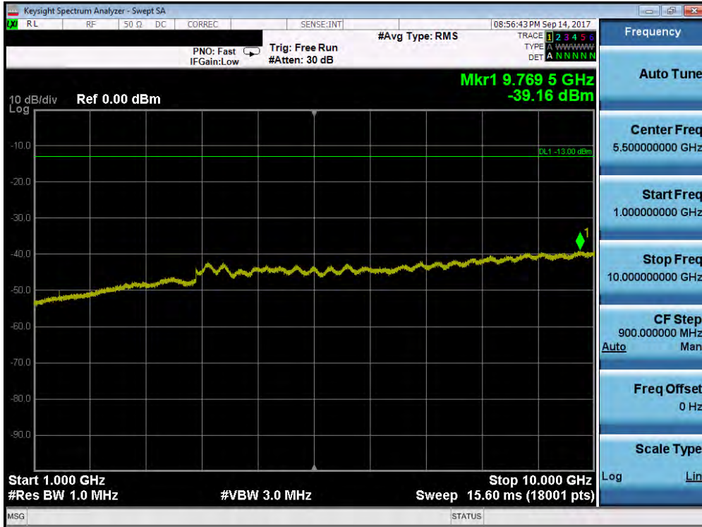
Plot 7-120. Conducted Spurious Plot (Band 12/17 – 10.0MHz QPSK – RB Size 1, RB Offset 0 – Mid Channel)
