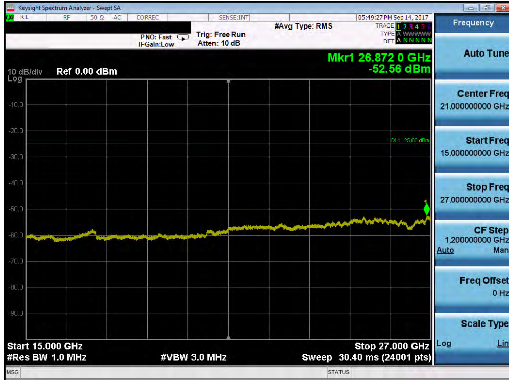
Plot 7-162. Conducted Spurious Plot (Band 7 – 20.0MHz QPSK – RB Size 1, RB Offset 0 – Low Channel)
