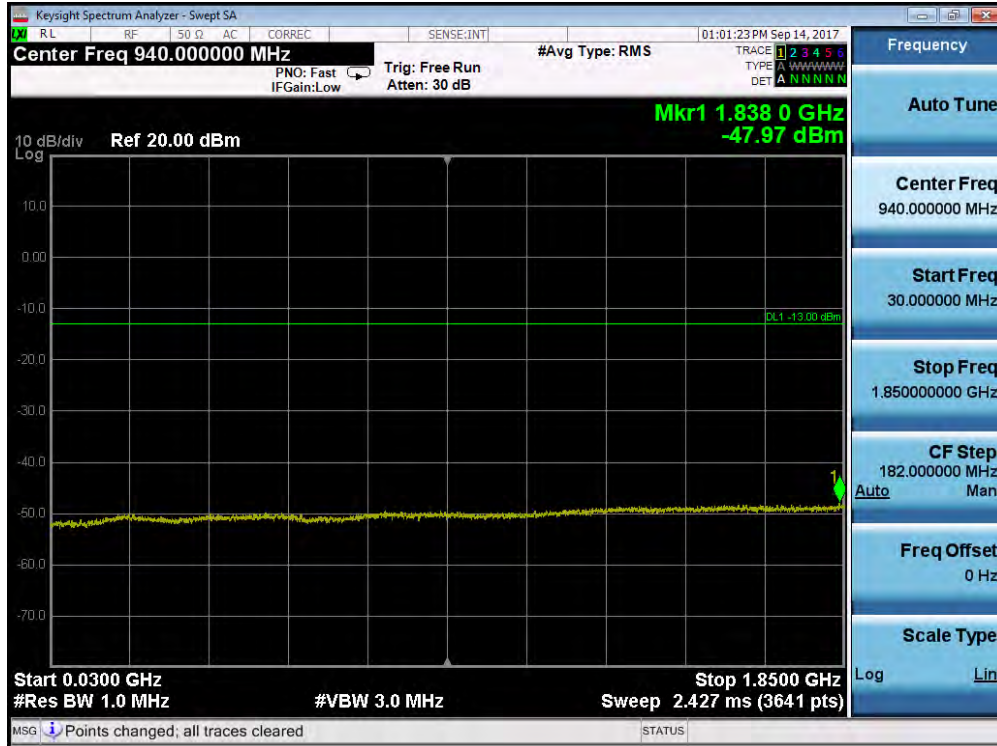
Plot 7-154. Conducted Spurious Plot (Band 2/25 – 20.0MHz QPSK – RB Size 1, RB Offset 0 – Mid Channel)
