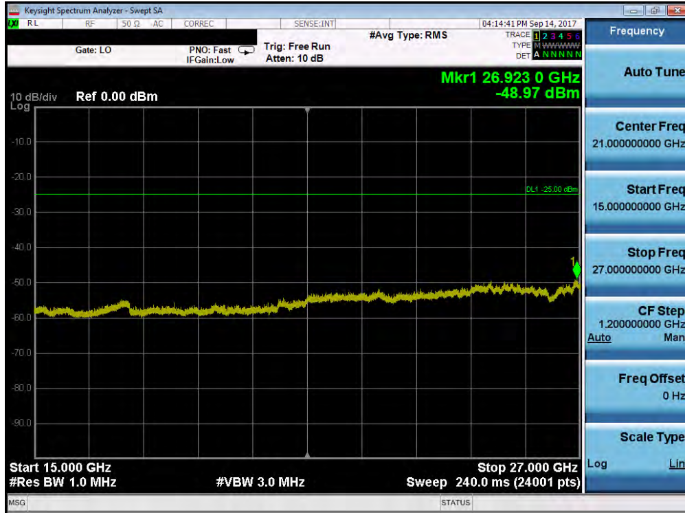
Plot 7-174. Conducted Spurious Plot (Band 38/41 – 20.0MHz QPSK – RB Size 1, RB Offset 0 – Mid Channel)
