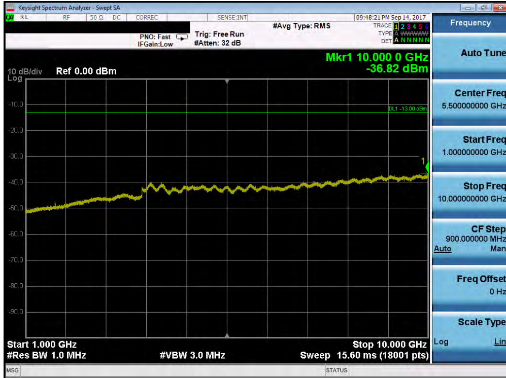
Plot 7-138. Conducted Spurious Plot (Band 5/26 – 10.0MHz QPSK – RB Size 1, RB Offset 0 – Mid Channel)
