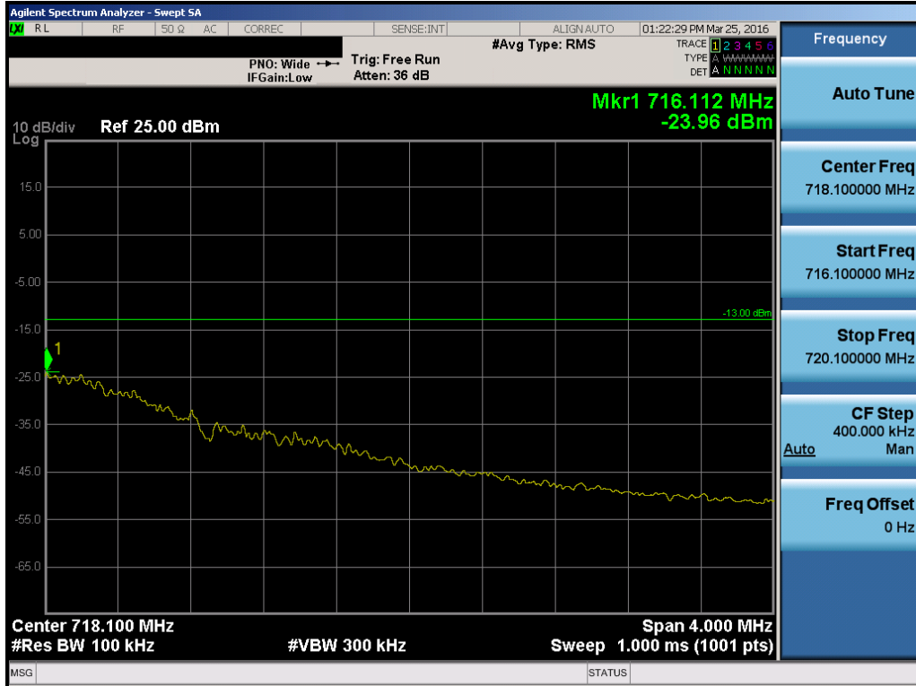
Plot 7-110. Upper Extended Band Edge Plot (Band 12 – 1.4MHz QPSK – RB Size 6)
