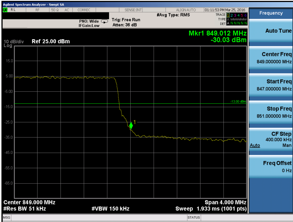
Plot 7-131. Upper Band Edge Plot (Band 5 – 5.0MHz QPSK – RB Size 25)
