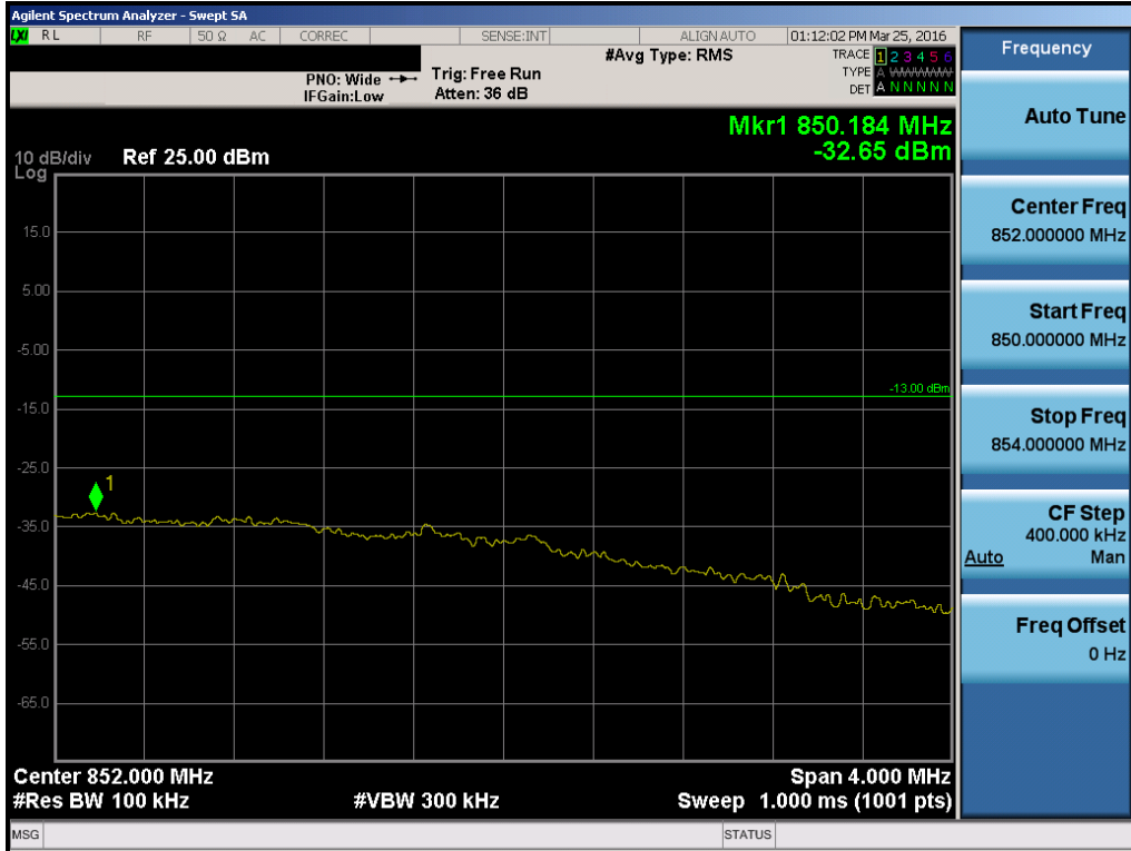
Plot 7-132. Upper Extended Band Edge Plot (Band 5 – 5.0MHz QPSK – RB Size 25)
