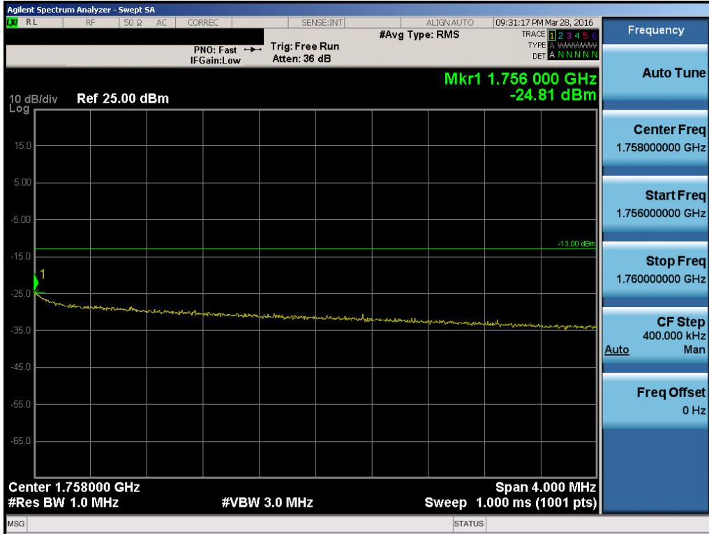
Plot 7-150. Upper Extended Band Edge Plot (Band 4 – 10.0MHz QPSK – RB Size 50)
