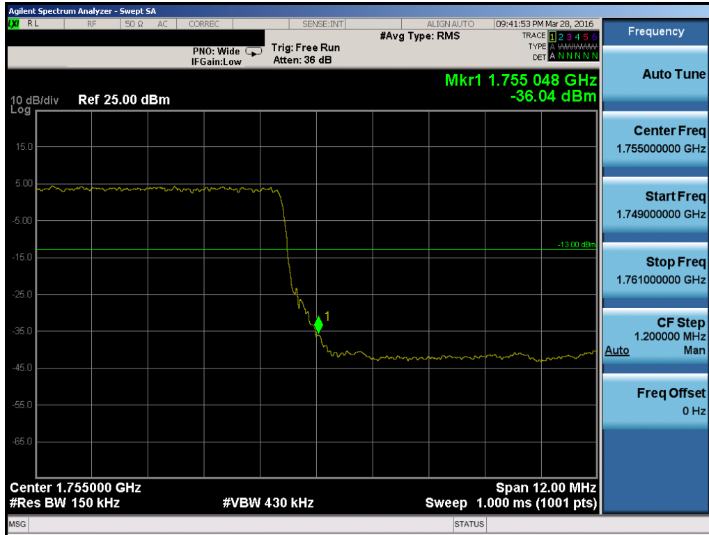
Plot 7-153. Upper Band Edge Plot (Band 4 – 15.0MHz QPSK – RB Size 75)
