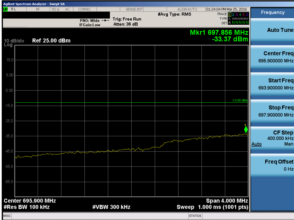
Plot 7-112. Lower Extended Band Edge Plot (Band 12 – 3.0MHz QPSK – RB Size 15)
