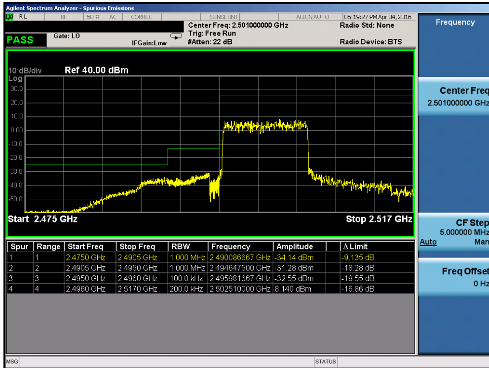
Plot 7-193. Lower ACP Plot (Band 41 – 10.0MHz QPSK – RB Size 50)
