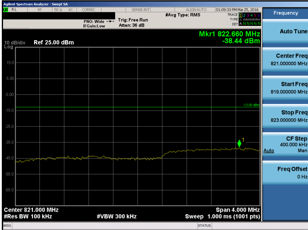
Plot 7-126. Lower Extended Band Edge Plot (Band 5 – 3.0MHz QPSK – RB Size 15)
