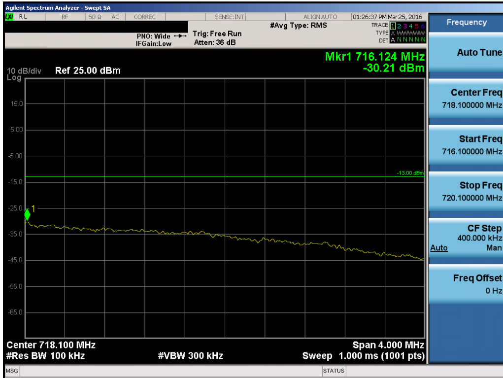
Plot 7-118. Upper Extended Band Edge Plot (Band 12 - 5.0MHz QPSK - RB Size 25)
