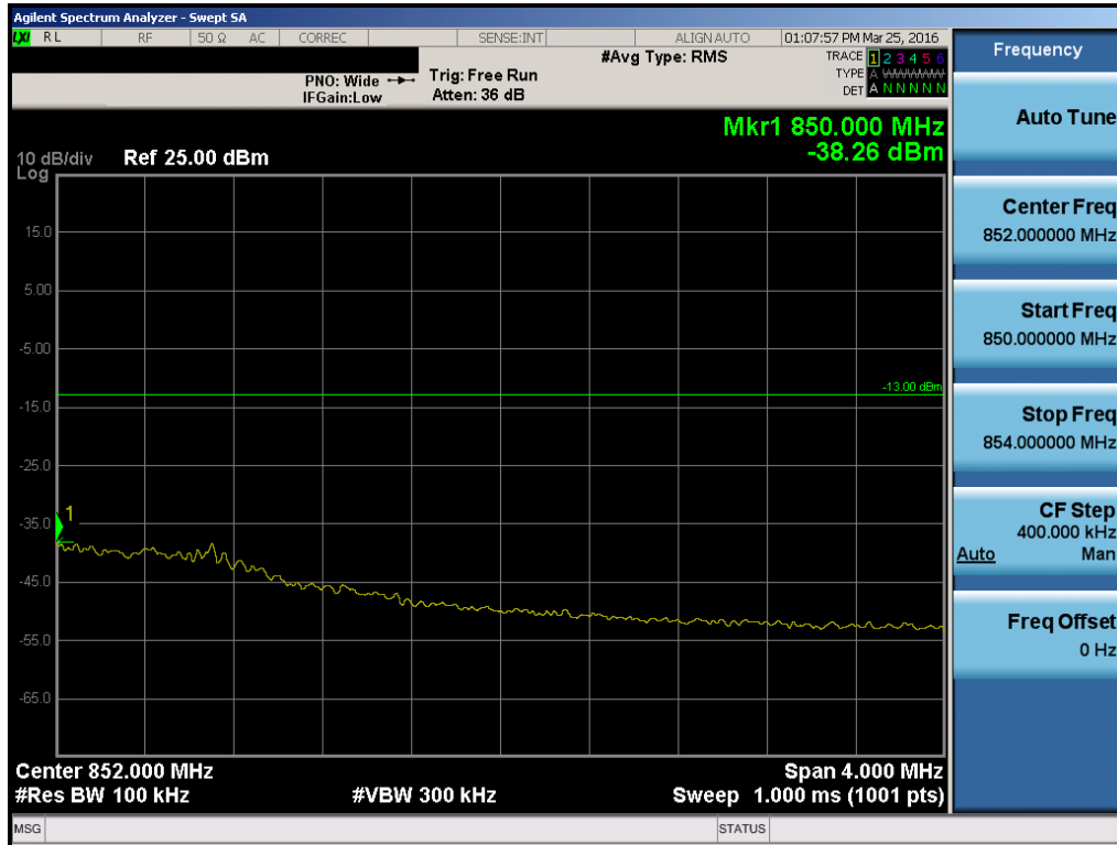
Plot 7-124. Upper Extended Band Edge Plot (Band 5 – 1.4MHz QPSK – RB Size 6)
