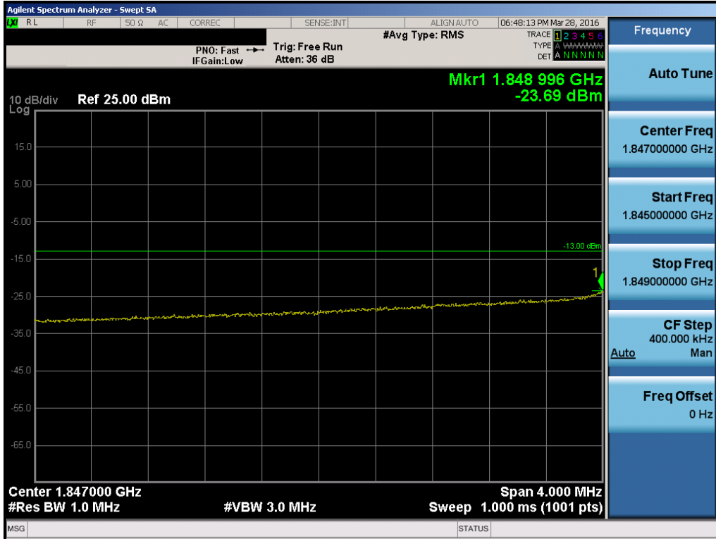
Plot 7-172. Lower Extended Band Edge Plot (Band 2 – 10.0MHz QPSK – RB Size 50)
