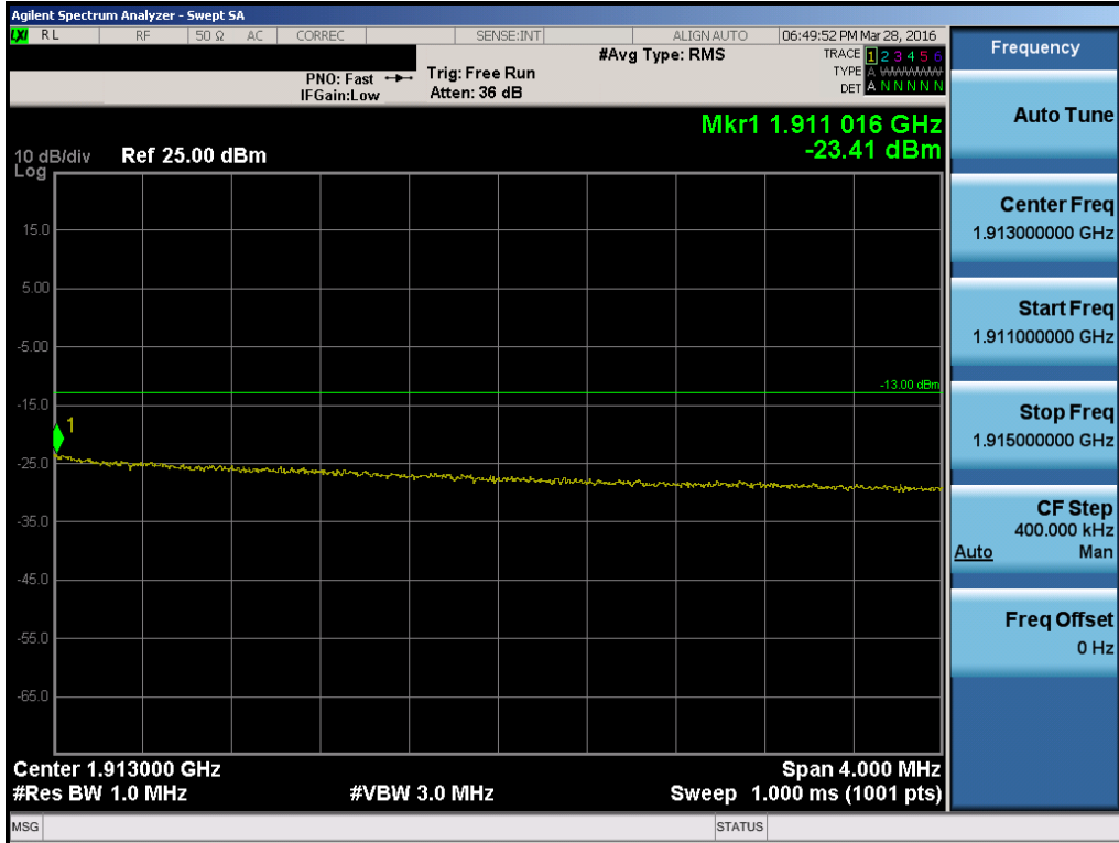
Plot 7-174. Upper Extended Band Edge Plot (Band 2 – 10.0MHz QPSK – RB Size 50)
