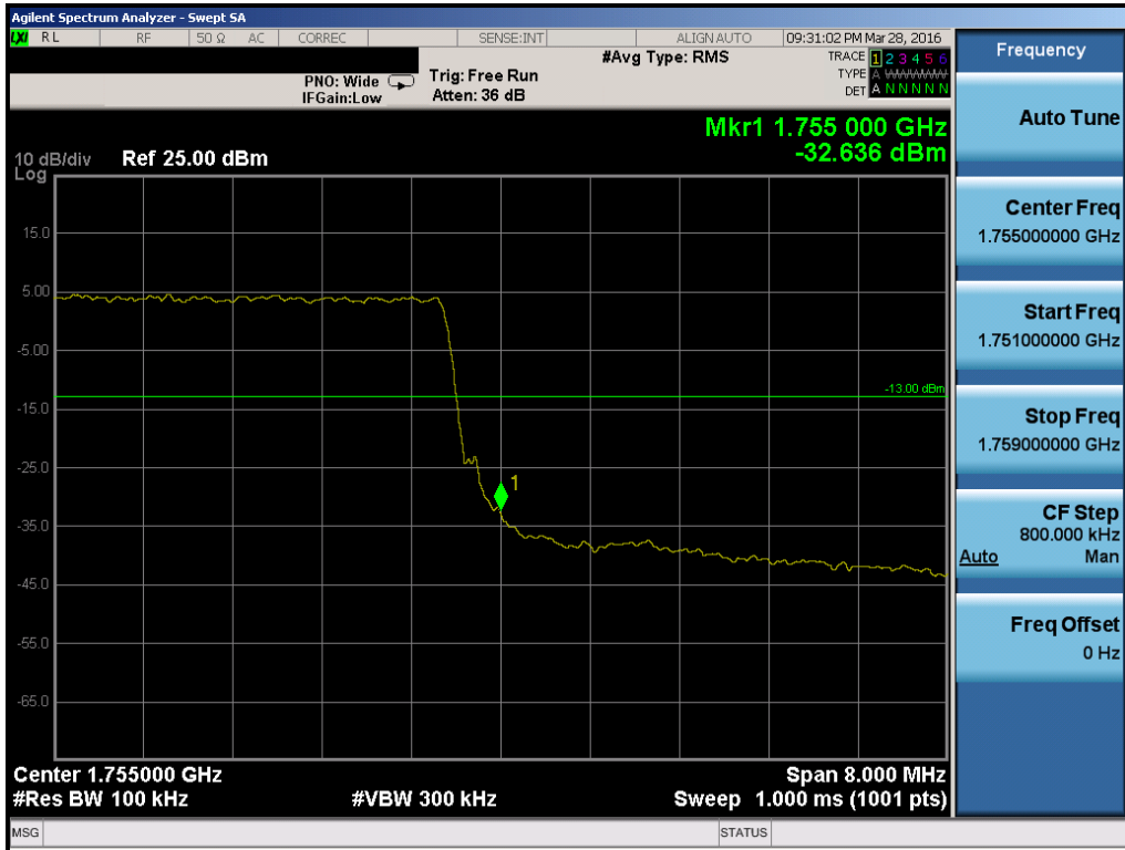
Plot 7-149. Upper Band Edge Plot (Band 4 – 10.0MHz QPSK – RB Size 50)
