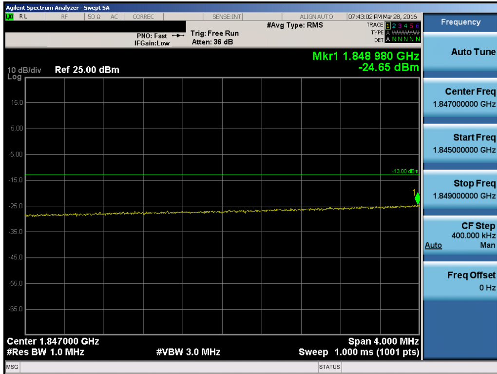
Plot 7-180. Lower Extended Band Edge Plot (Band 2 – 20.0MHz QPSK – RB Size 100)
