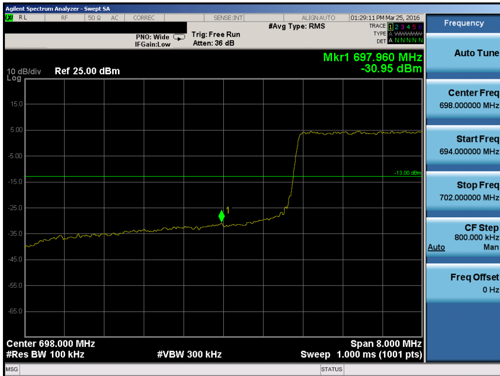
Plot 7-119. Lower Band Edge Plot (Band 12 - 10.0MHz QPSK - RB Size 50)
