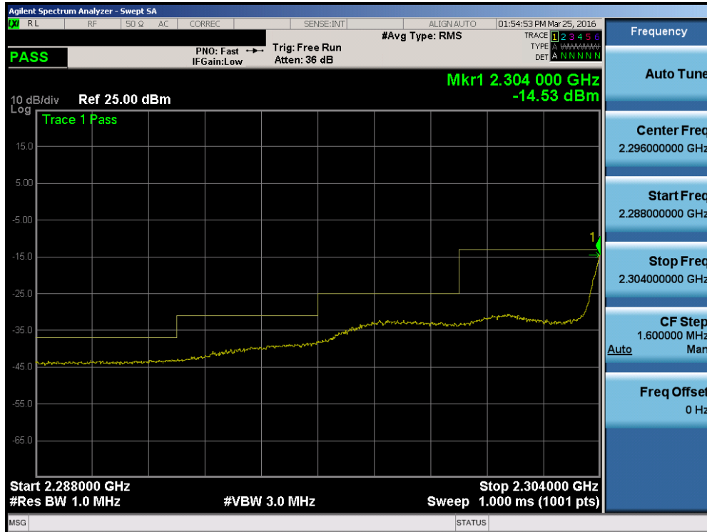
Plot 7-184. Lower Extended Band Edge Plot (Band 30 – 5.0MHz QPSK – RB Size 50)
