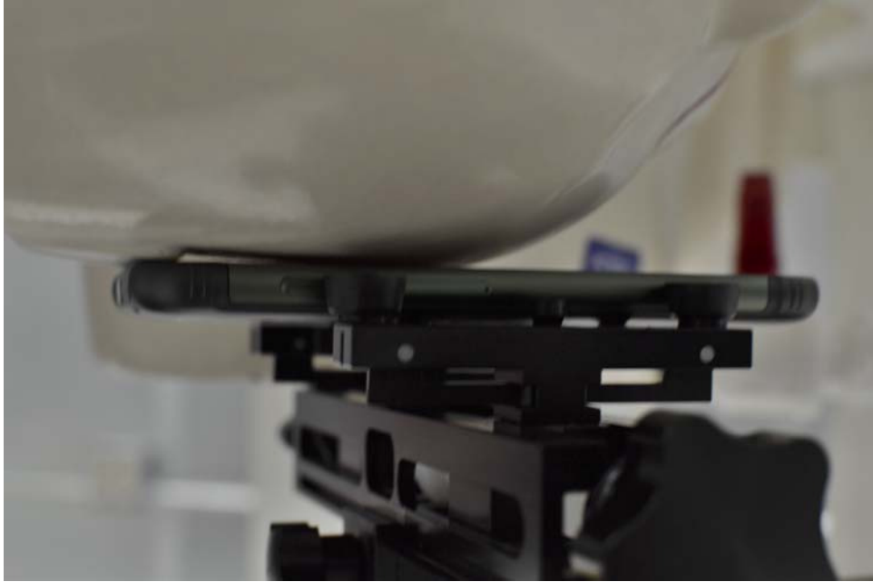
SAR Test Setup Photo 1: Right Cheek
