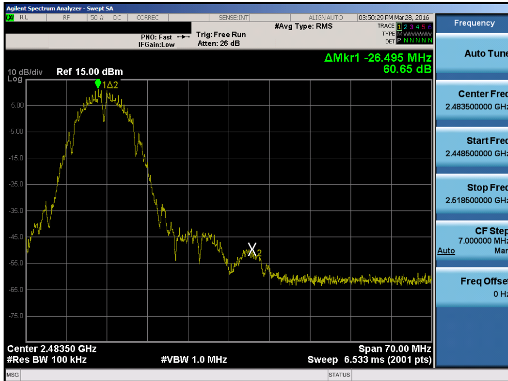
Plot 7-44. Band Edge Plot (802.11b – Ch. 11)
