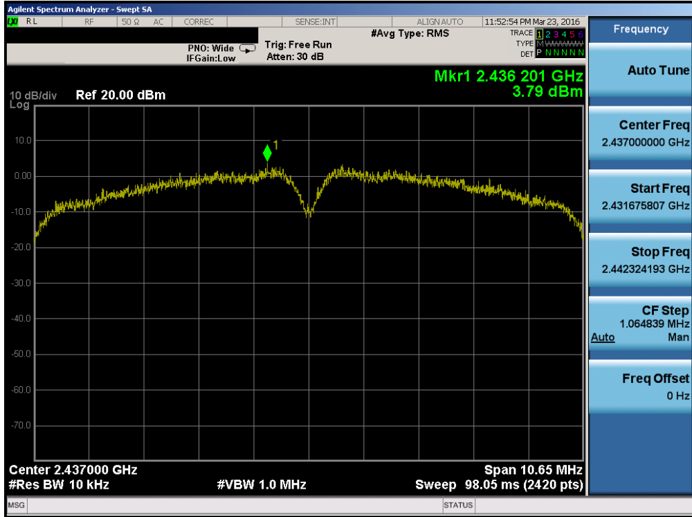
Plot 7-20. Power Spectral Density Plot (802.11b – Ch. 6)
