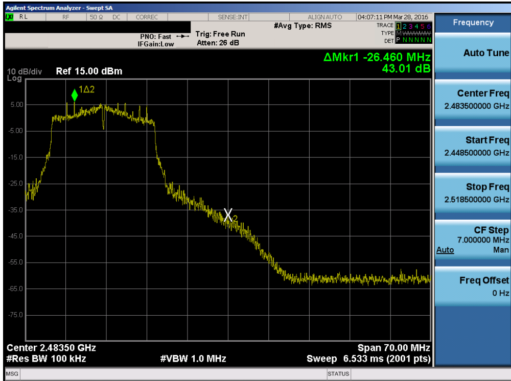
Plot 7-48. Band Edge Plot (802.11n (2.4GHz) – Ch. 11)
