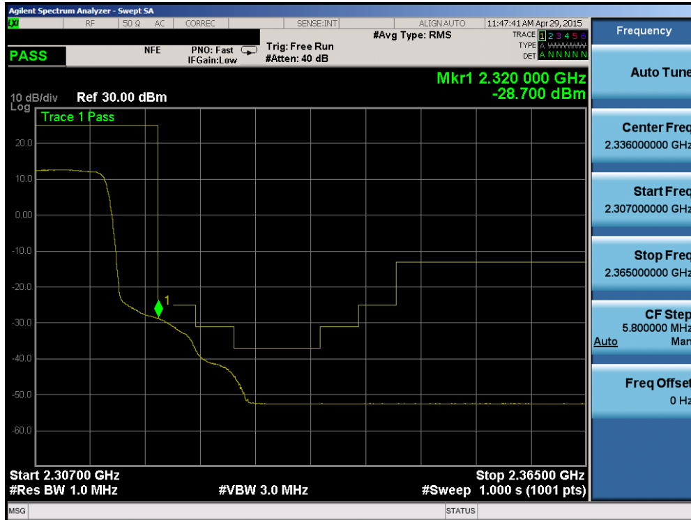
Plot 6-167. Upper Extended Band Edge Plot (Band 30 – 10MHz QPSK – RB Size 50)
