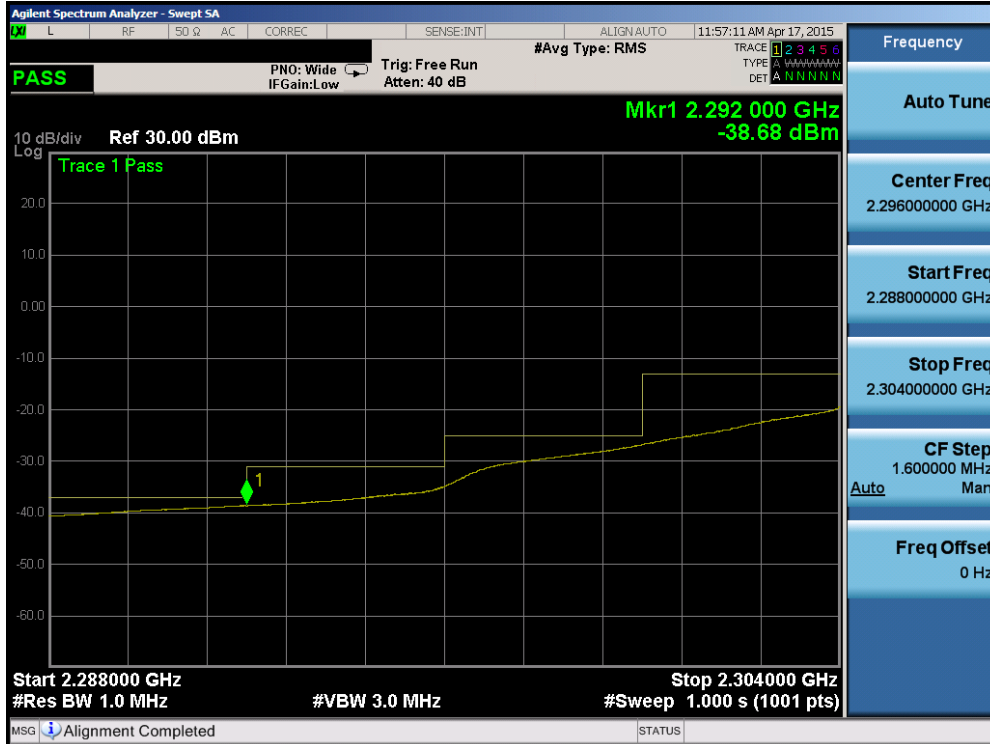
Plot 6-165. Lower Extended Band Edge Plot (Band 30 – 10MHz QPSK – RB Size 50)
