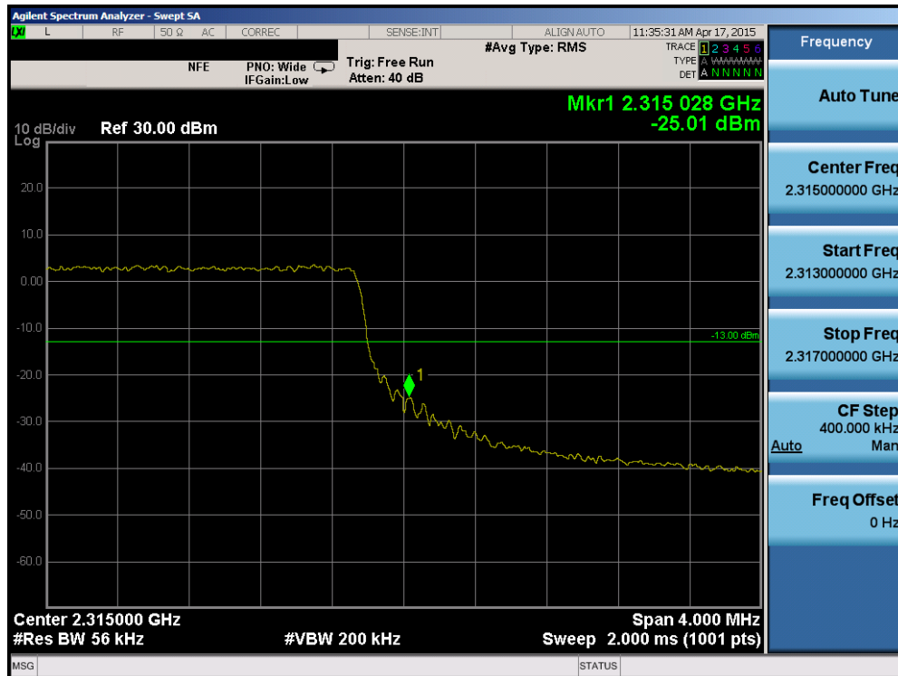
Plot 6-162. Upper Band Edge Plot (Band 30 – 5MHz QPSK – RB Size 25)
