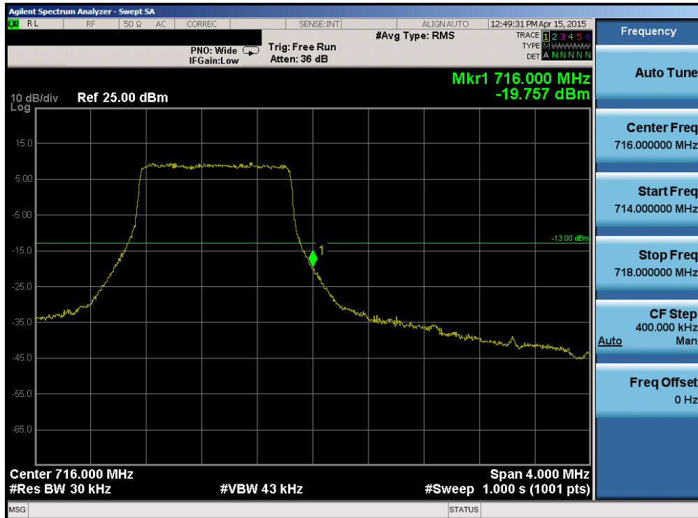
Plot 6-86. Upper Band Edge Plot (Band 12 – 1.4MHz QPSK – RB Size 6)
