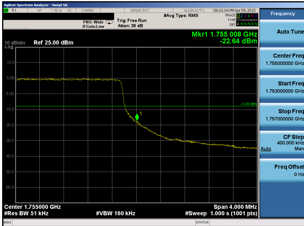
Plot 6-122. Upper Band Edge Plot (Band 4 – 5.0MHz QPSK – RB Size 25)
