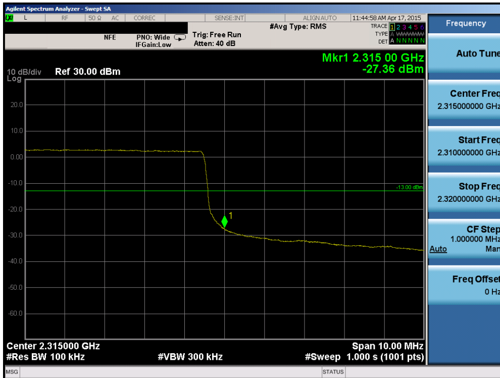
Plot 6-166. Upper Band Edge Plot (Band 30 – 10MHz QPSK – RB Size 50)
