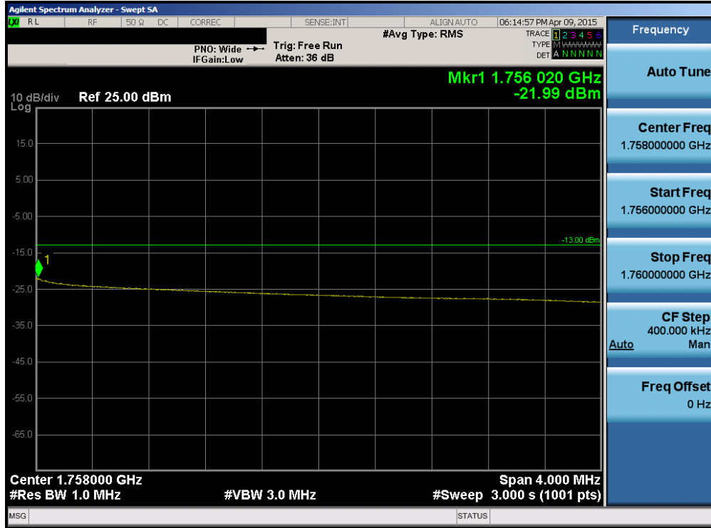
Plot 6-127. Upper Extended Band Edge Plot (Band 4 – 10.0MHz QPSK – RB Size 50)
