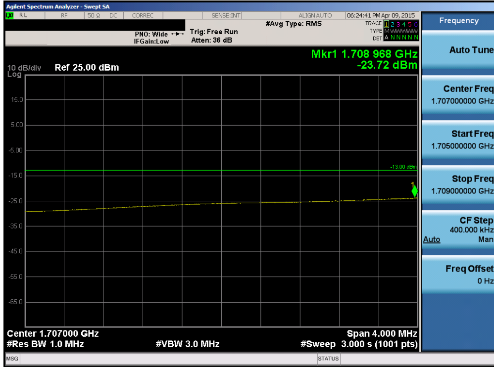
Plot 6-129. Lower Extended Band Edge Plot (Band 4 – 15.0MHz QPSK – RB Size 75)
