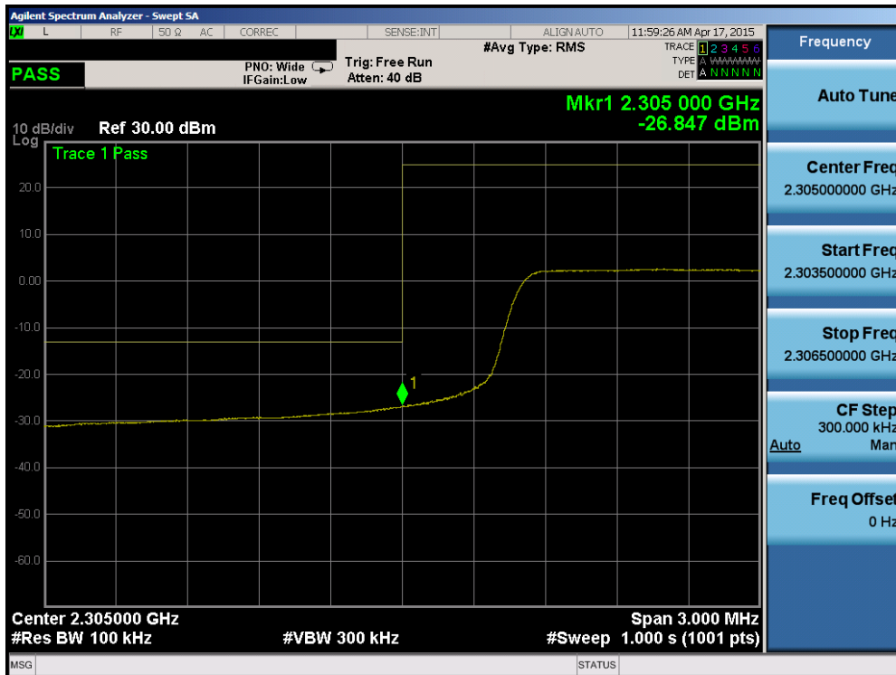
Plot 6-164. Lower Band Edge Plot (Band 30 – 10MHz QPSK – RB Size 50)
