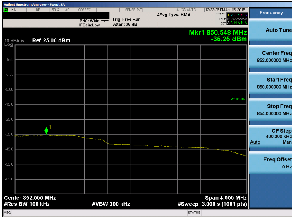
Plot 6-105. Upper Extended Band Edge Plot (Band 5 – Band 5 – 3.0MHz QPSK – RB Size 15)
