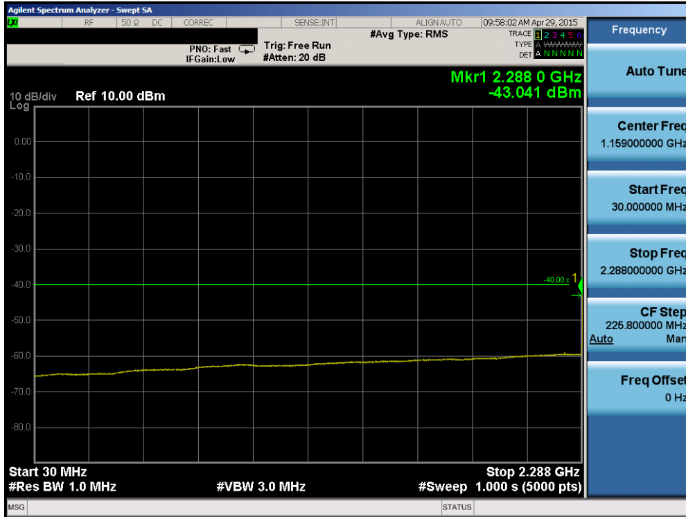
Plot 6-81. Conducted Spurious Plot (Band 30 – 10.0MHz QPSK – RB Size 1, RB Offset 0 – Mid Channel)
