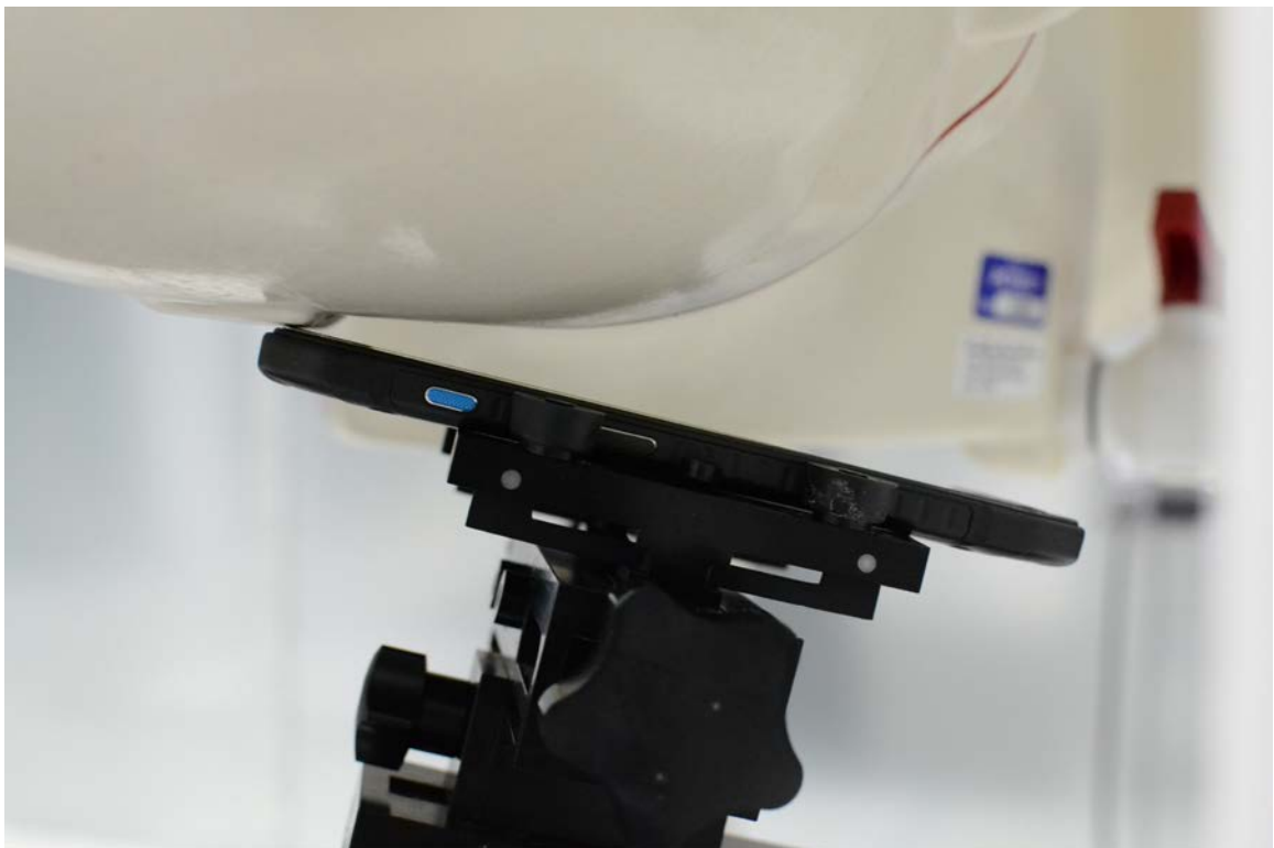
SAR Test Setup Photo 2: Right Tilt
