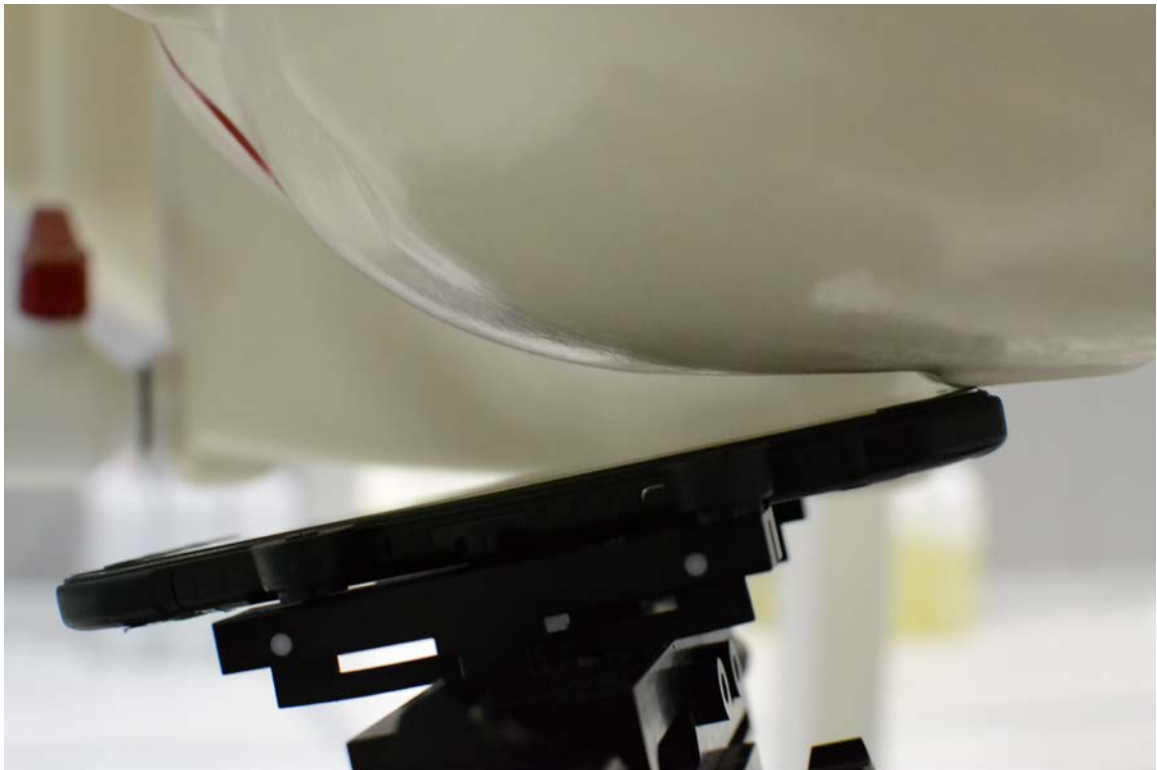
SAR Test Setup Photo 4: Left Tilt
