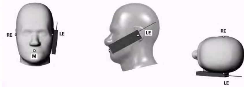
Figure 6-1 Front, Side and Top View of Cheek Position
