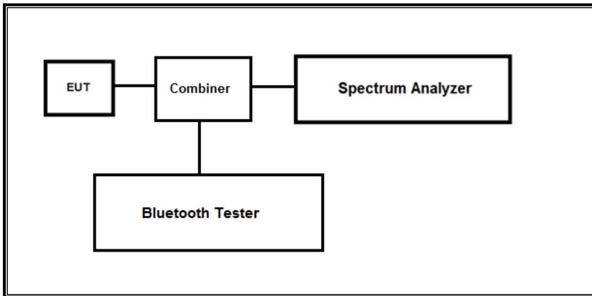
**SETUP DIAGRAM FOR TESTS (RADIATED TEST SETUP)**
