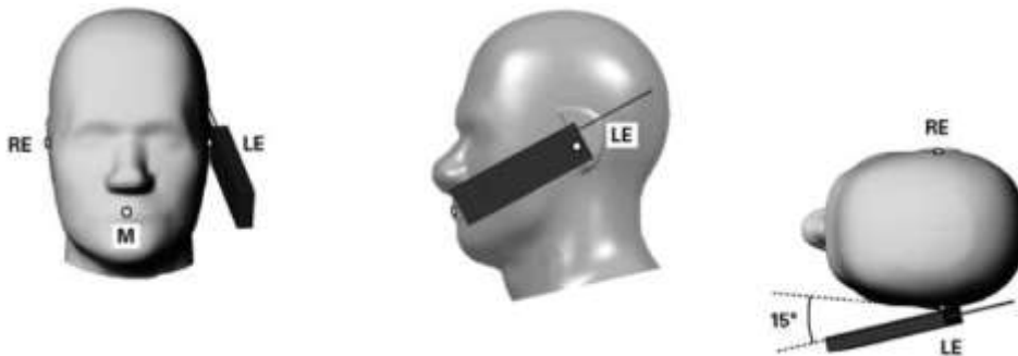
Figure 6.5. Tilt 15° position of the wireless device
