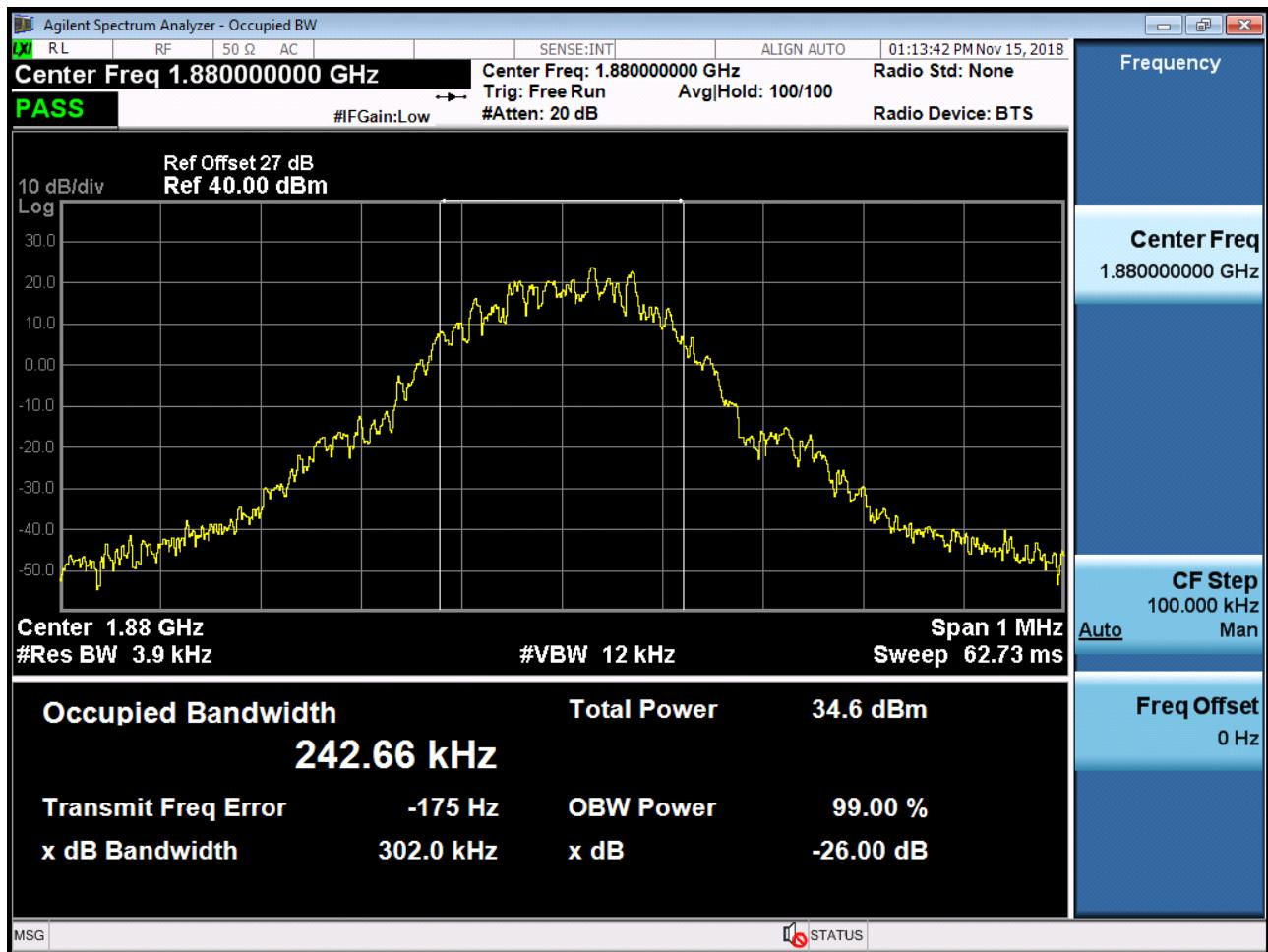
■ GSM1900 MODE (810 CH.) Occupied Bandwidth
