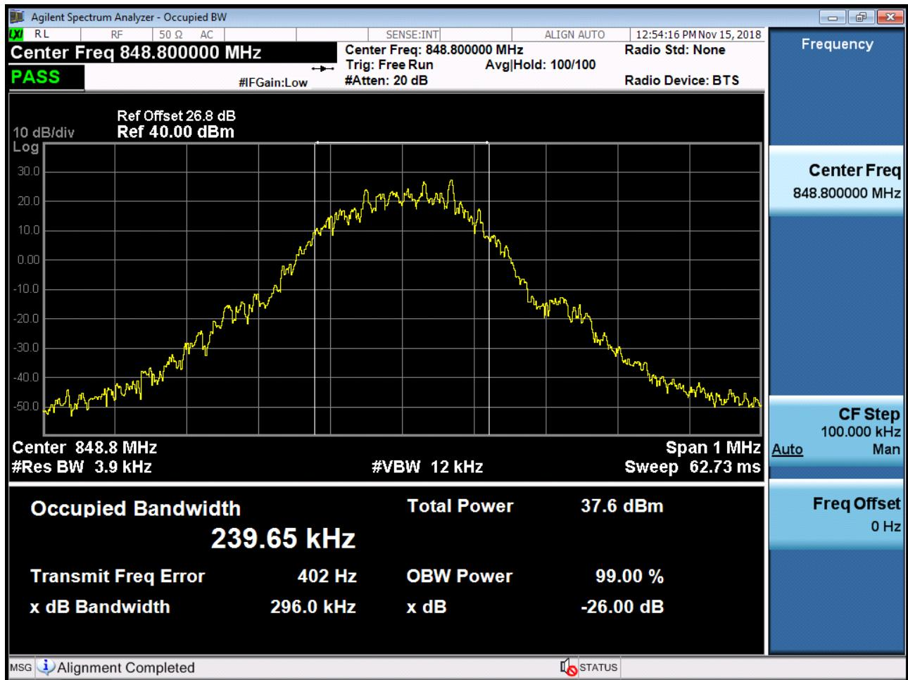
■ GSM850 EDGE (128 CH.) Occupied Bandwidth
