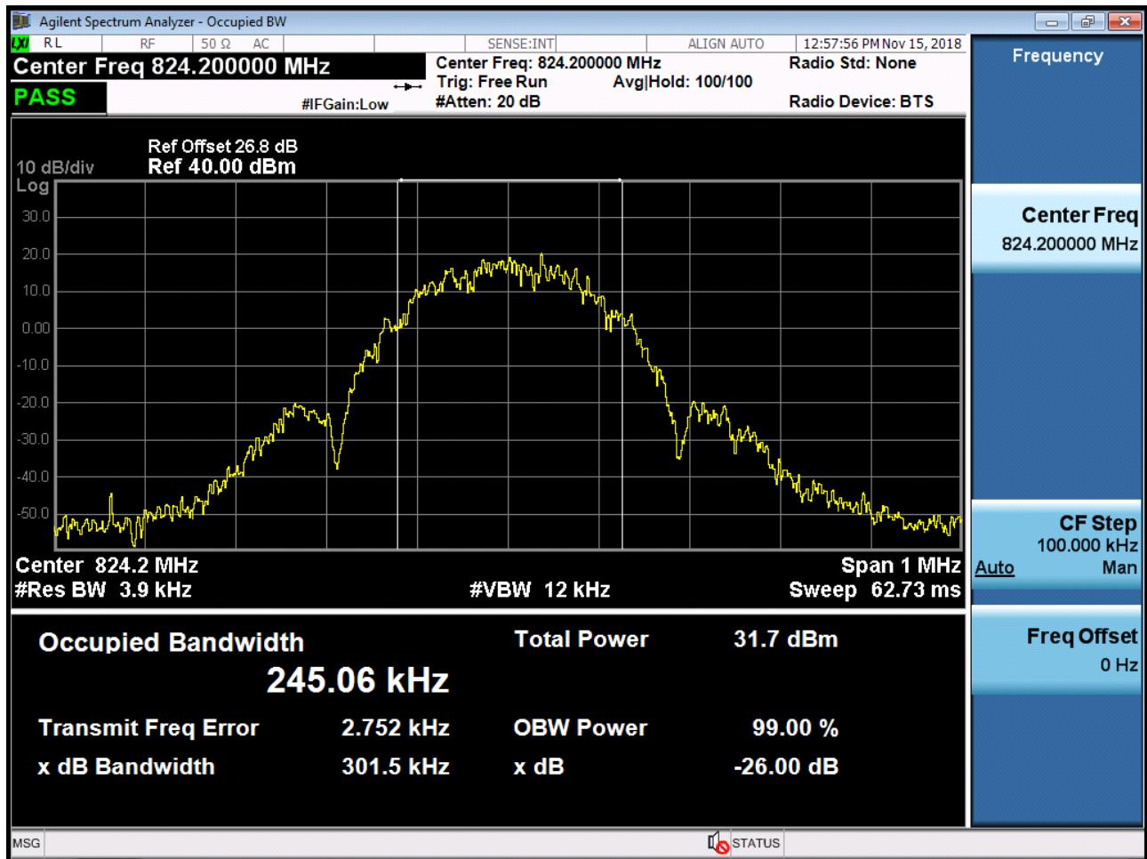
■ GSM1900 MODE (512 CH.) Occupied Bandwidth
