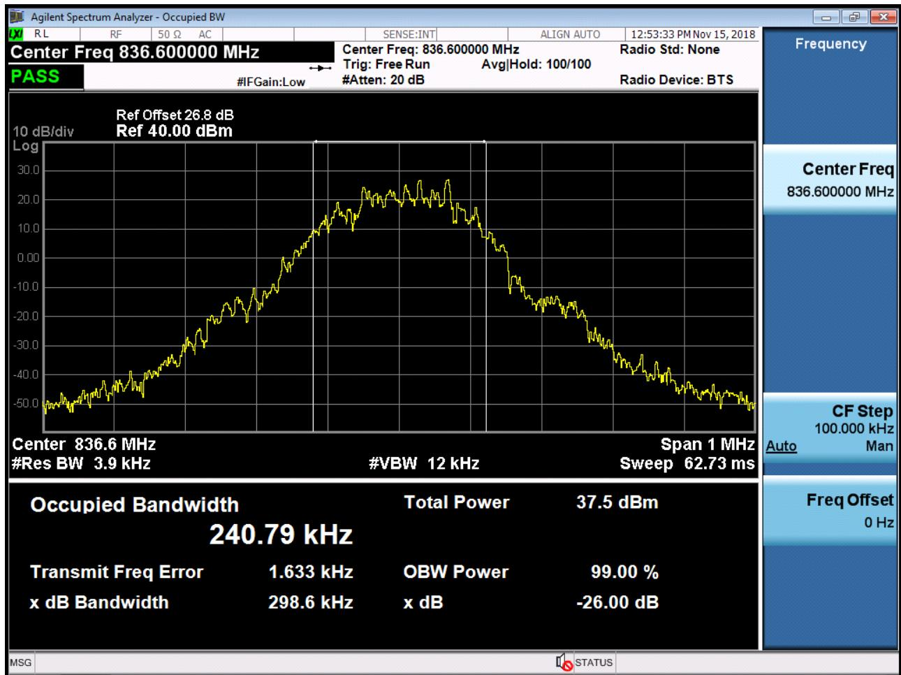
■ GSM850 MODE (251 CH.) Occupied Bandwidth
