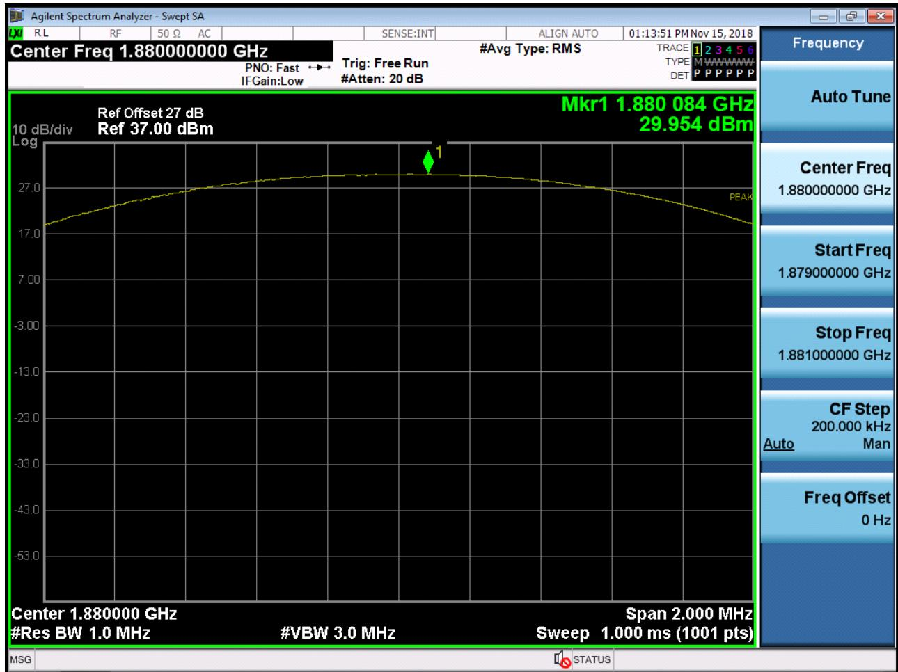
■ GSM1900 MODE (661 CH.) Peak-to-Average Ratio P<sub>Avg</sub>
