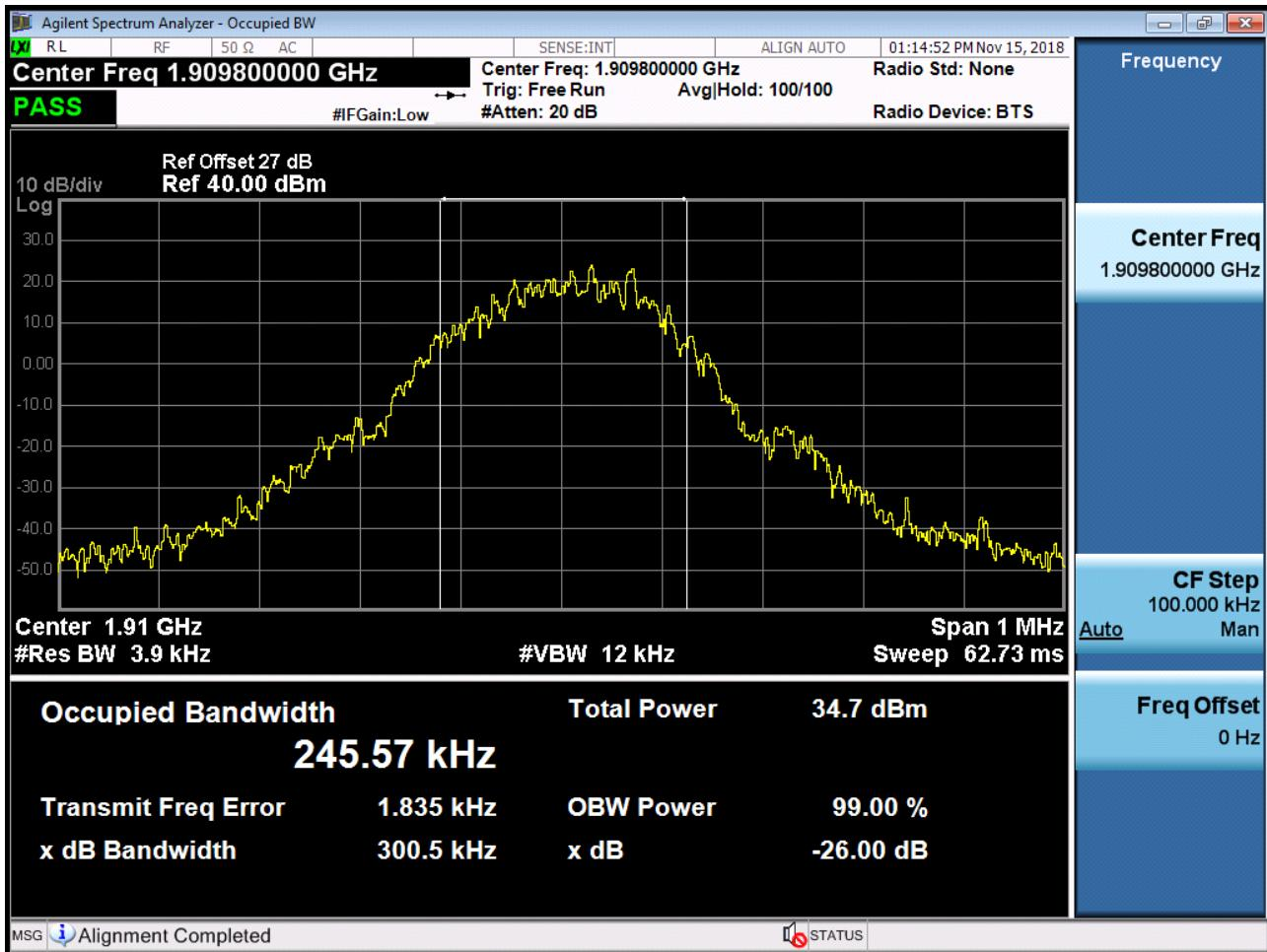
■ GSM1900 EDGE (810 CH.) Occupied Bandwidth
