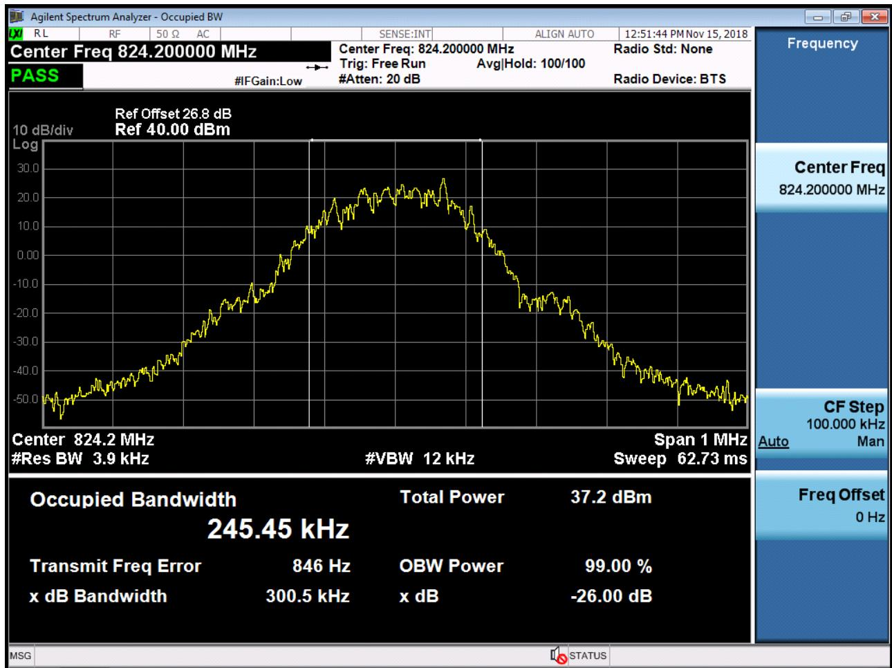
■ GSM850 MODE (190 CH.) Occupied Bandwidth
