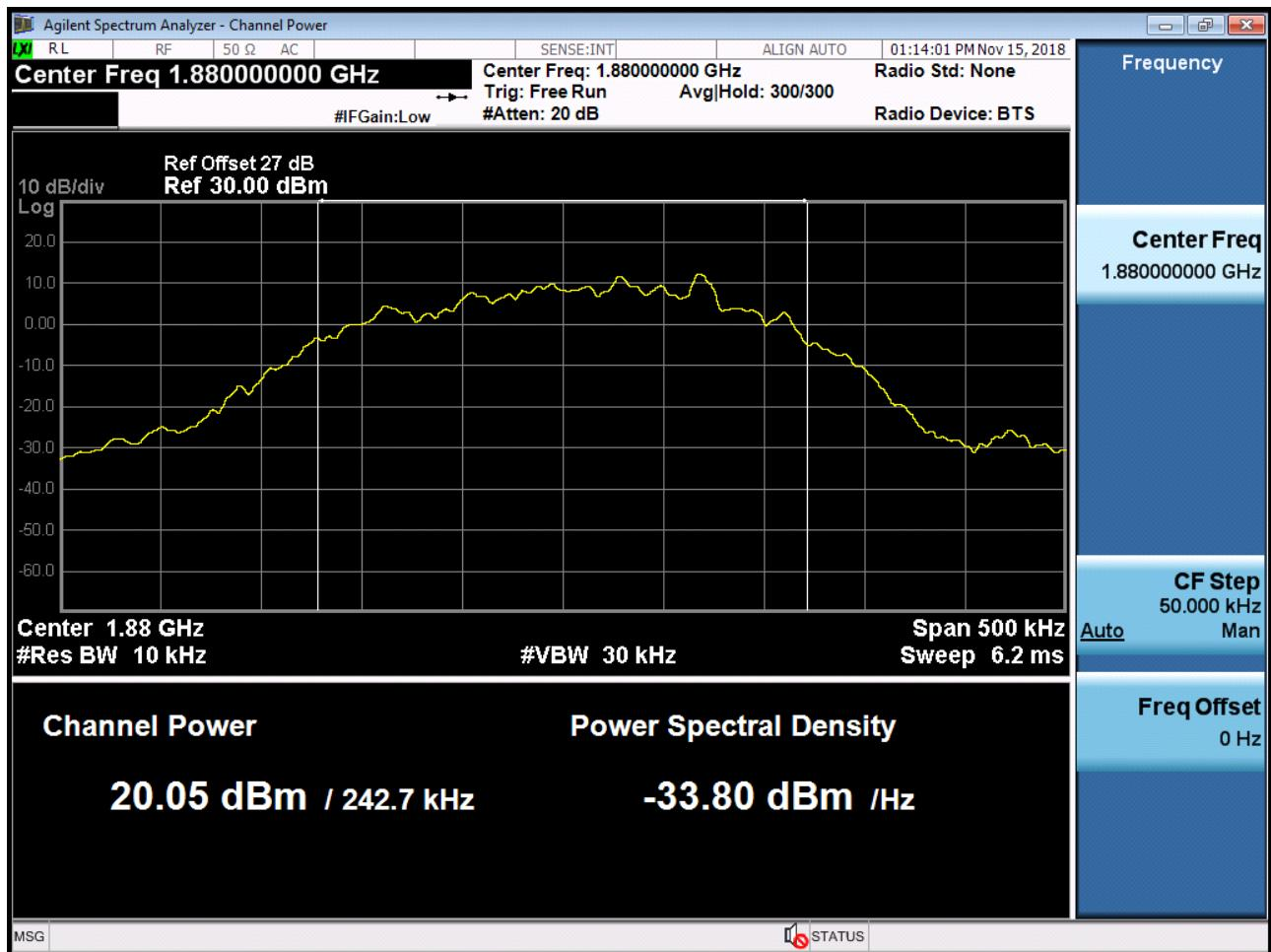
■ GSM1900 MODE (661 CH.) Peak-to-Average Ratio Duty
