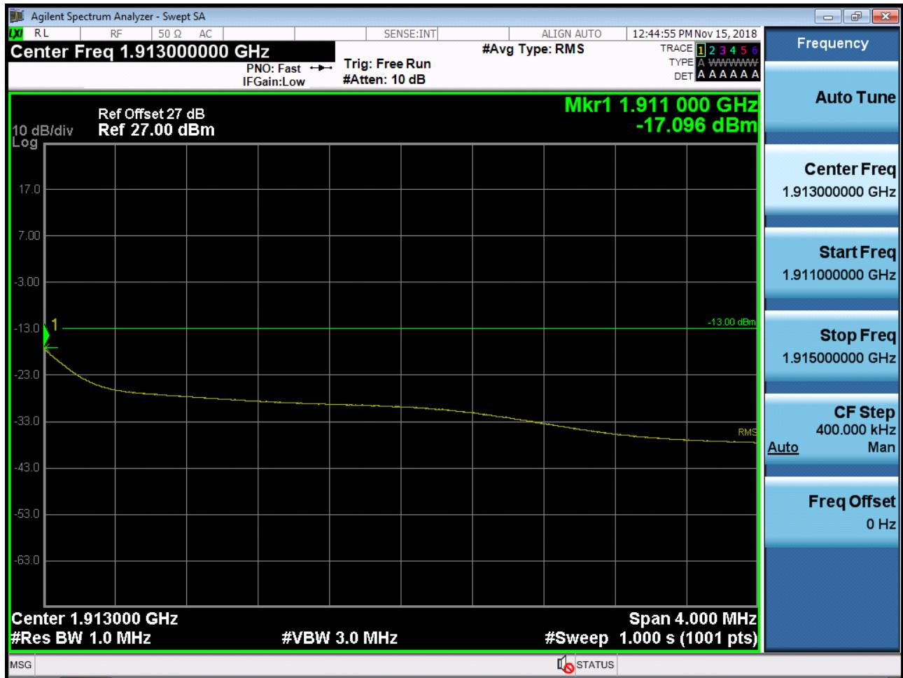
■ GSM850 MODE (128 CH.) Conducted Spurious Emissions
