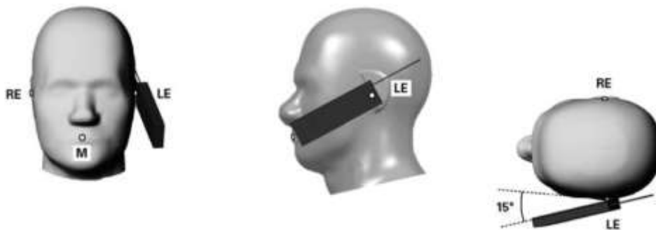
Figure 6.5. Tilt 15° position of the wireless device
