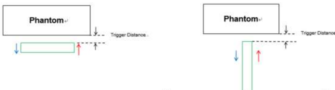
Proximity Sensor Trigger Distance Assessment KDB 616217 D04 §6.2 (Rear /Front/Bottom)
