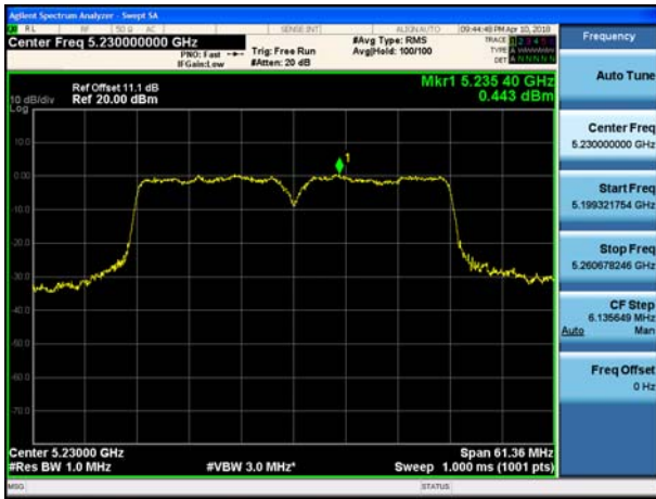
802.11n_HT40 UNII 2C BAND PSD CH 134
