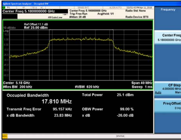
802.11ac_VHT20 UNII 2C BAND 26dB Bandwidth(CH 140)
