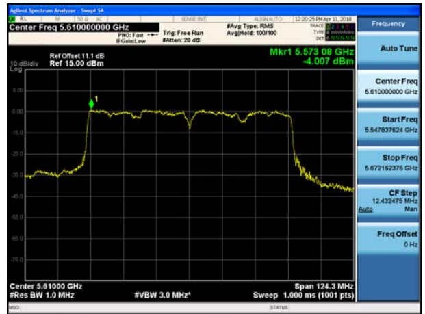
802.11ac_VHT80 UNII 3 BAND PSD CH 122
