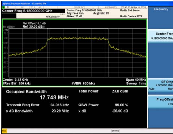
802.11n_HT20 UNII 2C BAND 26dB Bandwidth(CH 100)
