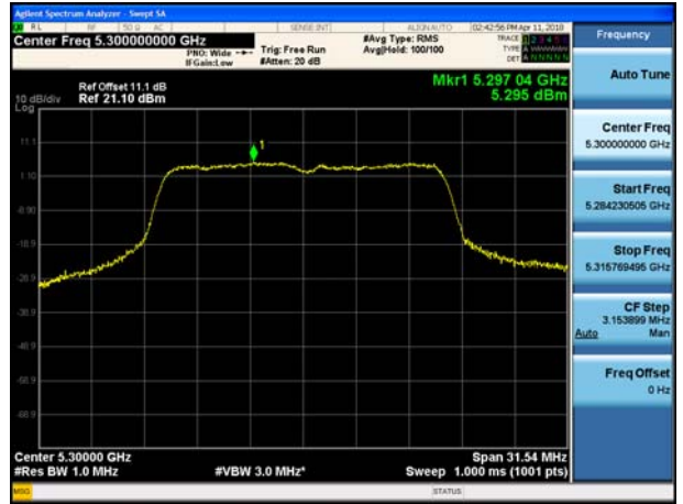
802.11a UNII 3 BAND PSD CH 149
