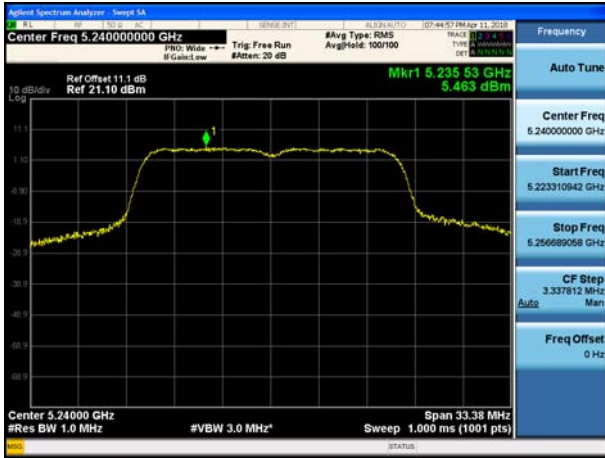
802.11n_HT20 UNII 2C BAND PSD CH 120
