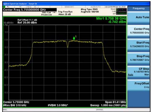
802.11n_HT40 UNII 3 BAND PSD CH 151
