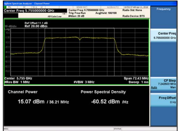
802.11ac_VHT40 UNII 3 BAND Average Power (5755 MHz ~5795 MHz) CH 151 MCS2
