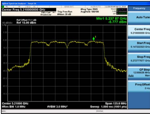
802.11ac_VHT80 UNII 2C BAND PSD CH 106
