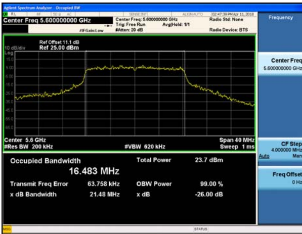
802.11a UNII 2C BAND 26dB Bandwidth (CH120)
