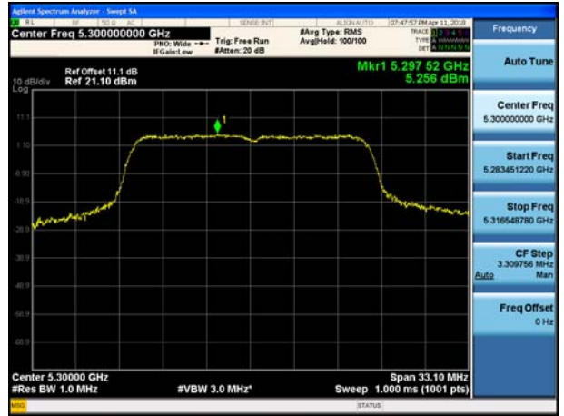
802.11n_HT20 UNII 3 BAND PSD CH 149
