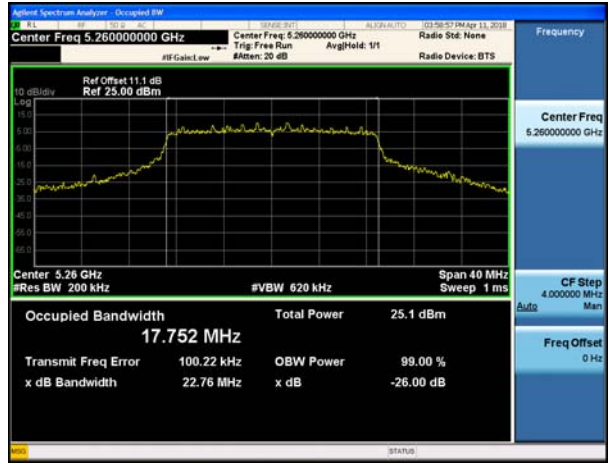
802.11ac_VHT20 UNII 3 BAND 26dB Bandwidth(CH 165)
