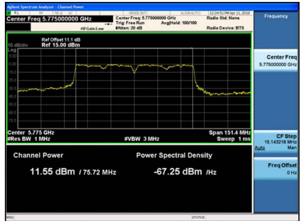
802.11ac_VHT80 UNII 3 BAND Average Power (5775 MHz) CH 155 MCS2
