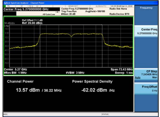
802.11ac_VHT40 UNII 3 BAND Average Power (5755 MHz ~5795 MHz) CH 151 MCS2
