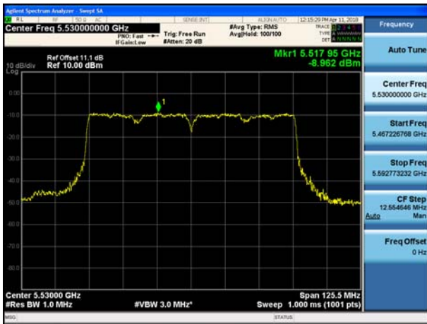
802.11ac_VHT80 UNII 3 BAND PSD CH 155
