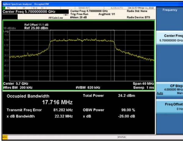
802.11ac_VHT20 UNII 2C BAND 26dB Bandwidth(CH 140)
