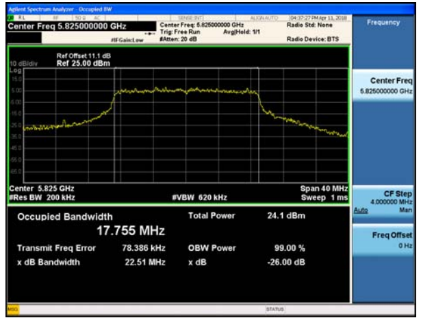
802.11ac_VHT20 UNII 3 BAND 26dB Bandwidth(CH 165)
