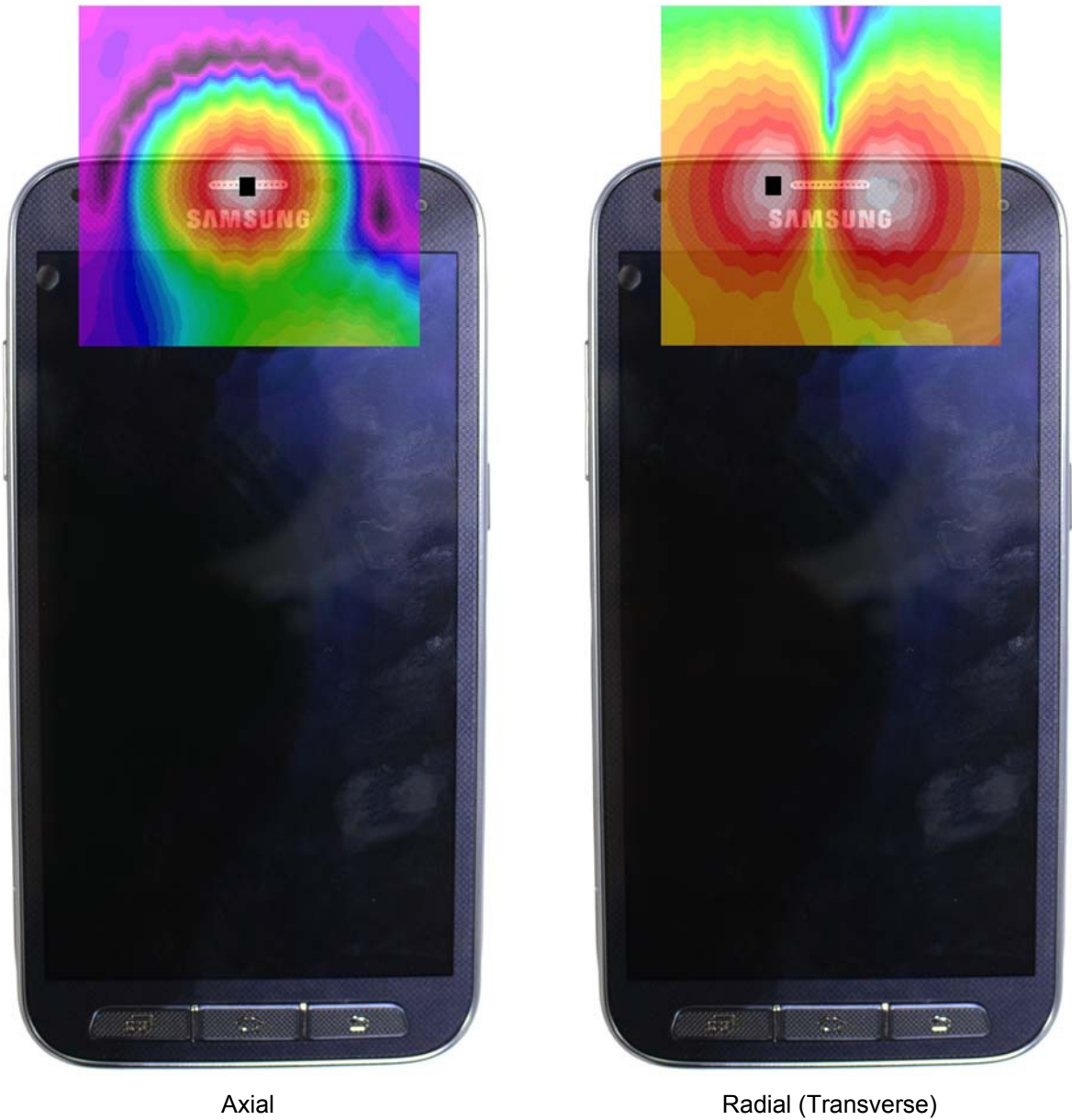
Figure 13-3 T-Coil Scan Overlay Magnetic Field Distributions
