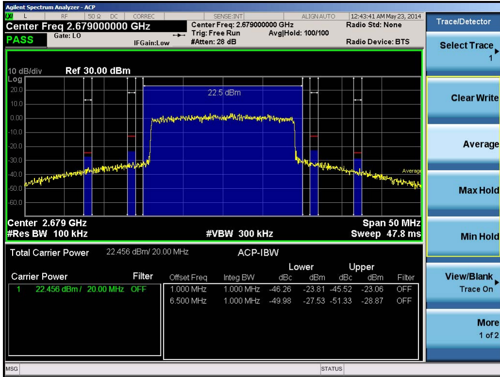
Plot 6-108. Upper ACP Plot (Band 41 – 20.0MHz QPSK – RB Size 100)
