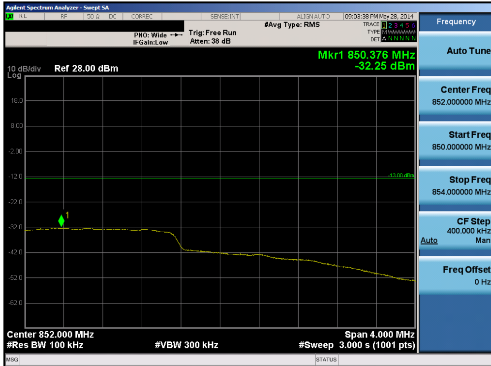
Plot 6-66. Upper Extended Band Edge Plot (Band 26 – Band 5 – 3.0MHz QPSK – RB Size 15)
