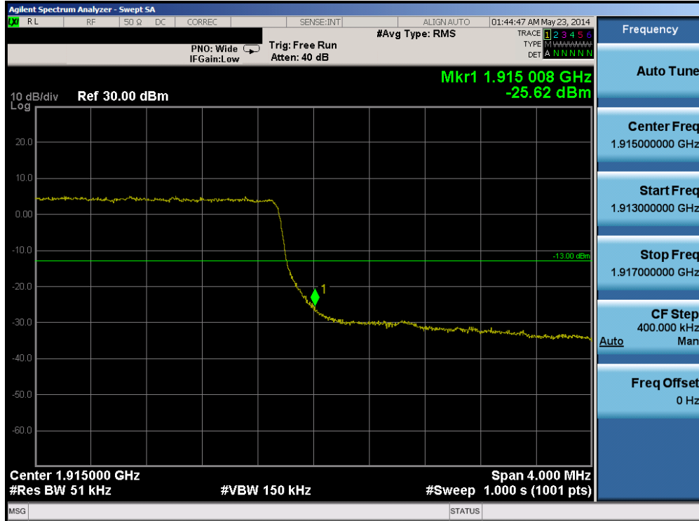
Plot 6-83. Upper Band Edge Plot (Band 25 – 5.0MHz QPSK – RB Size 25)
