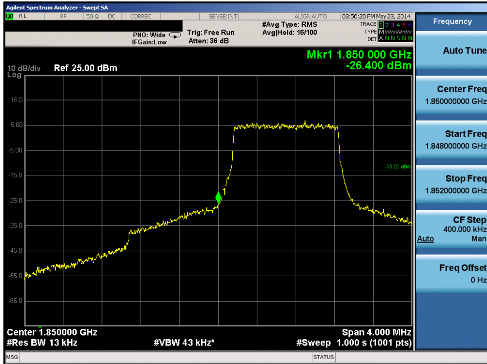
Plot 6-73. Lower Band Edge Plot (Band 25 – 1.4MHz QPSK – RB Size 6)
