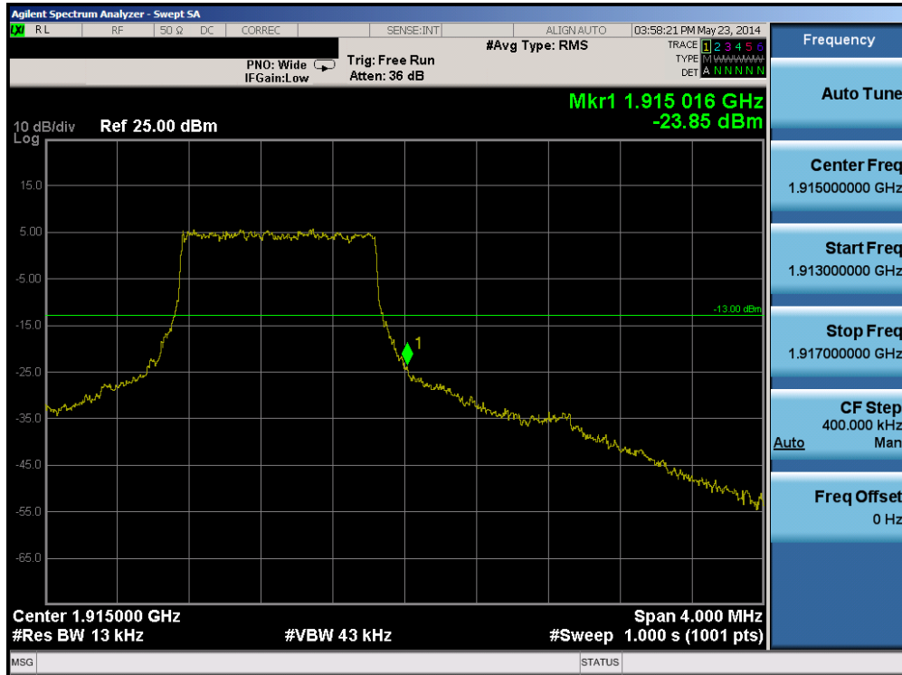
Plot 6-75. Upper Band Edge Plot (Band 25 – 1.4MHz QPSK – RB Size 6)
