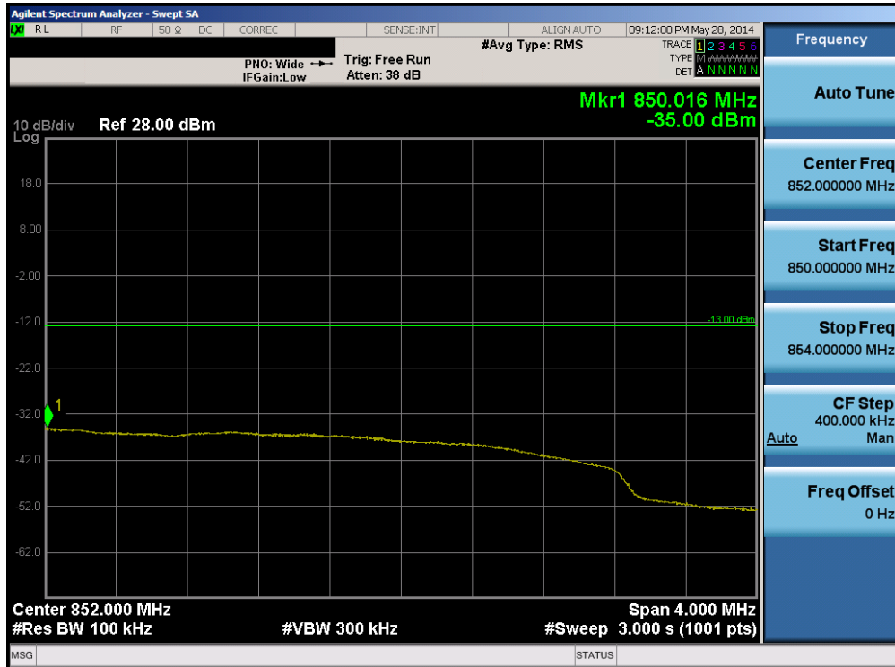
Plot 6-70. Upper Extended Band Edge Plot (Band 26 – 5.0MHz QPSK – RB Size 25)
