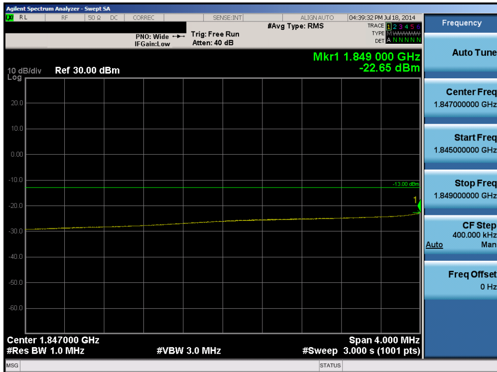
Plot 6-62. Lower Extended Band Edge Plot (Band 2 – 10.0MHz QPSK – RB Size 50)
