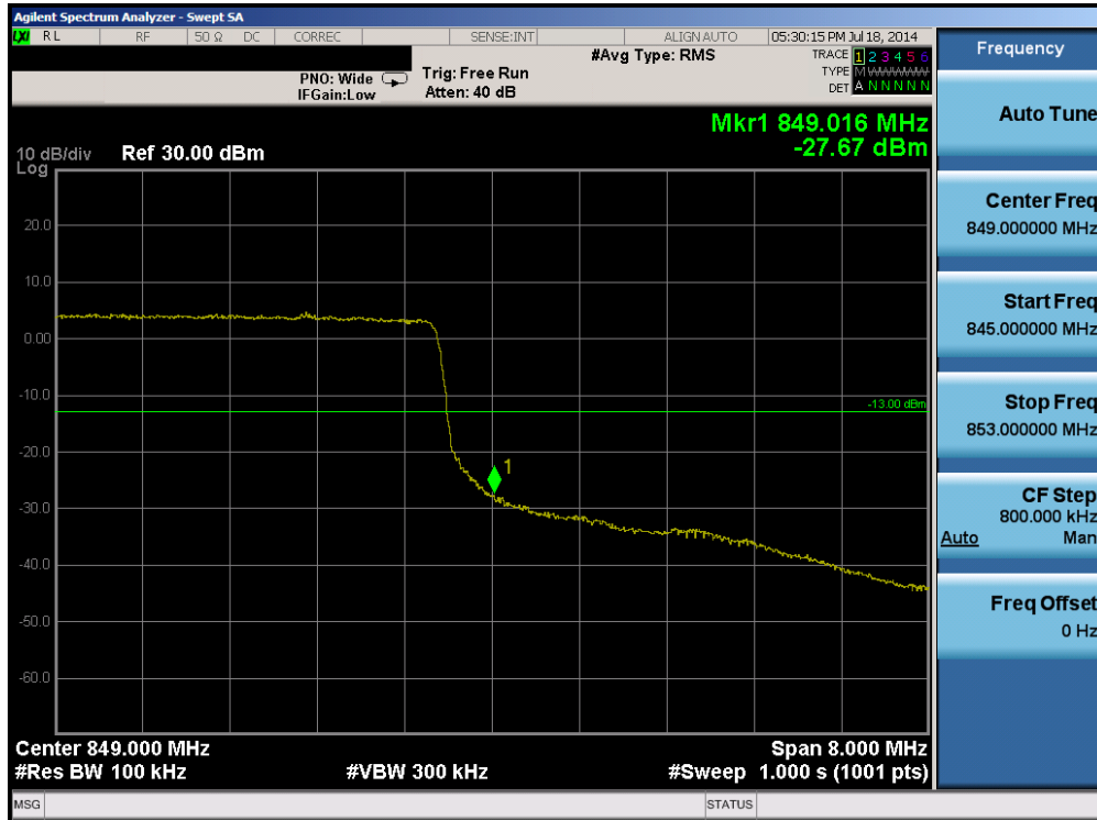
Plot 6-47. Upper Band Edge Plot (Band 5 – 10.0MHz QPSK – RB Size 50)
