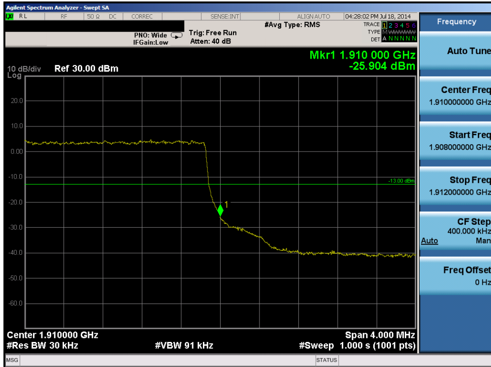
Plot 6-55. Upper Band Edge Plot (Band 2 – 3.0MHz QPSK – RB Size 15)
