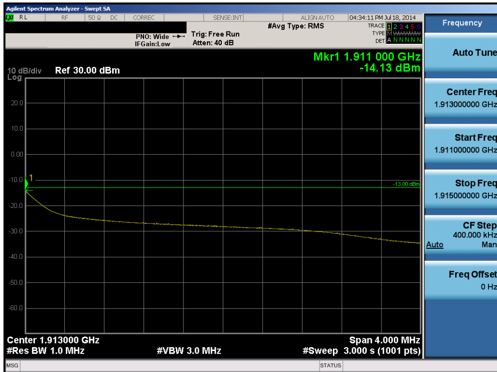
Plot 6-60. Upper Extended Band Edge Plot (Band 2 – 5.0MHz QPSK – RB Size 25)
