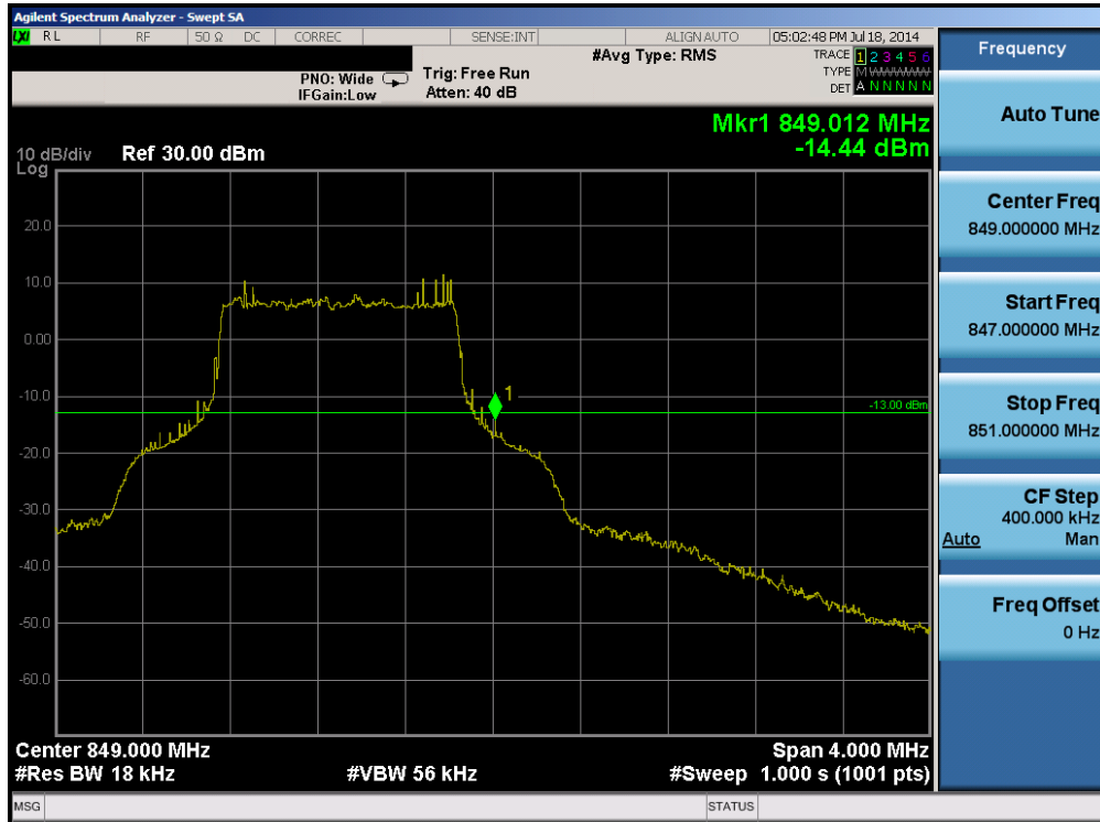
Plot 6-35. Upper Band Edge Plot (Band 5 – 1.4MHz QPSK – RB Size 6)
