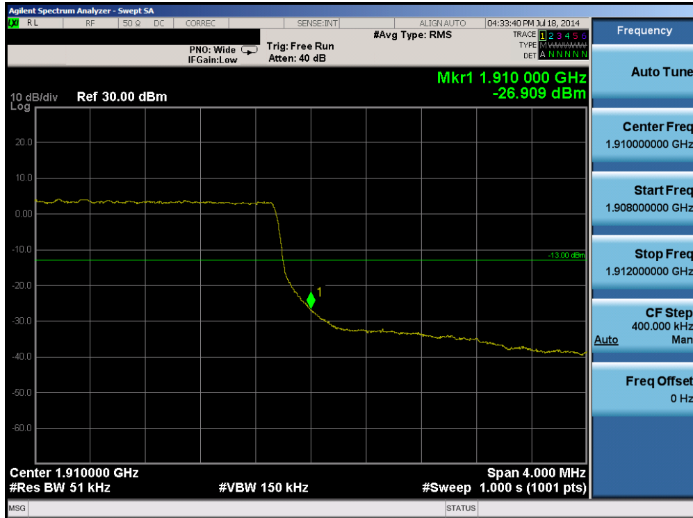
Plot 6-59. Upper Band Edge Plot (Band 2 – 5.0MHz QPSK – RB Size 25)
