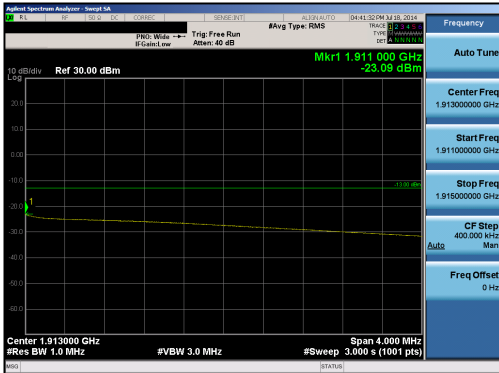
Plot 6-64. Upper Extended Band Edge Plot (Band 2 – 10.0MHz QPSK – RB Size 50)
