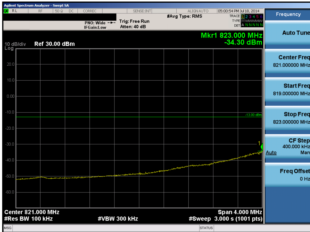
Plot 6-34. Lower Extended Band Edge Plot (Band 5 – 1.4MHz QPSK – RB Size 6)
