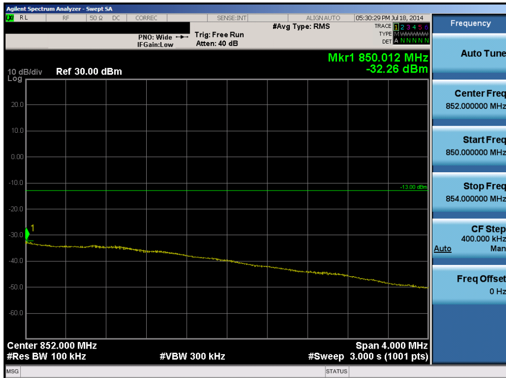
Plot 6-48. Upper Extended Band Edge Plot (Band 5 – 10.0MHz QPSK – RB Size 50)
