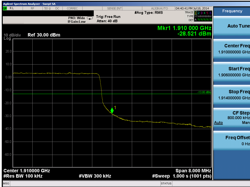
Plot 6-63. Upper Band Edge Plot (Band 2 – 10.0MHz QPSK – RB Size 50)
