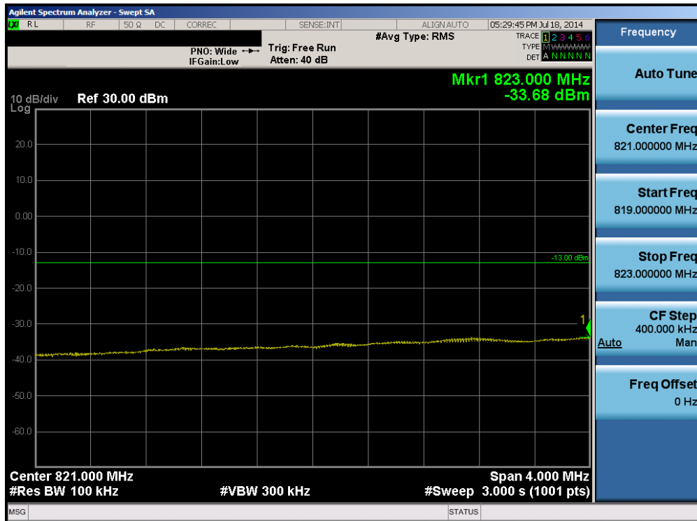
Plot 6-46. Lower Extended Band Edge Plot (Band 5 – 10.0MHz QPSK – RB Size 50)
