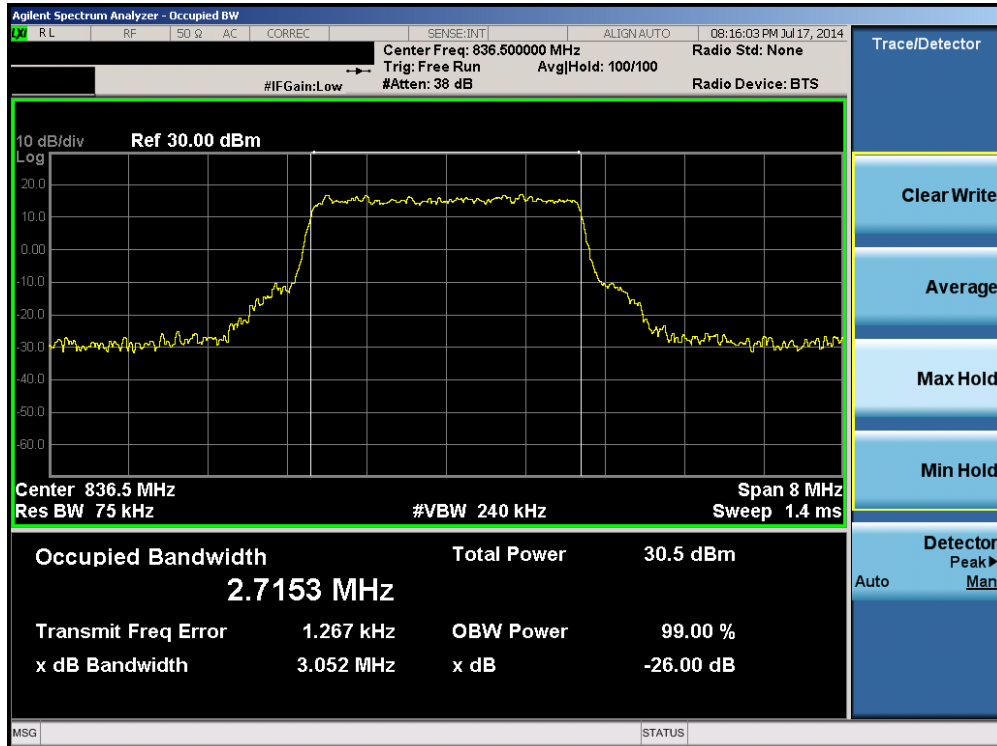
Plot 6-7. Occupied Bandwidth Plot (Band 5 – 3.0MHz QPSK – RB Size 15)
