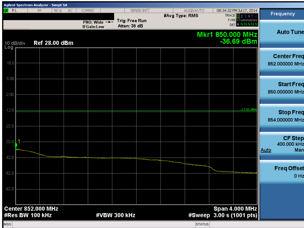
Plot 6-76. Upper Extended Band Edge Plot (Band 5 – 5.0MHz QPSK – RB Size 25)
