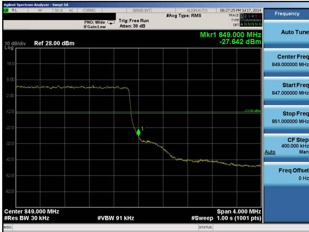
Plot 6-71. Upper Band Edge Plot (Band 5 – 3.0MHz QPSK – RB Size 15)
