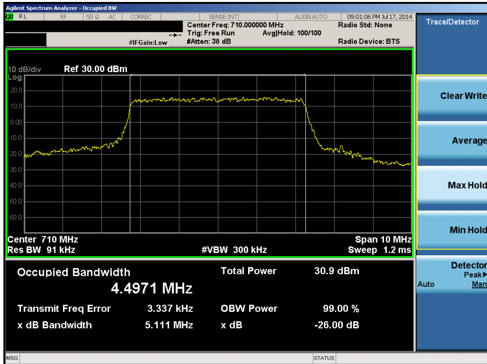
Plot 6-2. Occupied Bandwidth Plot (Band 17 – 5.0MHz 16-QAM – RB Size 25)
