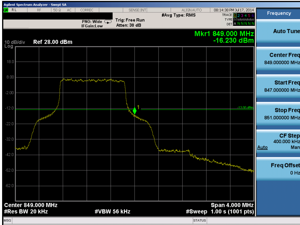
Plot 6-67. Upper Band Edge Plot (Band 5 – 1.4MHz QPSK – RB Size 6)
