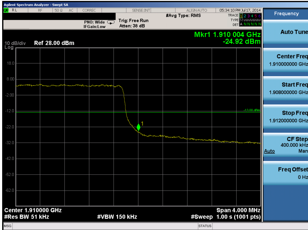
Plot 6-113. Upper Band Edge Plot (Band 2 – 5.0MHz QPSK – RB Size 25)
