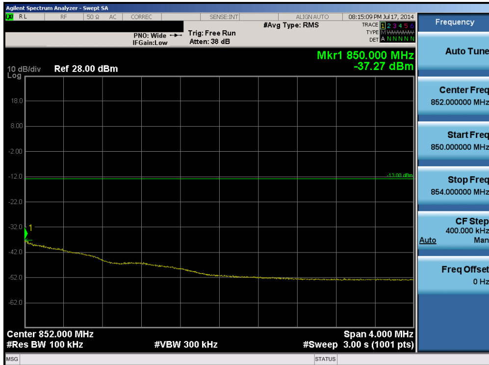
Plot 6-68. Upper Extended Band Edge Plot (Band 5 – 1.4MHz QPSK – RB Size 6)
