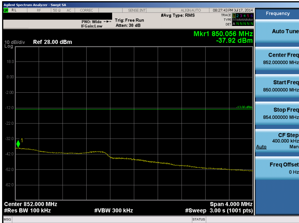
Plot 6-72. Upper Extended Band Edge Plot (Band 5 – Band 5 – 3.0MHz QPSK – RB Size 15)
