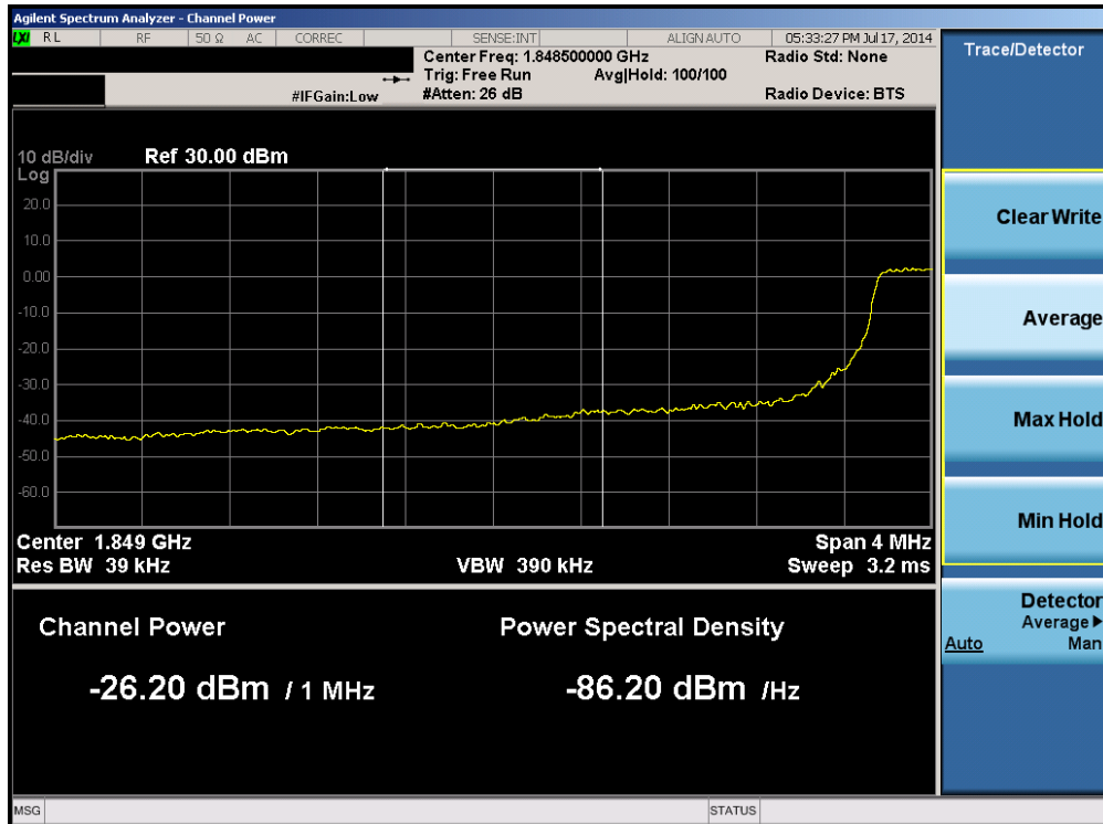
Plot 6-112. Lower Extended Band Edge Plot (Band 2 – 5.0MHz QPSK – RB Size 25)
