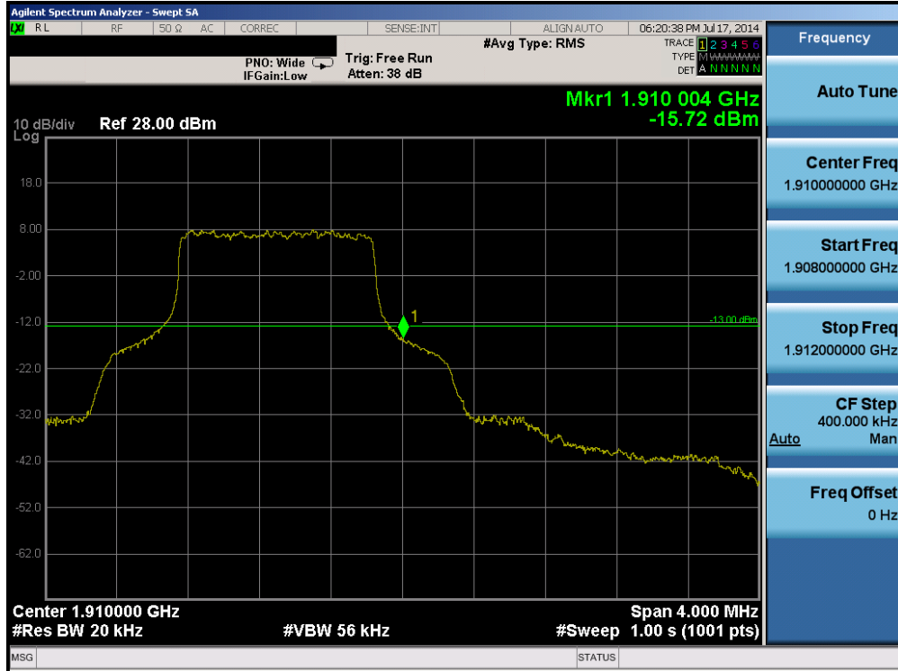
Plot 6-105. Upper Band Edge Plot (Band 2 – 1.4MHz QPSK – RB Size 6)
