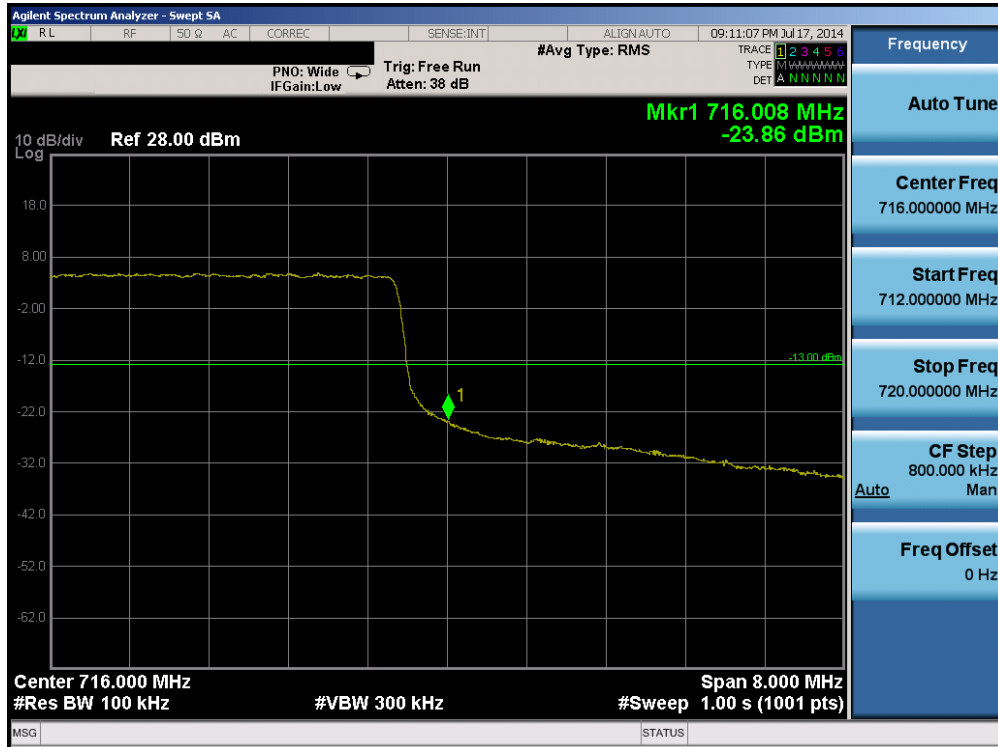
Plot 6-64. Upper Band Edge Plot (Band 17 – 10.0MHz QPSK – RB Size 50)
