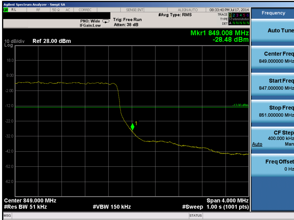
Plot 6-75. Upper Band Edge Plot (Band 5 – 5.0MHz QPSK – RB Size 25)
