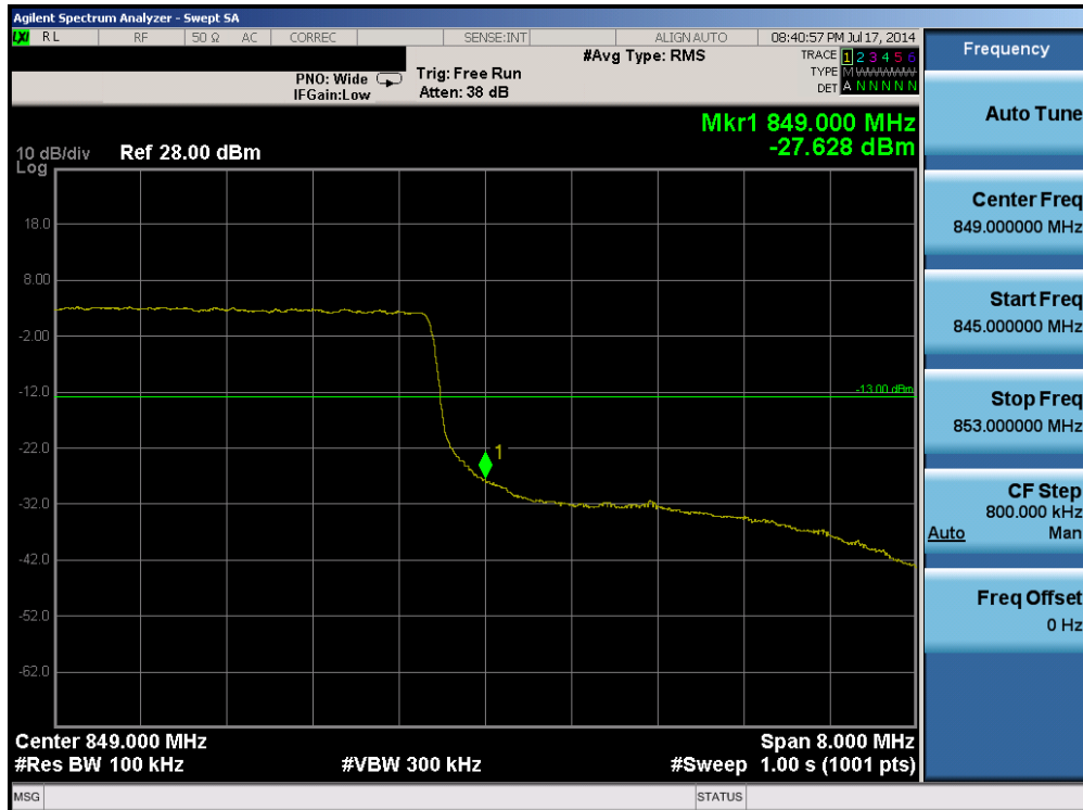
Plot 6-78. Upper Band Edge Plot (Band 5 – 10.0MHz QPSK – RB Size 50)
