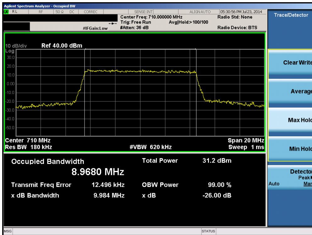
Plot 6-4. Occupied Bandwidth Plot (Band 17 – 10.0MHz 16-QAM – RB Size 50)
