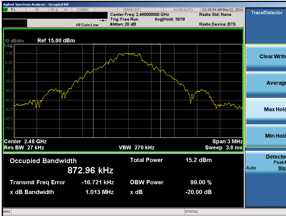
Plot 6-3. 20dB Bandwidth Plot (Bluetooth, 1Mbps – Ch. 78)
