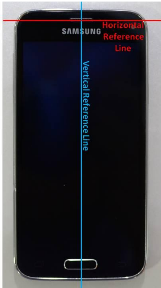
SAR Test Setup Photo 11 – DUT Reference Lines
