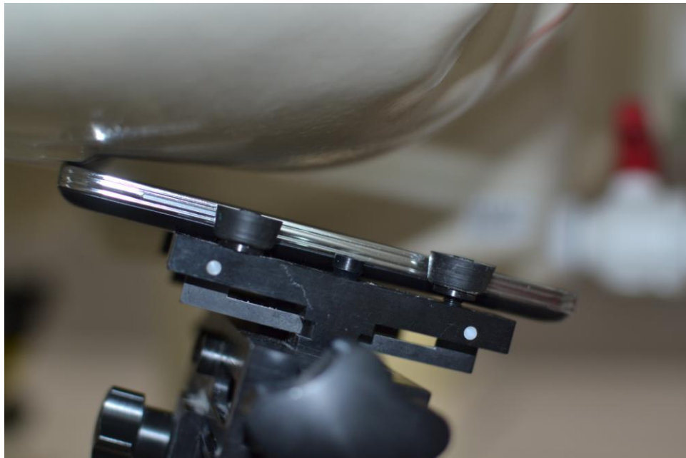
SAR Test Setup Photo 2 – Right Tilt
