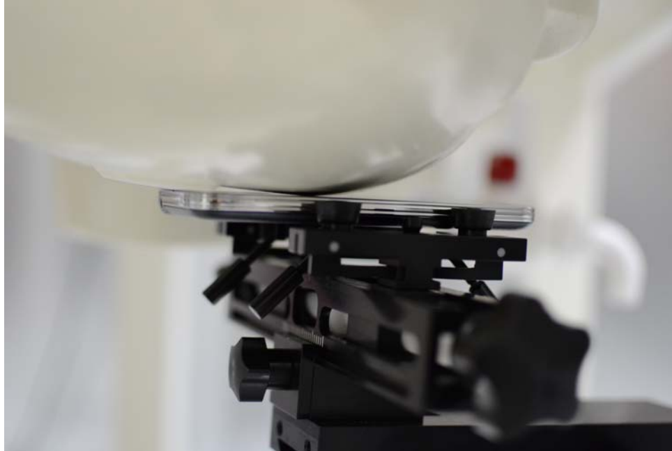
SAR Test Setup Photo 1 – Right Cheek
