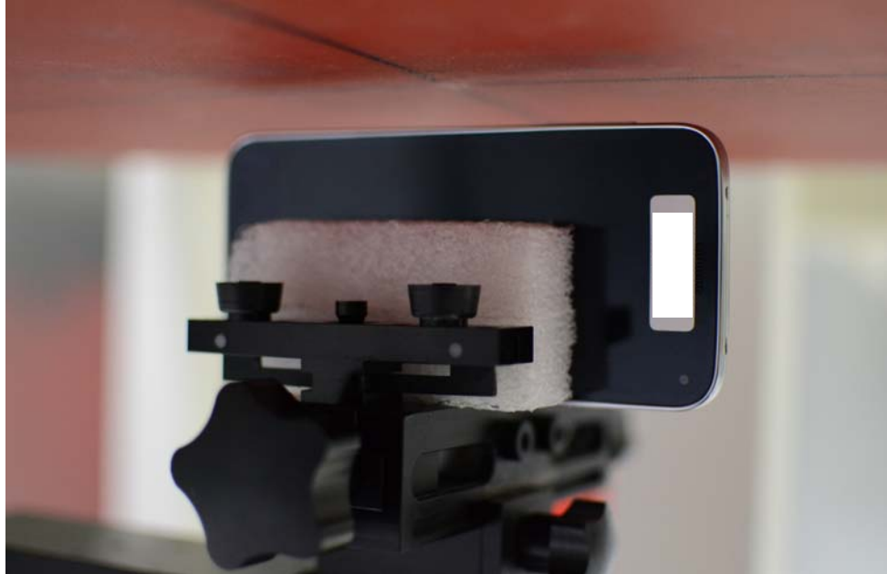
SAR Test Setup Photo 10 – Left Edge at 10 mm
