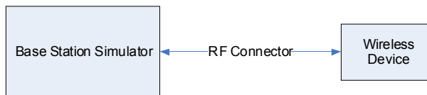
Figure 9-1 Power Measurement Setup
