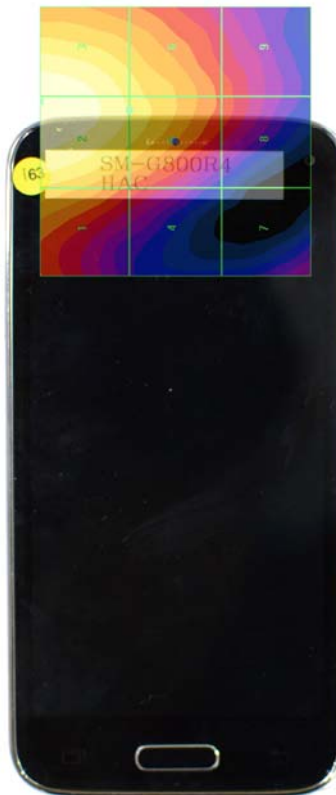
Figure 18-4 E-Field WD Scan overlay
