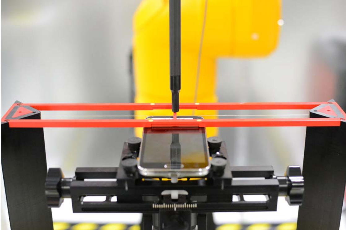
Figure 18-1 Ear Reference Point HAC Phantom Alignment
