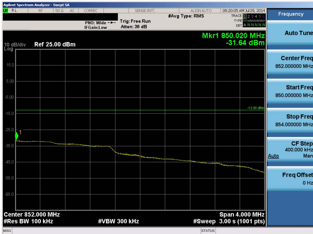
Plot 6-183. Upper Extended Band Edge Plot (Band 5 – Band 5 – 3.0MHz QPSK – RB Size 15)
