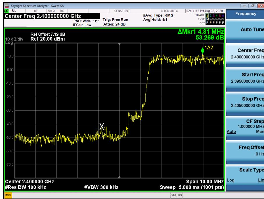
Test Plots with hopping (8DPSK)
