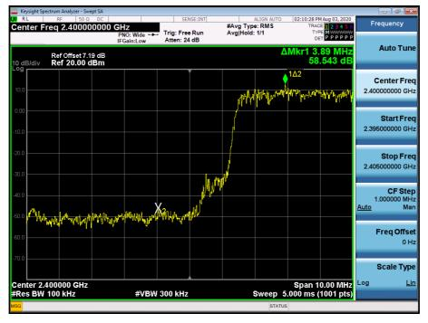
Test Plots with hopping ( $\pi$ /4DQPSK) Band Edges (CH.78)
