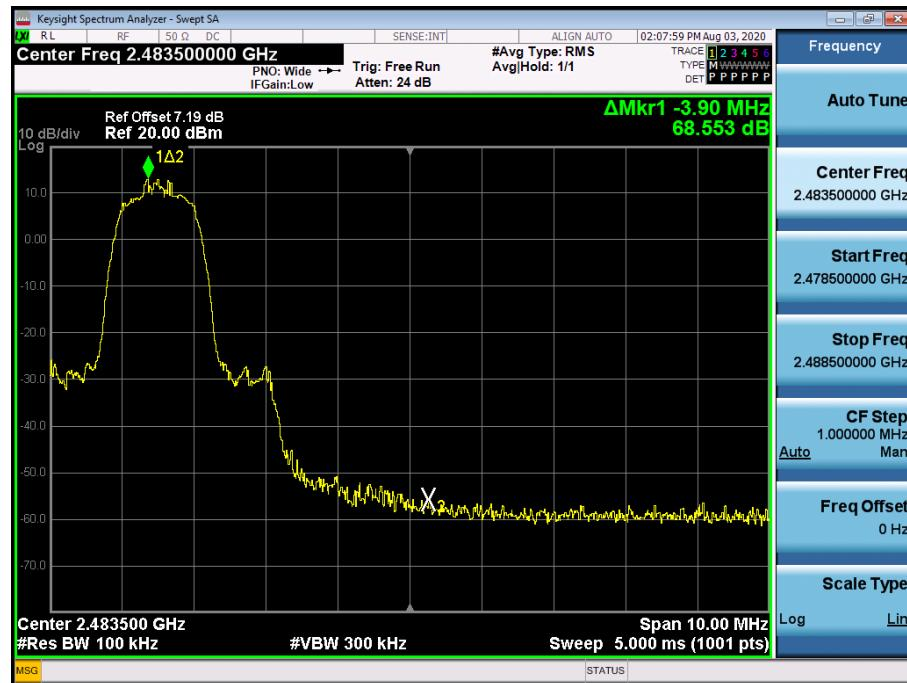
Test Plots with hopping (GFSK)
