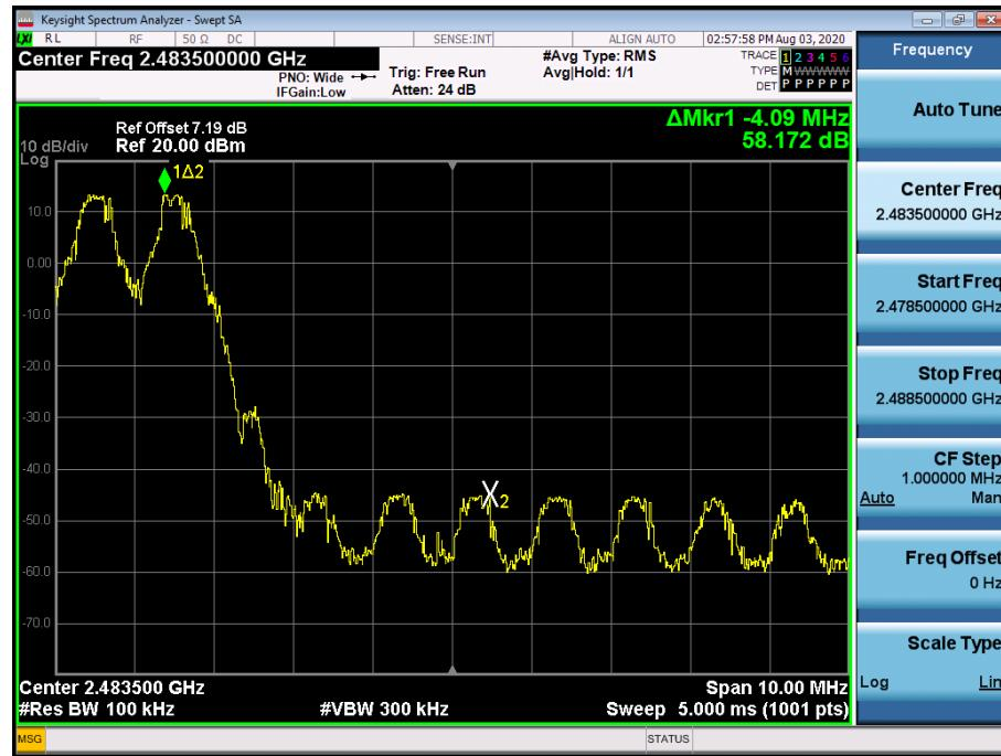
Test Plots with hopping (8DPSK)
