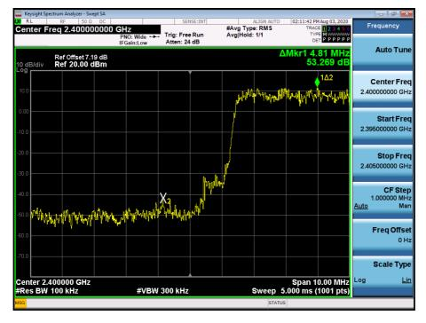
Test Plots with hopping (8DPSK) Band Edges (CH.78)
