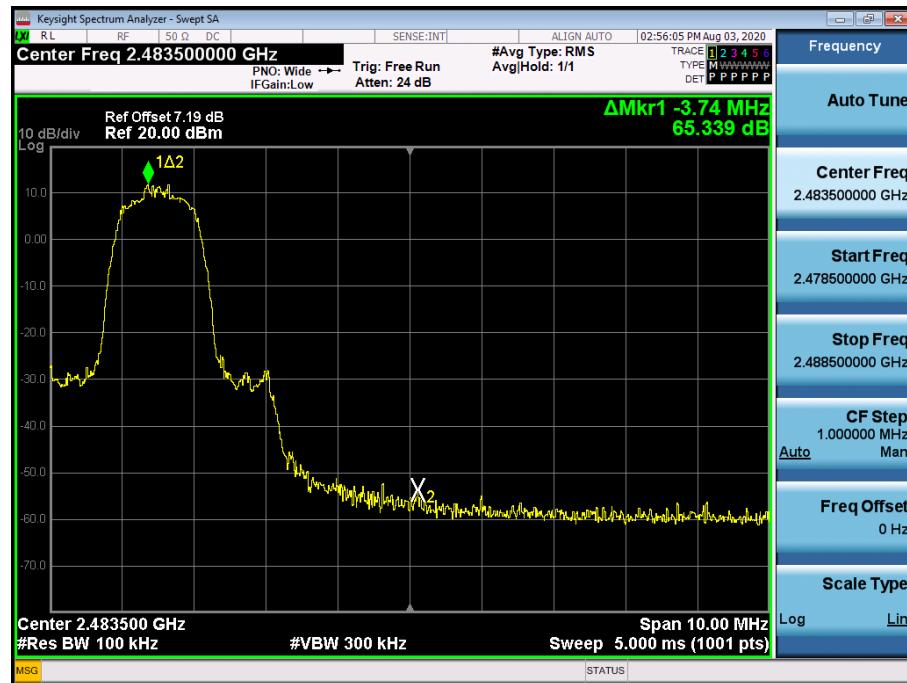
Test Plots with hopping (GFSK)
