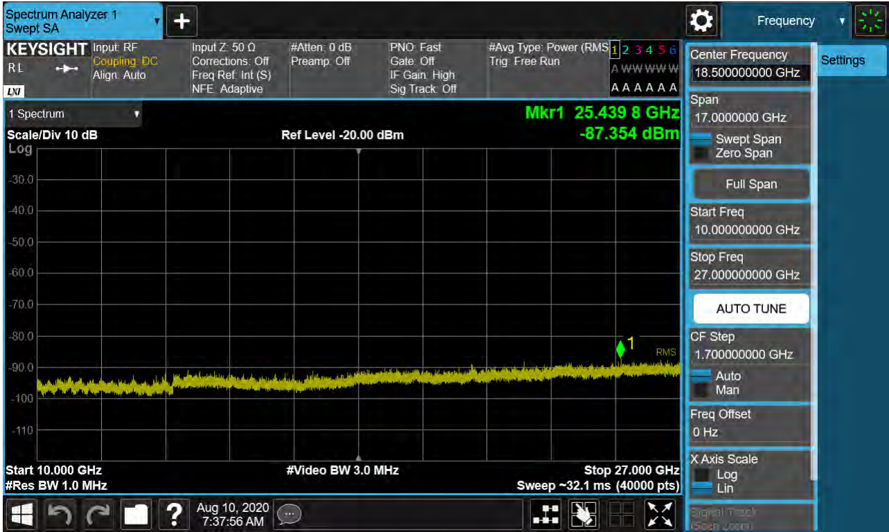
Sub6 n41. Conducted Spurious Plot 2 (40 MHz Ch. 518598 BPSK RB 1, Offset 0)
