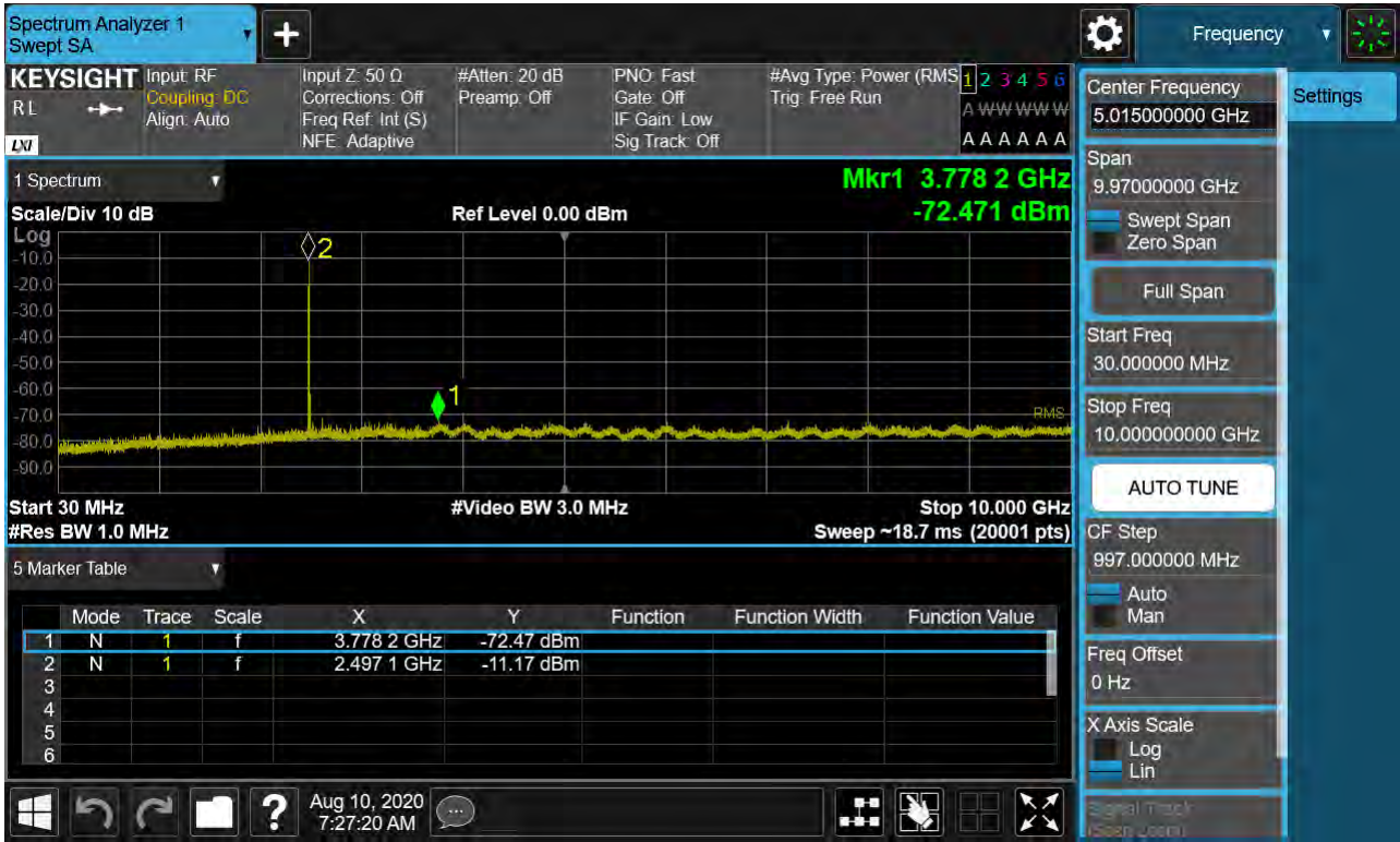
Sub6 n41. Conducted Spurious Plot 1 (40 MHz Ch.503202 BPSK RB 1, Offset 0)
