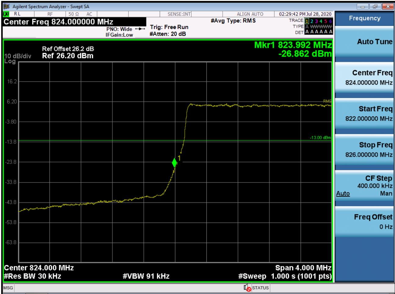
BAND5/ 26. Lower Extended Band Edge Plot (3M BW Ch.26805 QPSK\_RB15\_0)
