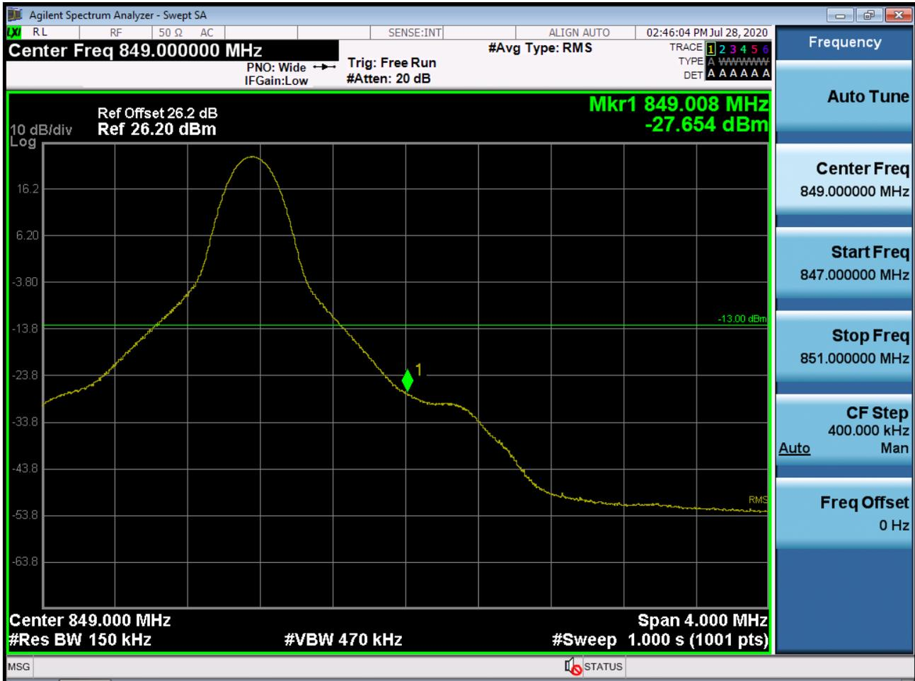
BAND 26. Upper Extended Band Edge Plot (15M BW Ch.26965 QPSK\_RB75\_0) -3
