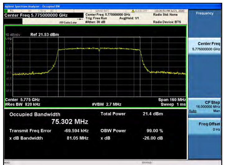
802.11ac_VHT80 UNII 3 BAND 26dB Bandwidth (CH 155)
