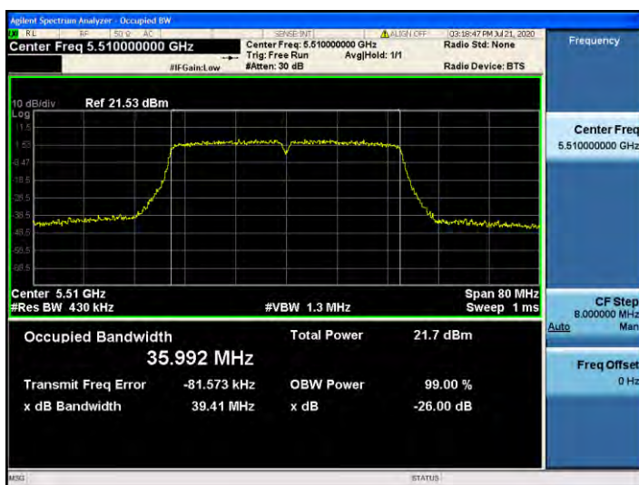
802.11n_HT40 UNII 2C BAND 26dB Bandwidth(CH 102)
