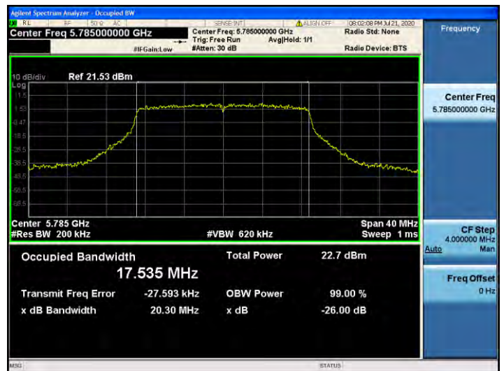
802.11n_HT20 UNII 3 BAND 26dB Bandwidth(CH 157)
