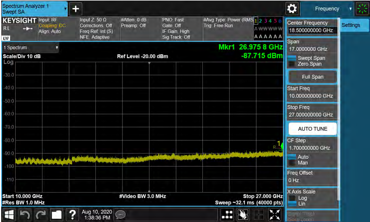
Sub6 n41. Conducted Spurious Plot 2 (100 MHz Ch.528000 BPSK RB 1, Offset 0)
