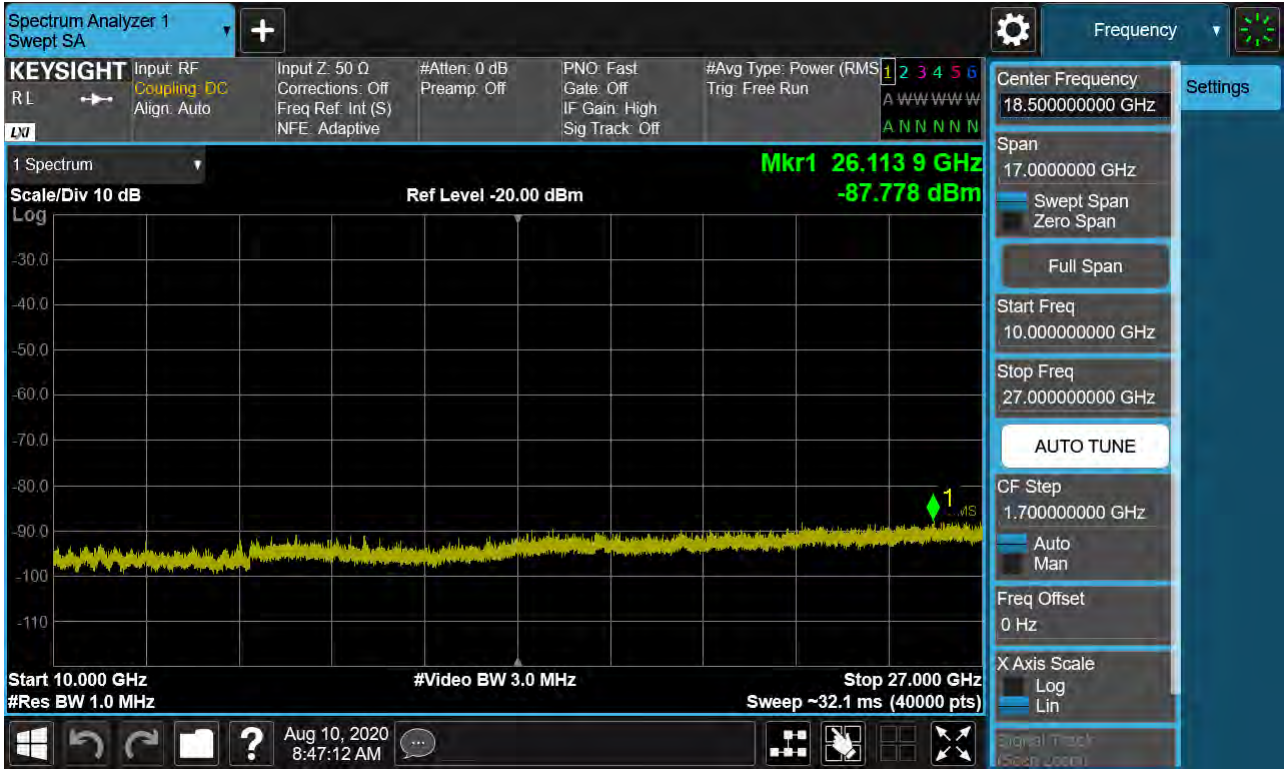
Sub6 n41. Conducted Spurious Plot 2 (60 MHz Ch. 518598 BPSK RB 1, Offset 0)
