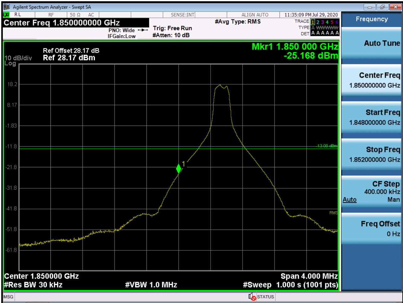
Sub6 n25(2). Lower Band Edge Plot (20M BW Ch.372000 BPSK_RB1_Offset 0)
