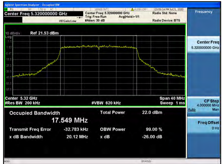
802.11n_HT20 UNII 3 BAND 26dB Bandwidth(CH 157)
