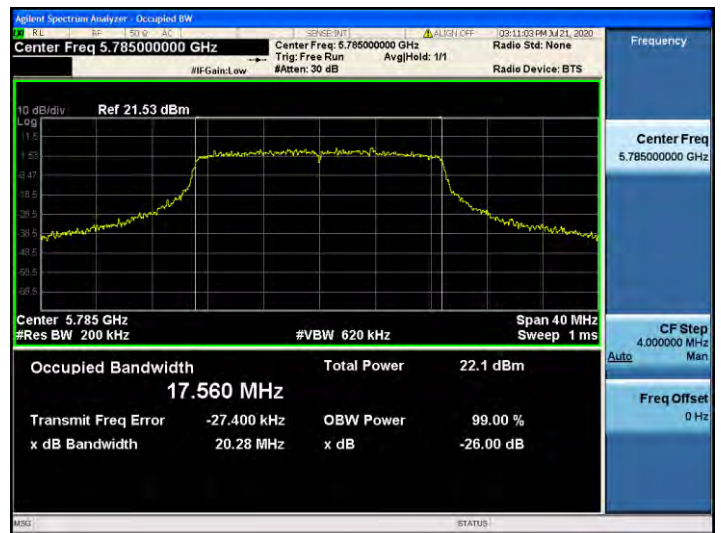
802.11n_HT20 UNII 3 BAND 26dB Bandwidth(CH 157)
