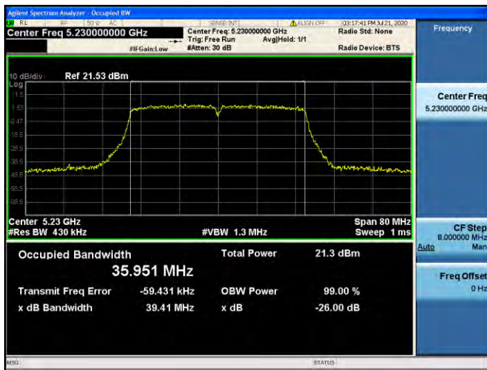
802.11n_HT40 UNII 2C BAND 26dB Bandwidth(CH 102)
