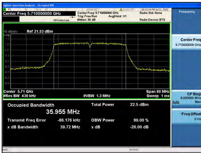
802.11n_HT40 UNII 2C BAND 26dB Bandwidth(CH 142)
