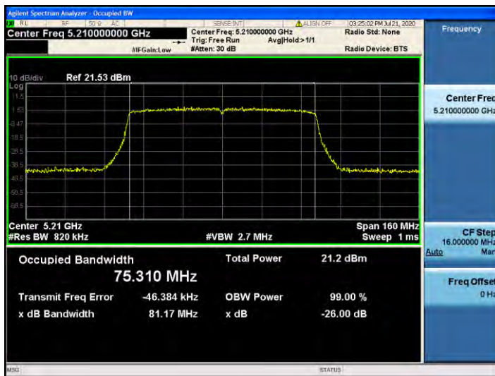
802.11ac_VHT80 UNII 2C BAND 26dB Bandwidth(CH 138)
