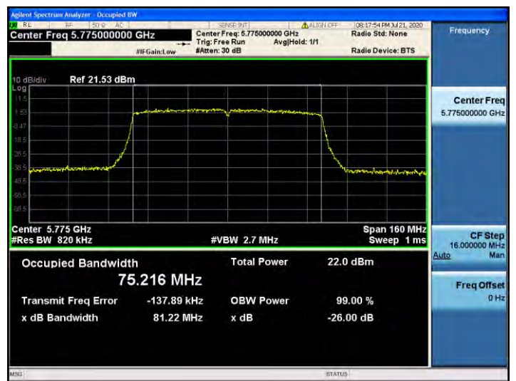
802.11ac_VHT80 UNII 3 BAND 26dB Bandwidth (CH 155)
