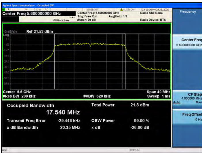
802.11ac_VHT20 UNII 2C BAND 26dB Bandwidth(CH 120)
