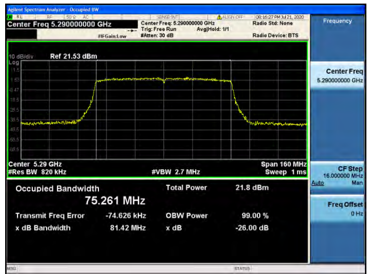
802.11ac_VHT80 UNII 3 BAND 26dB Bandwidth (CH 155)
