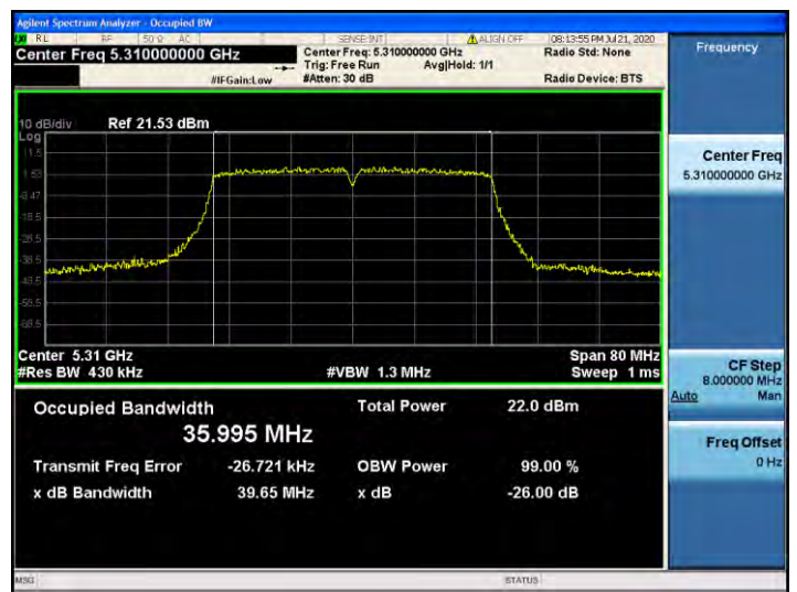
802.11ac_VHT40 UNII 3 BAND 26dB Bandwidth (CH 159)
