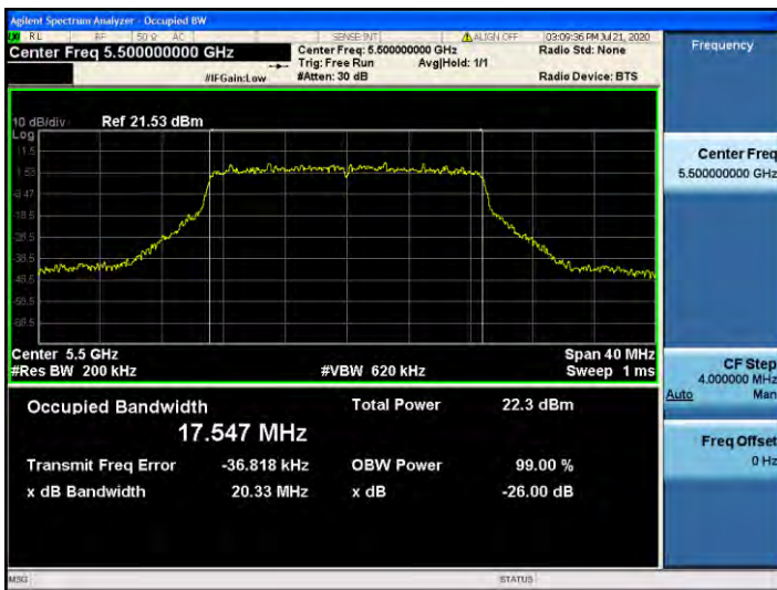
802.11n_HT20 UNII 2C BAND 26dB Bandwidth(CH 100)
