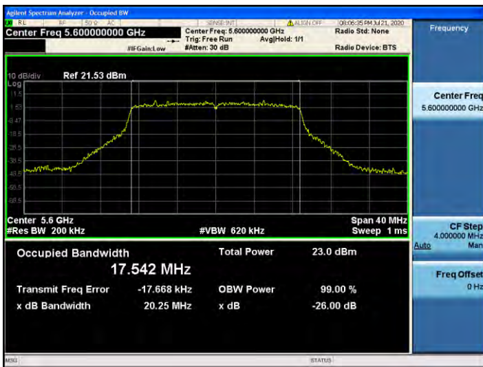
802.11ac_VHT20 UNII 2C BAND 26dB Bandwidth(CH 120)
