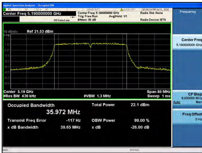
802.11n_HT40 UNII 2C BAND 26dB Bandwidth(CH 142)
