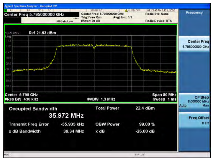
802.11ac_VHT40 UNII 3 BAND 26dB Bandwidth (CH 159)
