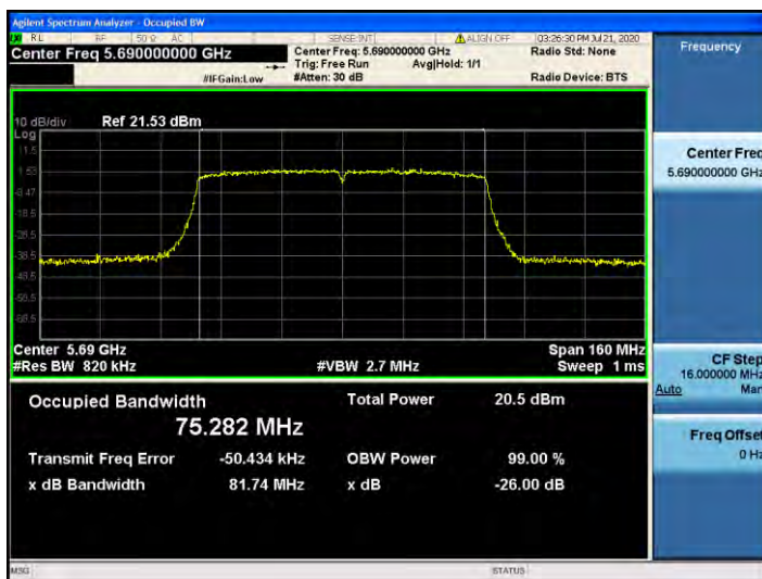
802.11ac_VHT80 UNII 2C BAND 26dB Bandwidth(CH 138)
