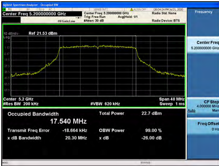
802.11ac_VHT20 UNII 2C BAND 26dB Bandwidth(CH 120)
