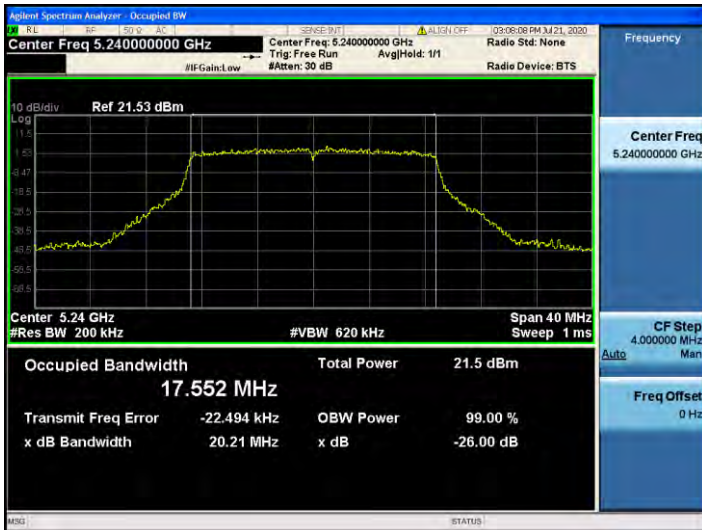
802.11n_HT20 UNII 2C BAND 26dB Bandwidth(CH 100)
