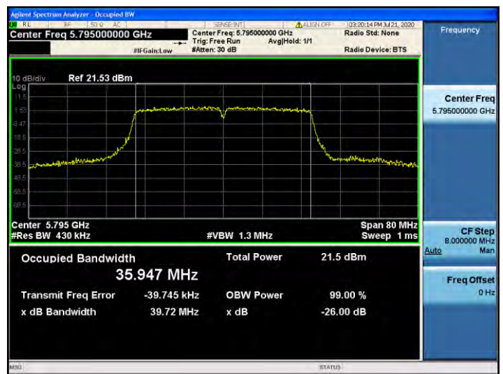
802.11n_HT40 UNII 3 BAND 26dB Bandwidth (CH 159)
