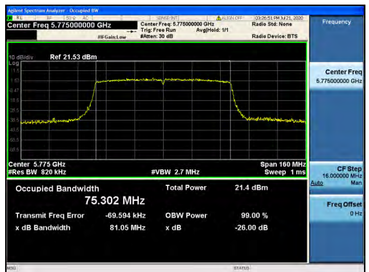
802.11ac_VHT80 UNII 3 BAND 26dB Bandwidth (CH 155)
