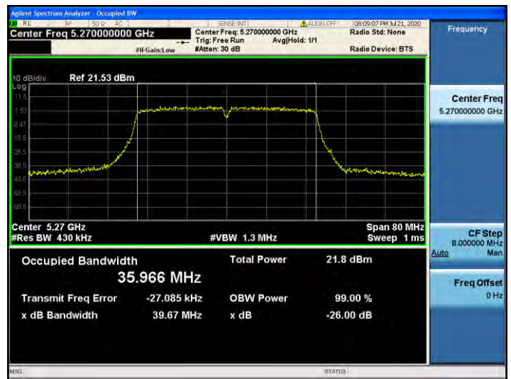
802.11n_HT40 UNII 3 BAND 26dB Bandwidth (CH 159)
