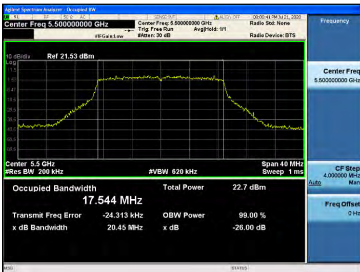
802.11n_HT20 UNII 2C BAND 26dB Bandwidth(CH 100)
