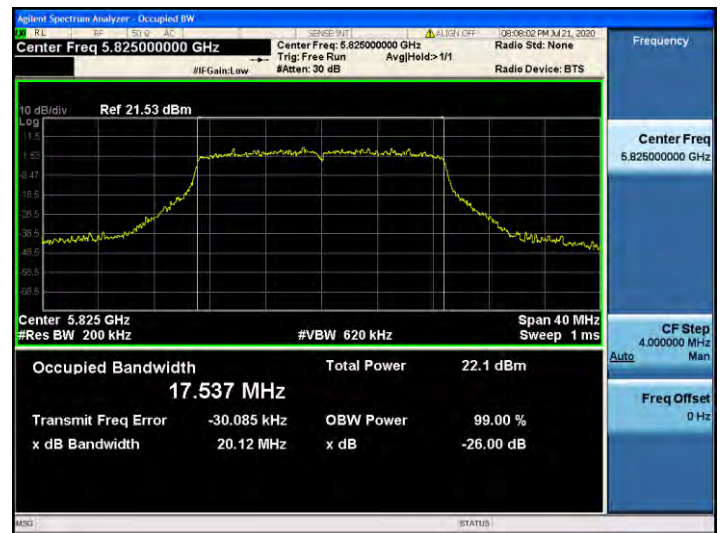
802.11ac_VHT20 UNII 3 BAND 26dB Bandwidth(CH 165)
