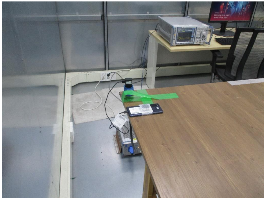
AC LINE CONDUCTED REAR TEST PHOTO(WPT)
