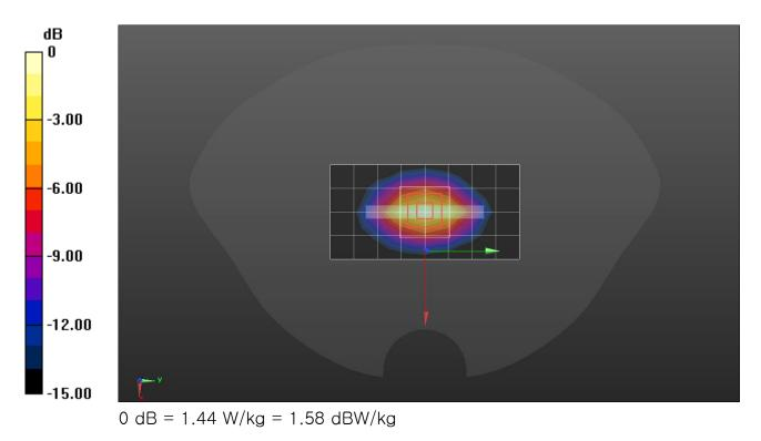
Frequency: 1852.4 MHz; Duty Cycle: 1:1; Room Ambient Temperature: 23.0°C; Liquid Temperature: 22.0°C Medium parameters used (interpolated): f = 1852.4 MHz;  $\sigma$  = 1.396 S/m;  $\epsilon_r$  = 39.657;  $\rho$  = 1000 kg/m<sup>3</sup> DASY5 Configuration:
