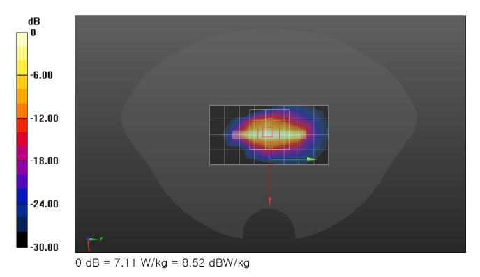
Frequency: 1732.6 MHz; Duty Cycle: 1:1; Room Ambient Temperature: 23.0°C; Liquid Temperature: 22.0°C Medium parameters used (interpolated): f = 1732.6 MHz;  $\sigma$  = 1.329 S/m;  $\epsilon_r$  = 40.082;  $\rho$  = 1000 kg/m<sup>3</sup> DASY5 Configuration:
