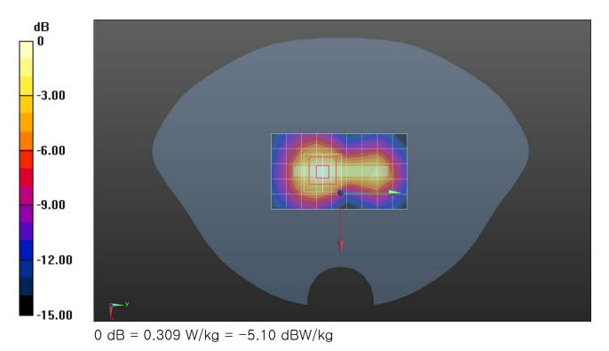
Frequency: 1770 MHz; Duty Cycle: 1:1; Room Ambient Temperature: 23.0°C; Liquid Temperature: 22.0°C Medium parameters used: f = 1770 MHz;  $\sigma$  = 1.36 S/m;  $\epsilon_r$  = 40.558;  $\rho$  = 1000 kg/m<sup>3</sup> DASY5 Configuration:
