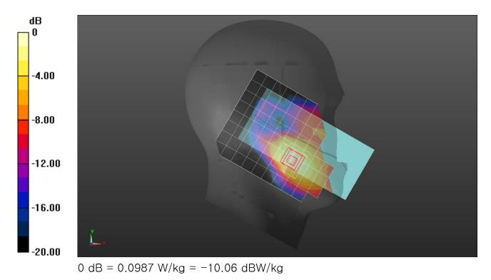
Frequency: 1880 MHz; Duty Cycle: 1:2.60016; Room Ambient Temperature: 23.0°C; Liquid Temperature: 22.0°C Medium parameters used: f = 1880 MHz;  $\sigma$  = 1.402 S/m;  $\epsilon_r$  = 39.331;  $\rho$  = 1000 kg/m<sup>3</sup> DASY5 Configuration:
