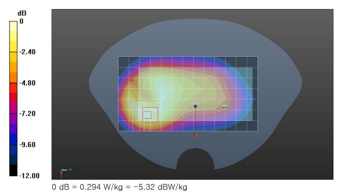
Frequency: 836.6 MHz; Duty Cycle: 1:2.60016; Room Ambient Temperature: 23.0°C; Liquid Temperature: 22.0°C Medium parameters used (interpolated): f = 836.6 MHz;  $\sigma$  = 0.937 S/m;  $\epsilon_r$  = 40.736;  $\rho$  = 1000 kg/m<sup>3</sup> DASY5 Configuration:
