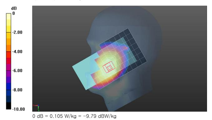
Frequency: 707.5 MHz; Duty Cycle: 1:1; Room Ambient Temperature: 23.0°C; Liquid Temperature: 22.0°C Medium parameters used (interpolated): f = 707.5 MHz;  $\sigma$  = 0.883 S/m;  $\epsilon_r$  = 42.277;  $\rho$  = 1000 kg/m<sup>3</sup> DASY5 Configuration:
