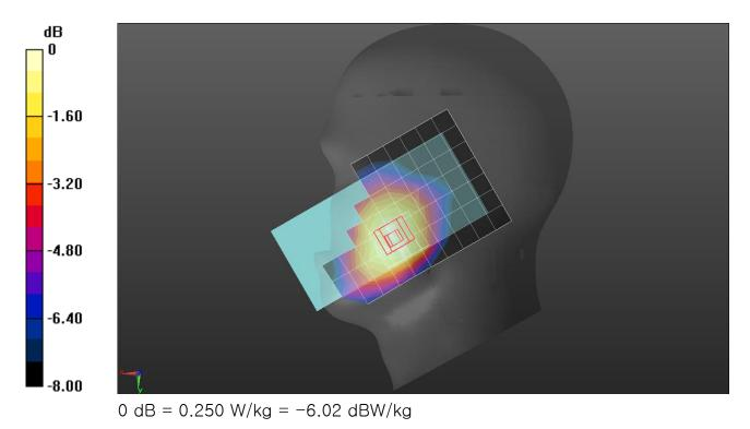
Frequency: 836.5 MHz; Duty Cycle: 1:1; Room Ambient Temperature: 23.0°C; Liquid Temperature: 22.0°C Medium parameters used (interpolated): f = 836.5 MHz;  $\sigma$  = 0.93 S/m;  $\epsilon_r$  = 40.583;  $\rho$  = 1000 kg/m<sup>3</sup> DASY5 Configuration:
