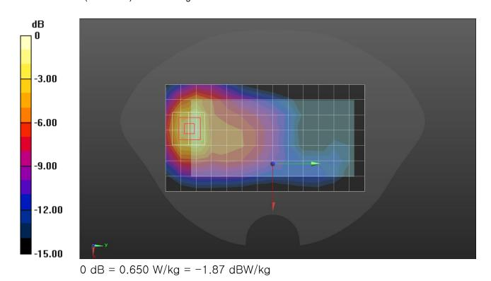
Frequency: 1770 MHz; Duty Cycle: 1:1; Room Ambient Temperature: 23.0°C; Liquid Temperature: 22.0°C Medium parameters used: f = 1770 MHz;  $\sigma$  = 1.345 S/m;  $\epsilon_r$  = 39.658;  $\rho$  = 1000 kg/m<sup>3</sup> DASY5 Configuration:
