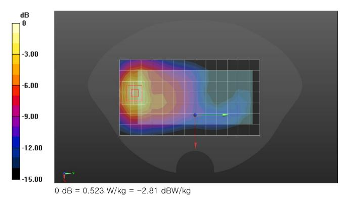
Frequency: 1752.6 MHz; Duty Cycle: 1:1; Room Ambient Temperature: 23.0°C; Liquid Temperature: 22.0°C Medium parameters used (interpolated): f = 1752.6 MHz;  $\sigma$  = 1.34 S/m;  $\epsilon_r$  = 40.001;  $\rho$  = 1000 kg/m<sup>3</sup> DASY5 Configuration:
