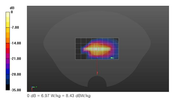
Frequency: 836.5 MHz; Duty Cycle: 1:1; Room Ambient Temperature: 23.0°C; Liquid Temperature: 22.0°C Medium parameters used (interpolated): f = 836.5 MHz;  $\sigma$  = 0.929 S/m;  $\epsilon_r$  = 42.233;  $\rho$  = 1000 kg/m<sup>3</sup> DASY5 Configuration:
