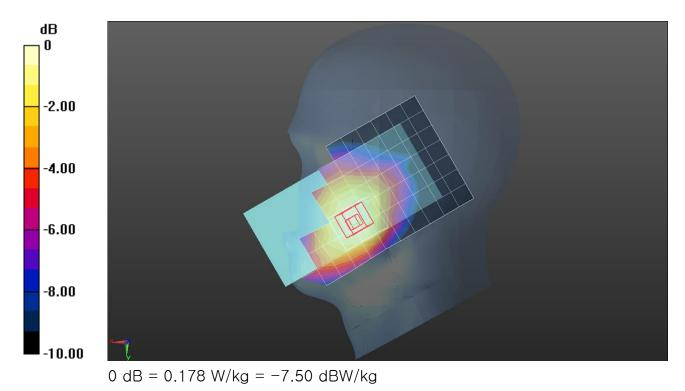
Frequency: 836.6 MHz; Duty Cycle: 1:2.60016; Room Ambient Temperature: 23.0°C; Liquid Temperature: 22.0°C Medium parameters used (interpolated): f = 836.6 MHz;  $\sigma$  = 0.929 S/m;  $\epsilon_r$  = 41.354;  $\rho$  = 1000 kg/m<sup>3</sup> DASY5 Configuration:
