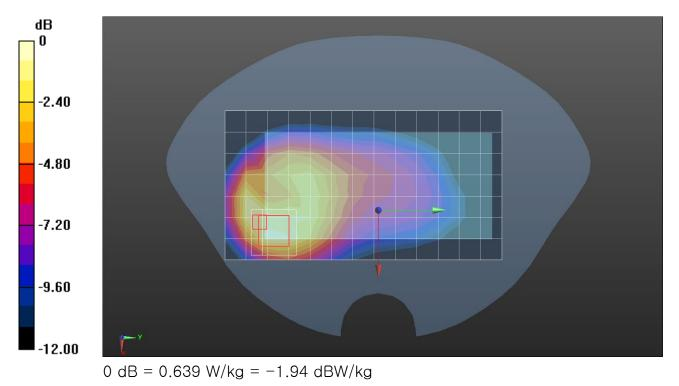
Frequency: 2593 MHz; Duty Cycle: 1:1.59956; Room Ambient Temperature: 23.0°C; Liquid Temperature: 22.0°C Medium parameters used (interpolated): f = 2593 MHz;  $\sigma$  = 1.899 S/m;  $\epsilon_r$  = 40.096;  $\rho$  = 1000 kg/m<sup>3</sup> DASY5 Configuration:
