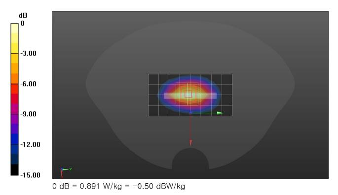
Frequency: 1770 MHz; Duty Cycle: 1:1; Room Ambient Temperature: 23.0°C; Liquid Temperature: 22.0°C Medium parameters used: f = 1770 MHz;  $\sigma$  = 1.376 S/m;  $\epsilon_r$  = 39.668;  $\rho$  = 1000 kg/m<sup>3</sup> DASY5 Configuration:
