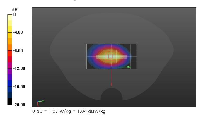
Frequency: 1860 MHz; Duty Cycle: 1:1; Room Ambient Temperature: 23.0°C; Liquid Temperature: 22.0°C Medium parameters used: f = 1860 MHz;  $\sigma$  = 1.425 S/m;  $\epsilon_r$  = 39.577;  $\rho$  = 1000 kg/m<sup>3</sup> DASY5 Configuration:
