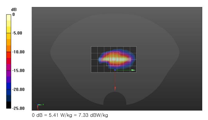
Frequency: 1880 MHz; Duty Cycle: 1:1; Room Ambient Temperature: 23.0°C; Liquid Temperature: 22.0°C Medium parameters used: f = 1880 MHz;  $\sigma$  = 1.414 S/m;  $\epsilon_r$  = 39.579;  $\rho$  = 1000 kg/m<sup>3</sup> DASY5 Configuration:
