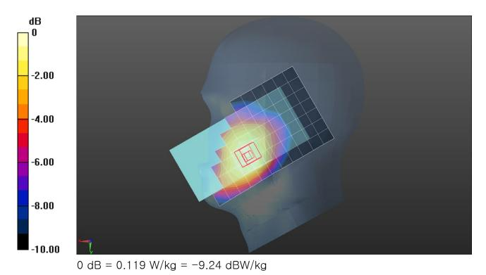
Frequency: 782 MHz; Duty Cycle: 1:1; Room Ambient Temperature: 23.0°C; Liquid Temperature: 22.0°C Medium parameters used (interpolated): f = 782 MHz;  $\sigma$  = 0.91 S/m;  $\epsilon_r$  = 42.005;  $\rho$  = 1000 kg/m<sup>3</sup> DASY5 Configuration:
