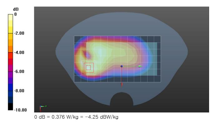
Frequency: 836.6 MHz; Duty Cycle: 1:1; Room Ambient Temperature: 23.0°C; Liquid Temperature: 22.0°C Medium parameters used (interpolated): f = 836.6 MHz;  $\sigma$  = 0.93 S/m;  $\epsilon_r$  = 41.799;  $\rho$  = 1000 kg/m<sup>3</sup> DASY5 Configuration:
