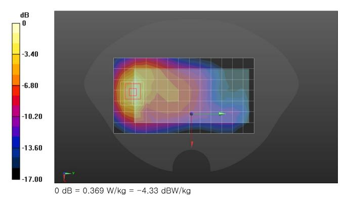
Frequency: 1880 MHz; Duty Cycle: 1:2.60016; Room Ambient Temperature: 23.0°C; Liquid Temperature: 22.0°C Medium parameters used: f = 1880 MHz;  $\sigma$  = 1.387 S/m;  $\epsilon_r$  = 39.18;  $\rho$  = 1000 kg/m<sup>3</sup> DASY5 Configuration:
