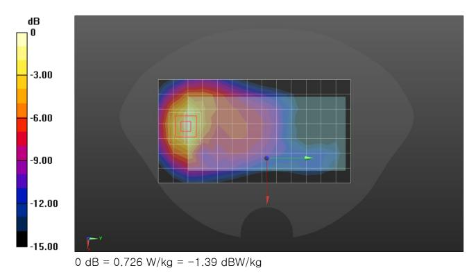
Frequency: 1907.6 MHz; Duty Cycle: 1:1; Room Ambient Temperature: 23.0°C; Liquid Temperature: 22.0°C Medium parameters used (interpolated): f = 1907.6 MHz;  $\sigma$  = 1.397 S/m;  $\epsilon_r$  = 39.014;  $\rho$  = 1000 kg/m<sup>3</sup> DASY5 Configuration:
