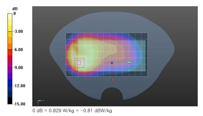
Frequency: 1880 MHz; Duty Cycle: 1:1; Room Ambient Temperature: 23.0°C; Liquid Temperature: 22.0°C Medium parameters used: f = 1880 MHz;  $\sigma$  = 1.402 S/m;  $\epsilon_r$  = 39.331;  $\rho$  = 1000 kg/m<sup>3</sup> DASY5 Configuration:
