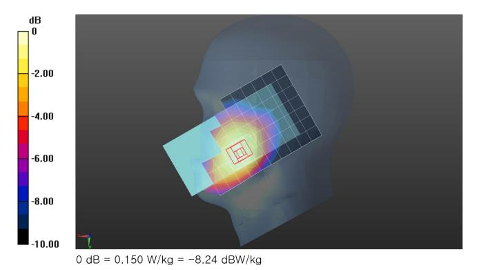
Frequency: 831.5 MHz; Duty Cycle: 1:1; Room Ambient Temperature: 23.0°C; Liquid Temperature: 22.0°C Medium parameters used (interpolated): f = 831.5 MHz;  $\sigma$  = 0.927 S/m;  $\epsilon_r$  = 41.372;  $\rho$  = 1000 kg/m<sup>3</sup> DASY5 Configuration:
