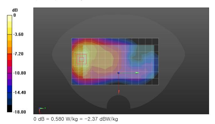
Frequency: 1900 MHz; Duty Cycle: 1:1; Room Ambient Temperature: 23.0°C; Liquid Temperature: 22.0°C Medium parameters used: f = 1900 MHz;  $\sigma$  = 1.394 S/m;  $\epsilon_r$  = 39.059;  $\rho$  = 1000 kg/m<sup>3</sup> DASY5 Configuration:
