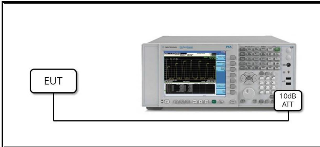
**SETUP DIAGRAM FOR TESTS (RADIATED TEST SETUP)**
