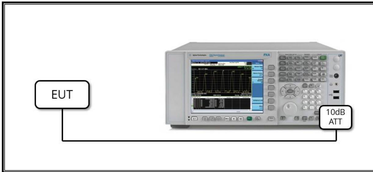
**SETUP DIAGRAM FOR TESTS (RADIATED TEST SETUP)**
