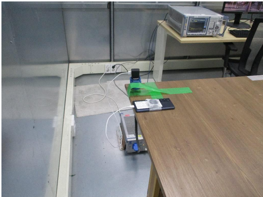
AC LINE CONDUCTED REAR TEST PHOTO(WPT)
