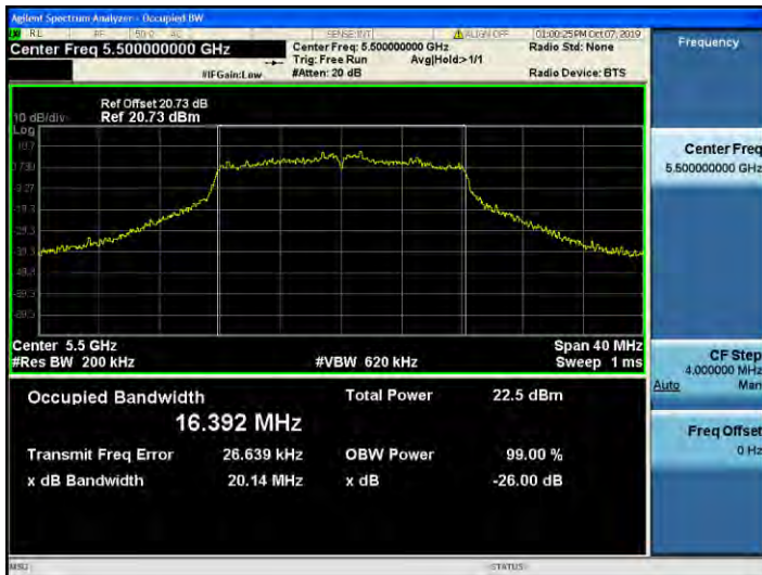
802.11a UNII 2C BAND 26dB Bandwidth (CH 100)
