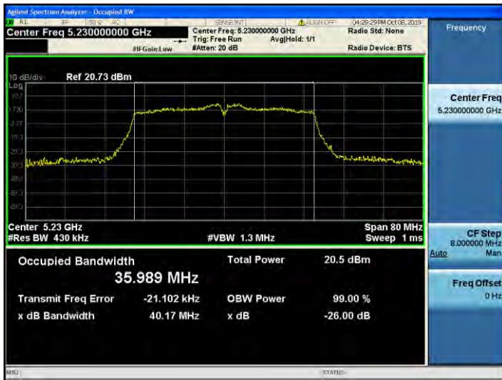
802.11n_HT40 UNII 2C BAND 26dB Bandwidth(CH 142)
