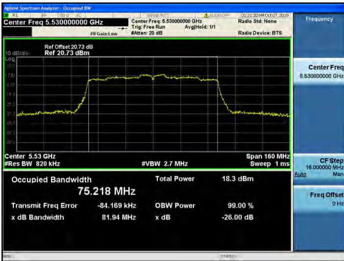
802.11ac_VHT80 UNII 2C BAND 26dB Bandwidth(CH 106)
