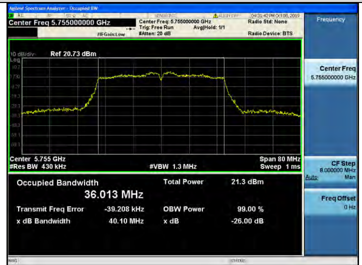
802.11n_HT40 UNII 3 BAND 26dB Bandwidth (CH 151)
