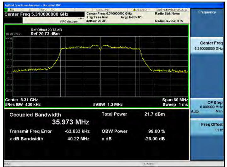
802.11ac_VHT40 UNII 3 BAND 26dB Bandwidth (CH 151)
