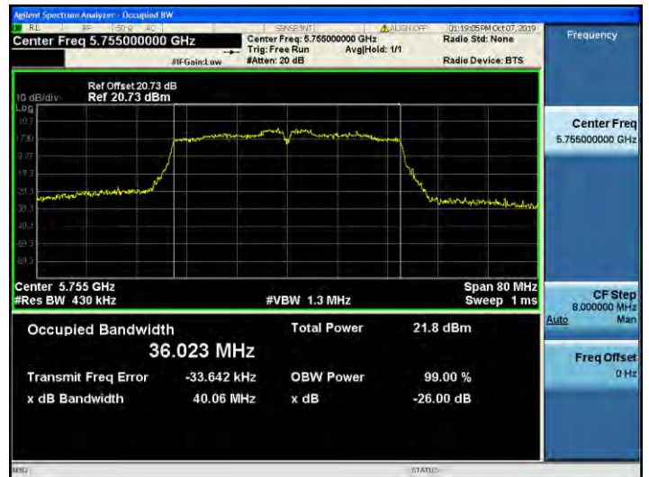
802.11ac_VHT40 UNII 3 BAND 26dB Bandwidth (CH 151)
