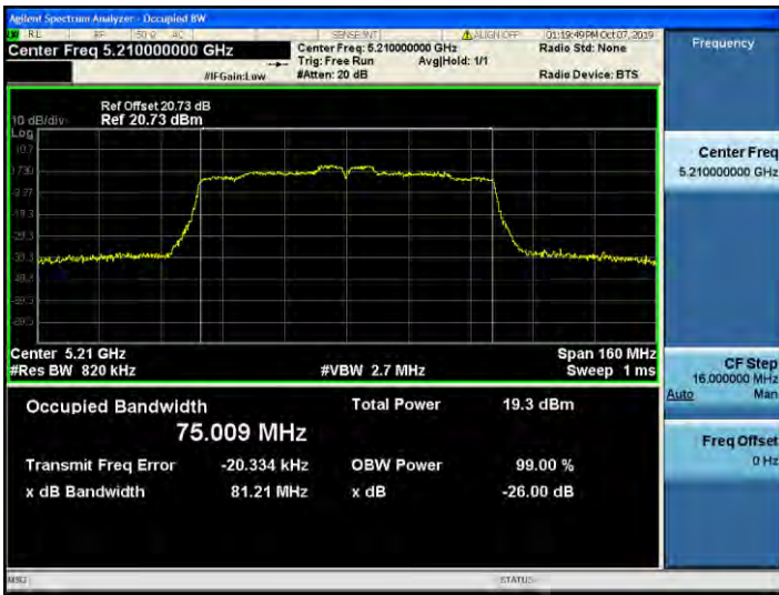
802.11ac_VHT80 UNII 2C BAND 26dB Bandwidth(CH 106)
