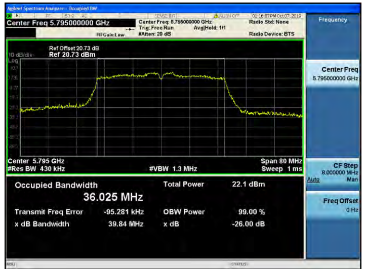
802.11n_HT40 UNII 3 BAND 26dB Bandwidth (CH 159)
