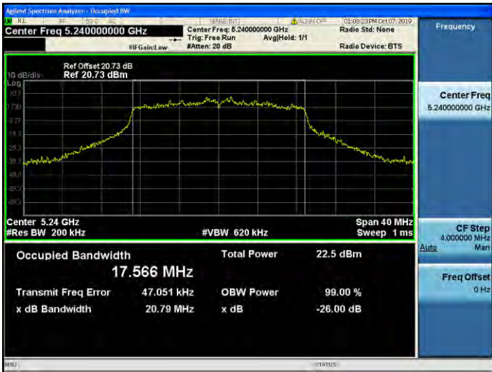
802.11n_HT20 UNII 2C BAND 26dB Bandwidth(CH 144)
