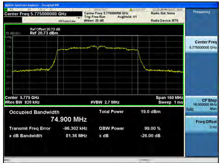
802.11ac_VHT80 UNII 3 BAND 26dB Bandwidth (CH 155)
