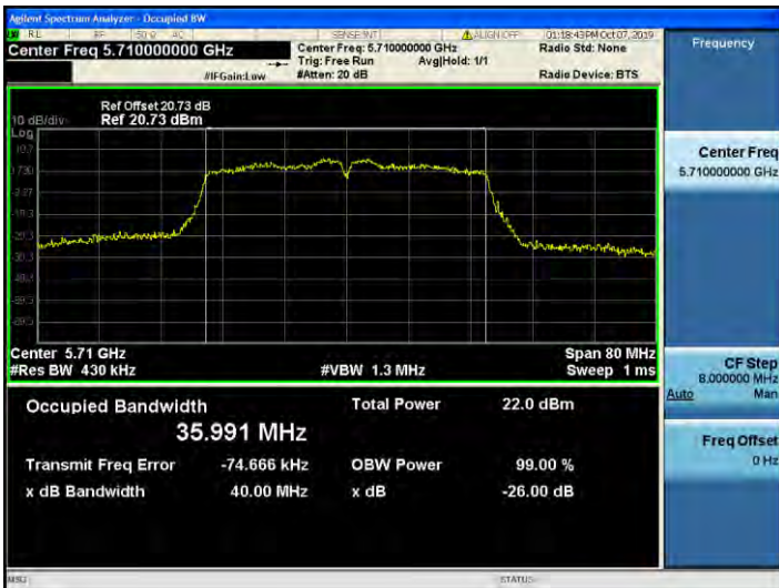
802.11ac_VHT40 UNII 2C BAND 26dB Bandwidth(CH 142)
