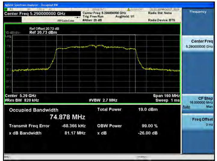
802.11ac_VHT80 UNII 3 BAND 26dB Bandwidth (CH 155)
