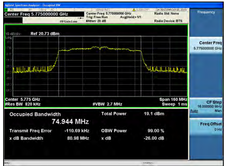
802.11ac_VHT80 UNII 3 BAND 26dB Bandwidth (CH 155)
