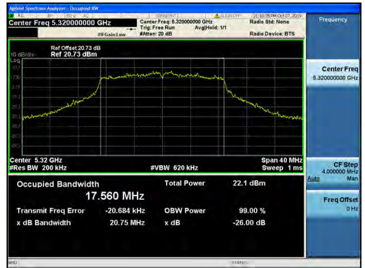
802.11ac_VHT20 UNII 3 BAND 26dB Bandwidth(CH 165)
