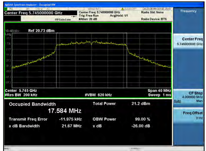
802.11n_HT20 UNII 3 BAND 26dB Bandwidth(CH 149)
