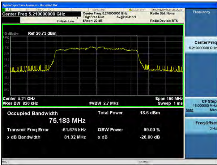
802.11ac_VHT80 UNII 2C BAND 26dB Bandwidth(CH 106)
