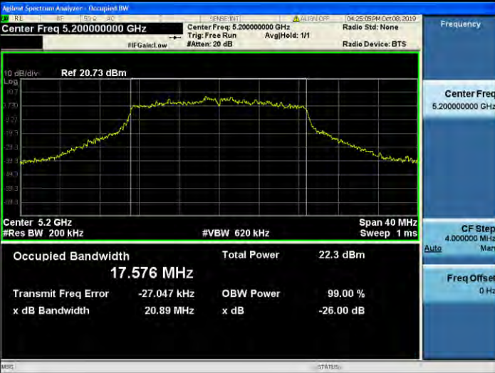
802.11ac_VHT20 UNII 2C BAND 26dB Bandwidth(CH 120)
