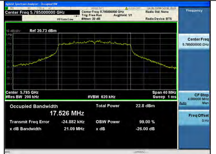
802.11ac_VHT20 UNII 3 BAND 26dB Bandwidth(CH 157)
