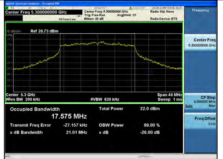
802.11ac_VHT20 UNII 3 BAND 26dB Bandwidth(CH 157)
