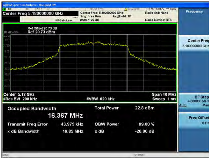
802.11a UNII 2C BAND 26dB Bandwidth (CH 100)
