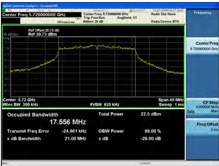
802.11n_HT20 UNII 2C BAND 26dB Bandwidth(CH 144)
