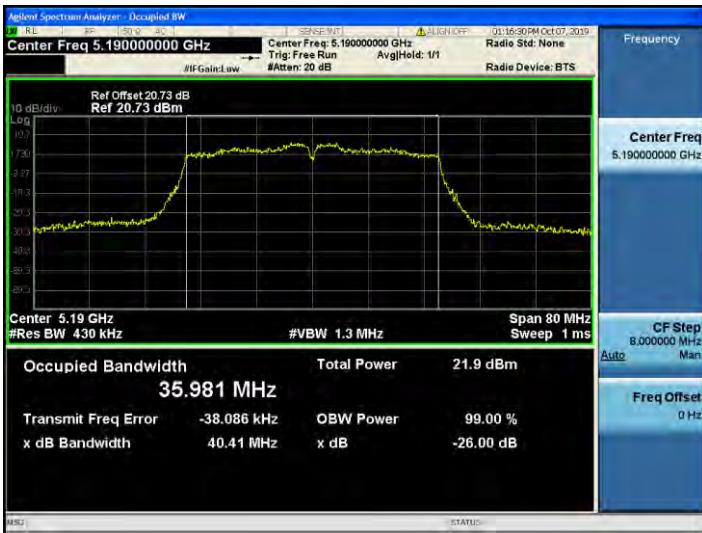
802.11ac_VHT40 UNII 2C BAND 26dB Bandwidth(CH 142)
