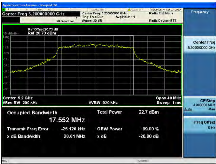
802.11ac_VHT20 UNII 2C BAND 26dB Bandwidth(CH 144)
