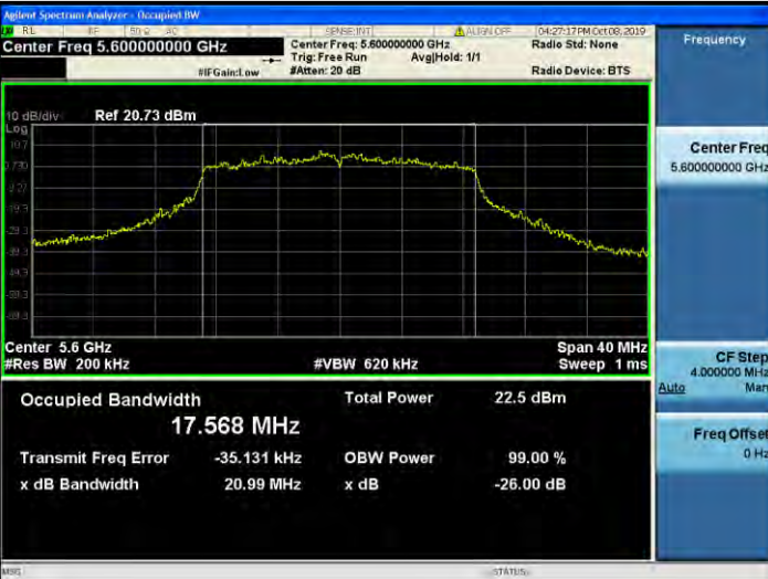
802.11ac_VHT20 UNII 2C BAND 26dB Bandwidth(CH 120)
