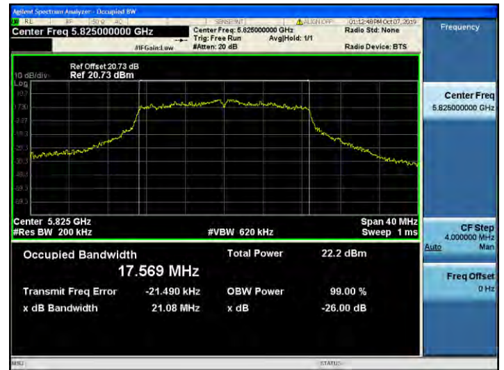
802.11ac_VHT20 UNII 3 BAND 26dB Bandwidth(CH 165)
