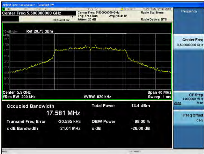
802.11n_HT20 UNII 2C BAND 26dB Bandwidth(CH 100)
