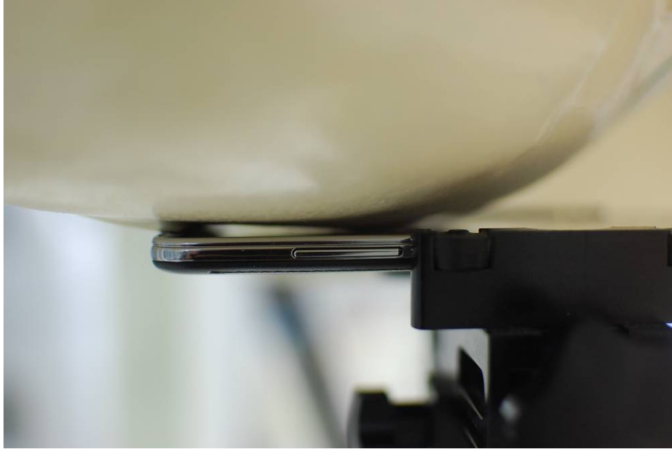
SAR Test Setup Photo 1 – Right Cheek
