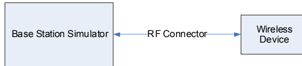
Figure 9-2 Power Measurement Setup
