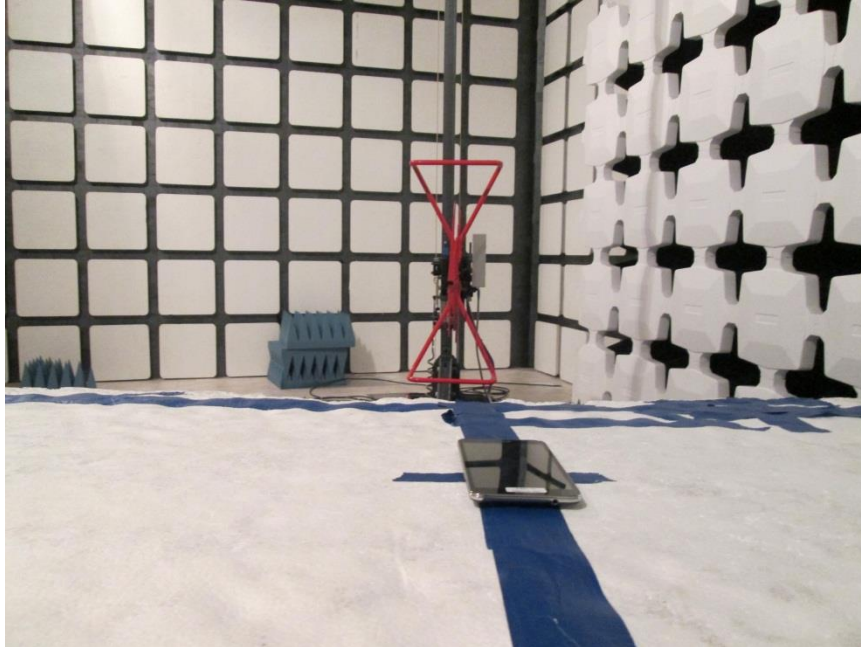
RADIATED FRONT PHOTO (BELOW 1 GHz)
