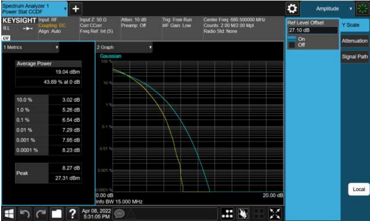
Sub6 n71. PAR Plot (15 M BW_Ch.349000_256QAM_Full RB)
