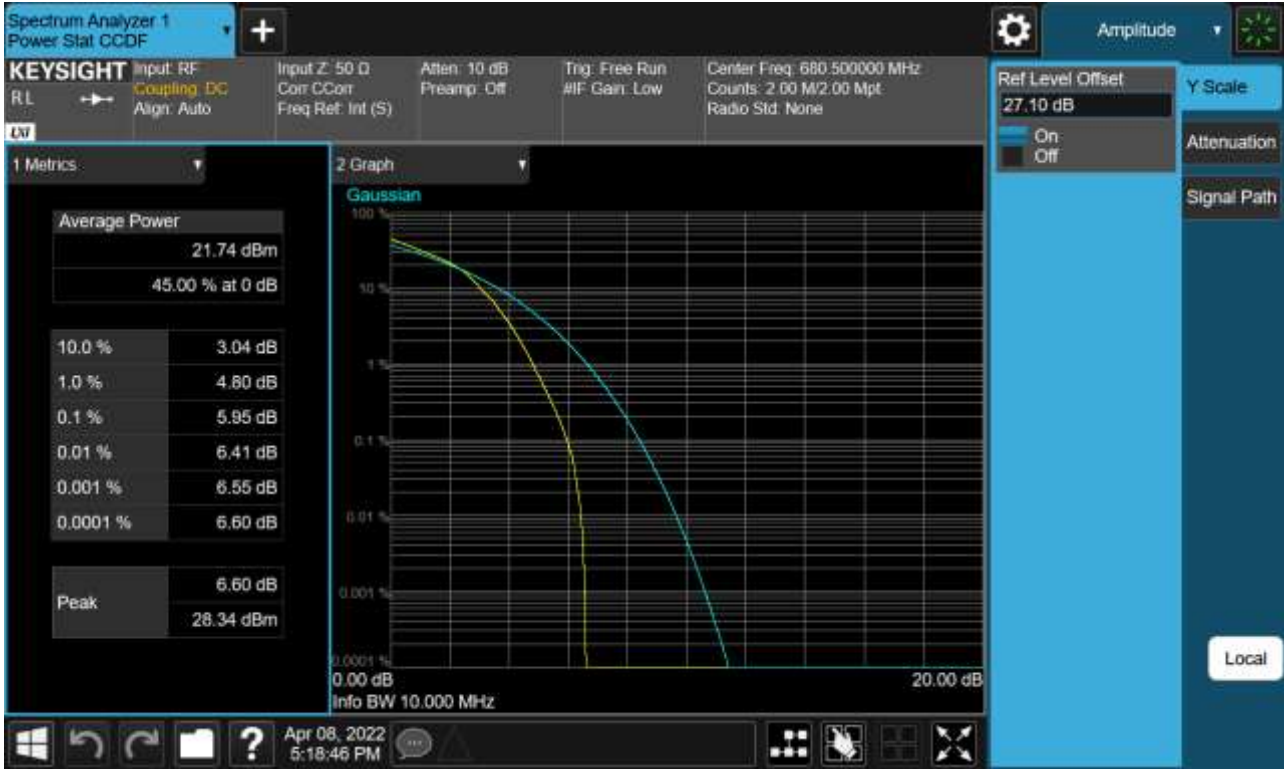
Sub6 n71. PAR Plot (10 M BW_Ch.349000_16QAM_Full RB)
