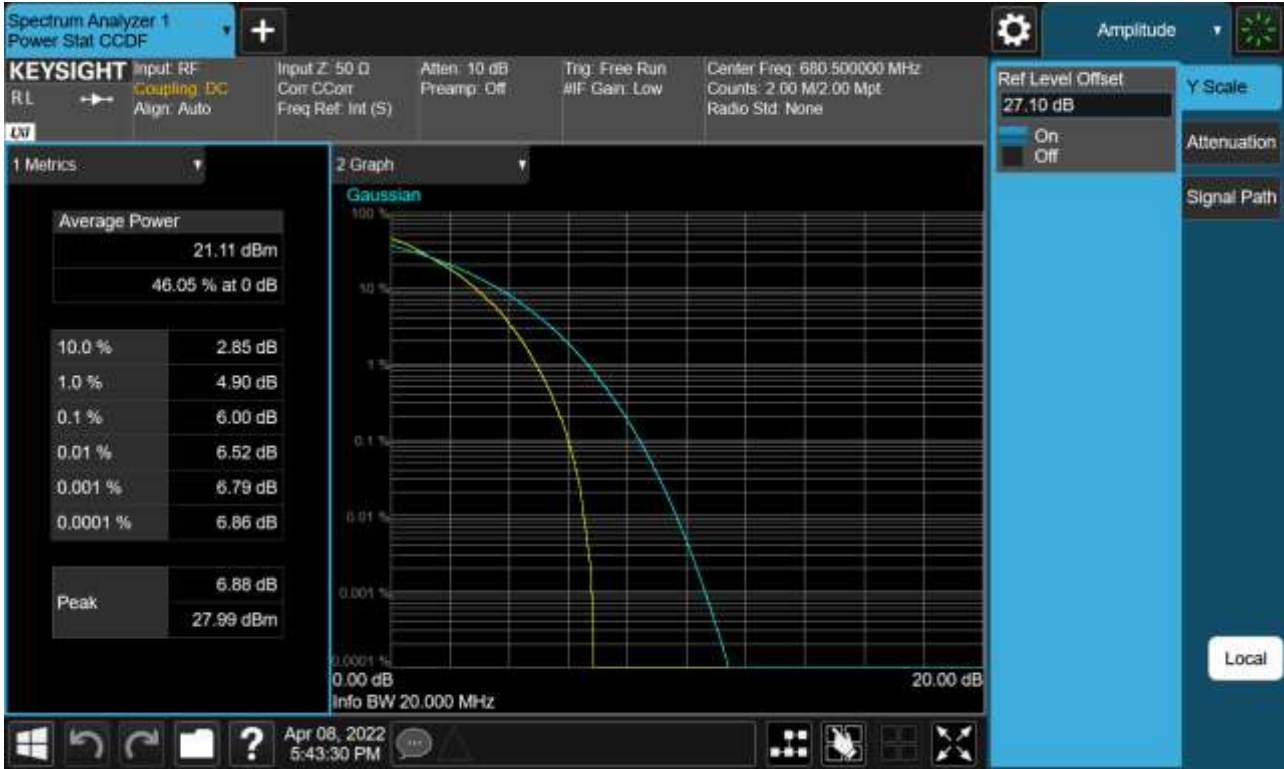
Sub6 n71. PAR Plot (20 M BW_Ch.349000_64QAM_Full RB)
