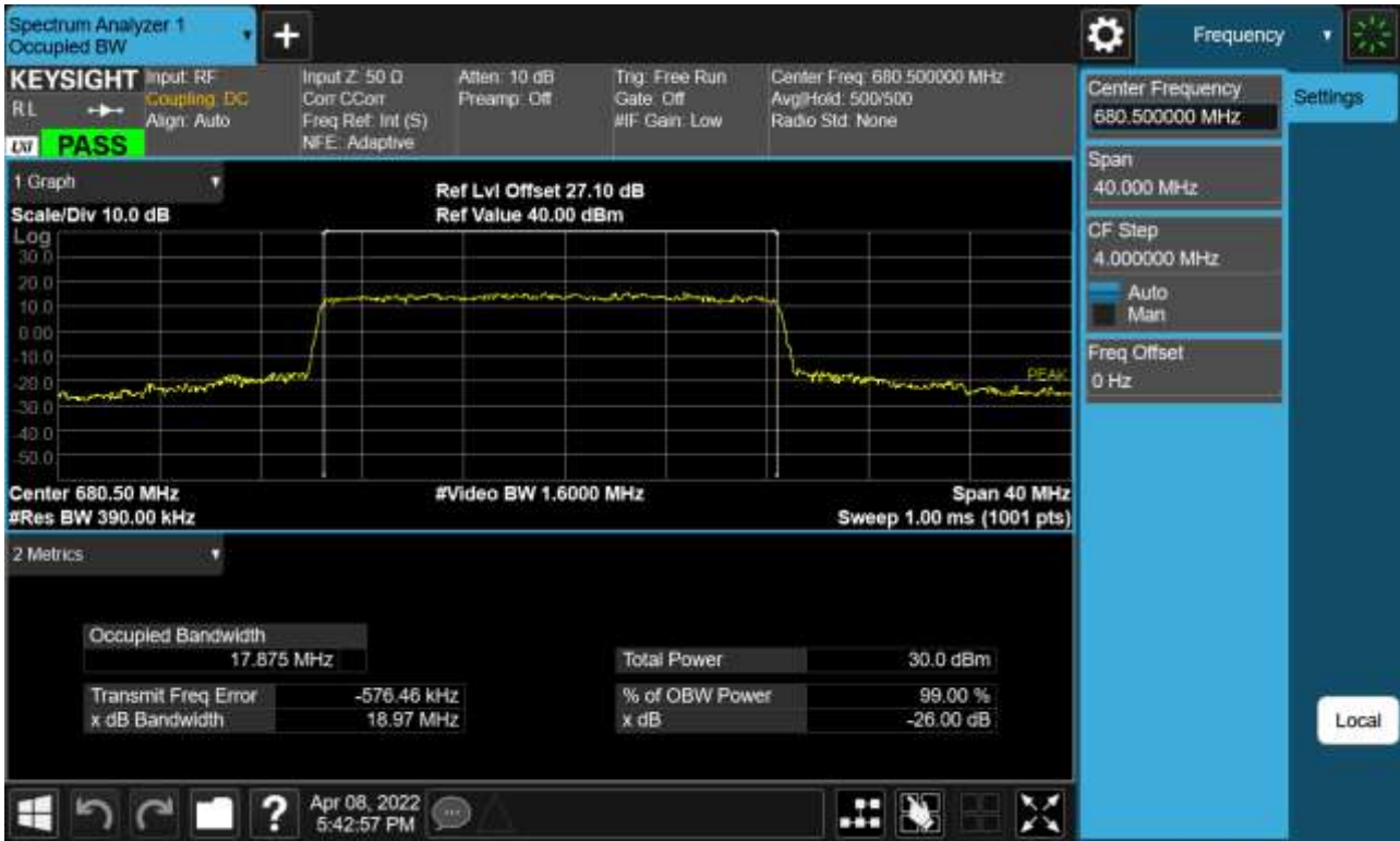
Sub6 n71. Occupied Bandwidth Plot (20 M BW Ch.136100 16QAM_ Full RB)
