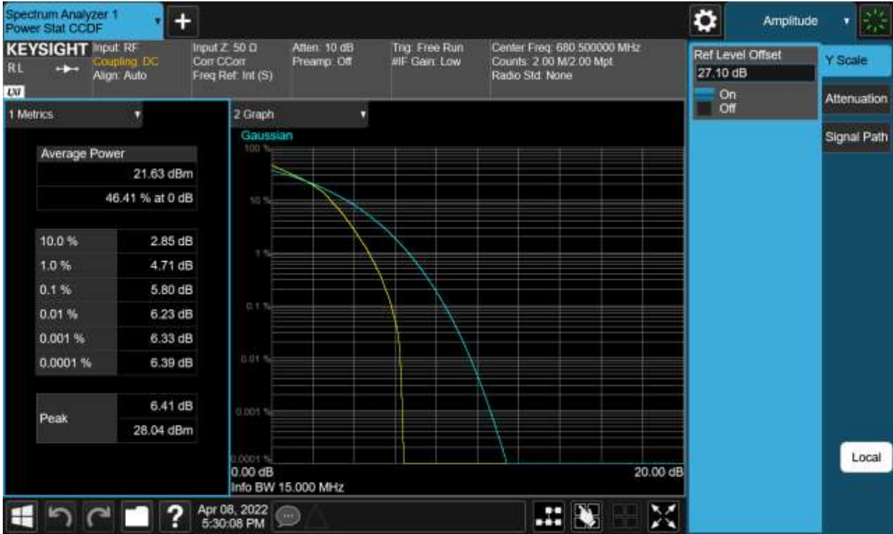
Sub6 n71. PAR Plot (15 M BW_Ch.349000_16QAM_Full RB)
