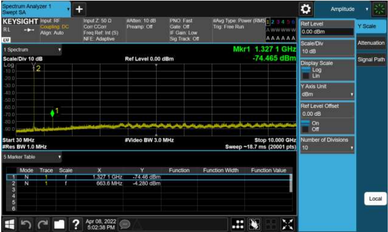
Sub6 n71. Conducted Spurious Plot _ (133100ch_5 MHz_BPSK_RB 1_1)
