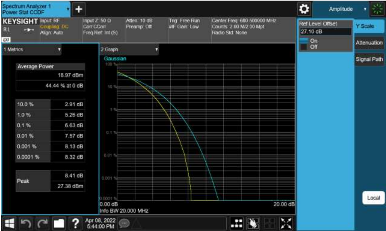
Sub6 n71. PAR Plot (20 M BW_Ch.349000_256QAM_Full RB)
