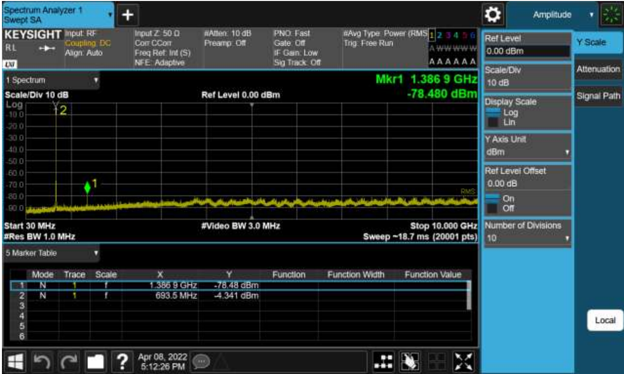
Sub6 n71. Conducted Spurious Plot _ (139100ch_5 MHz_BPSK_RB 1_1)
