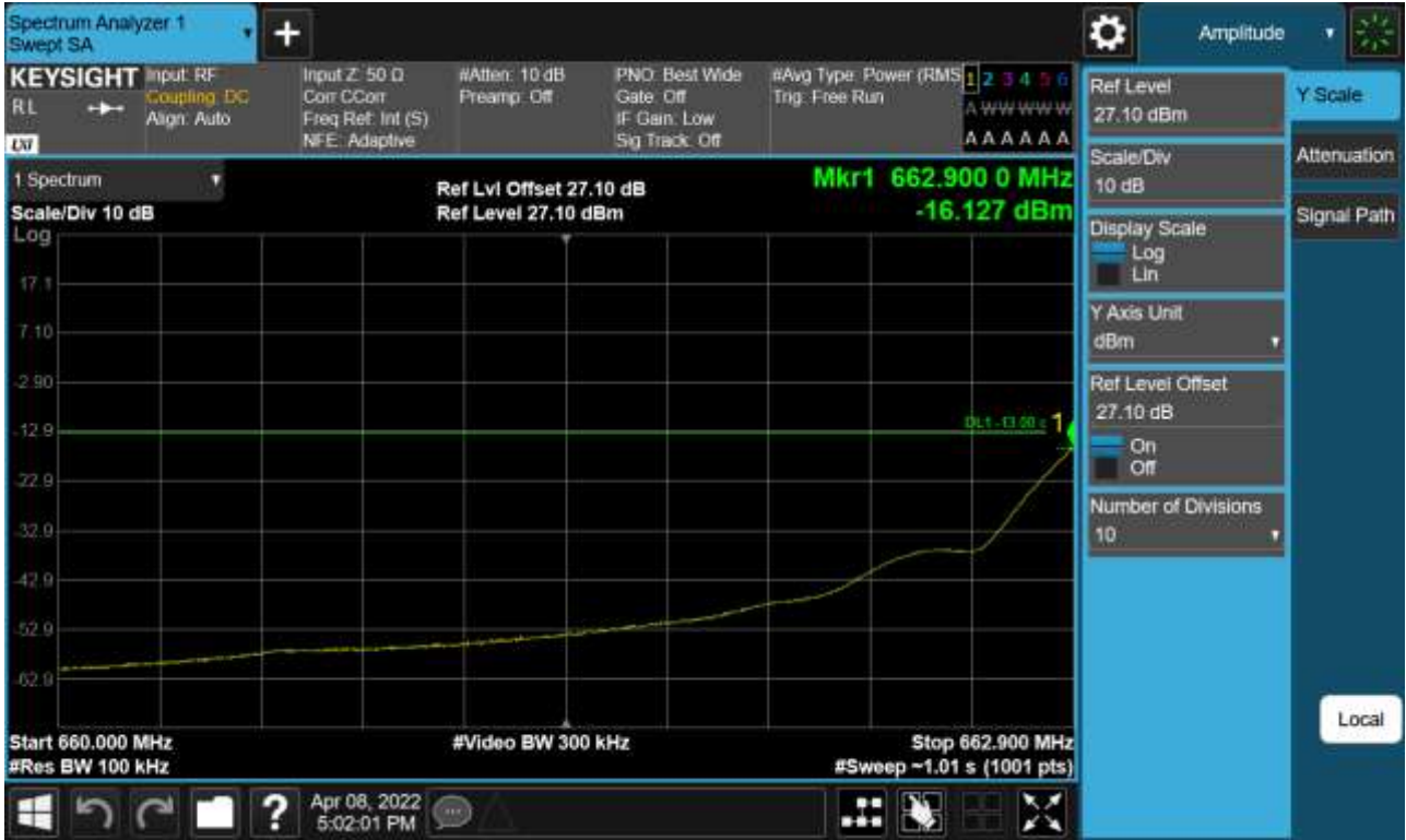
Sub6 n71. Lower Band Edge Plot (5 M BW Ch.133100 BPSK_RB1_Offset 0)_2
