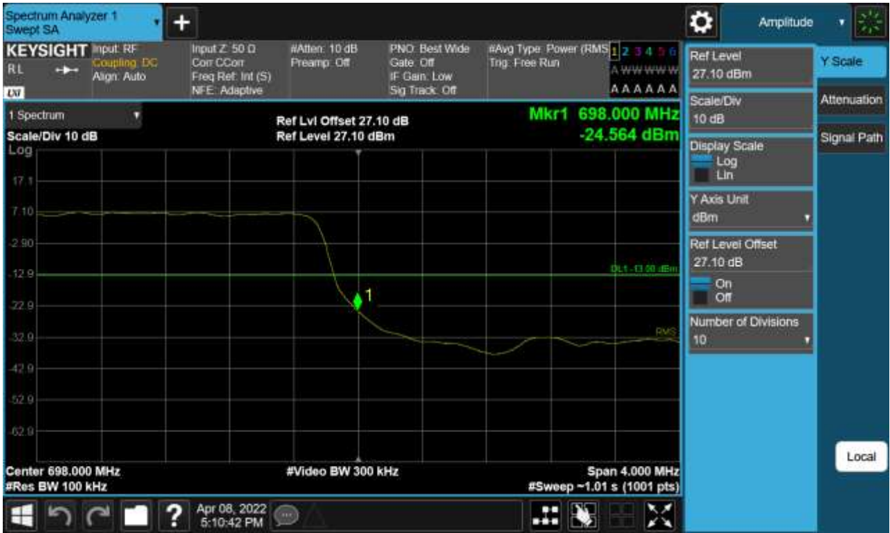
Sub6 n71. Upper Band Edge Plot (5 M BW Ch.139100 BPSK_ Full RB)
